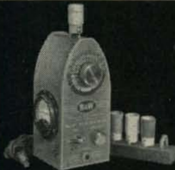
Grid Dip Meter
