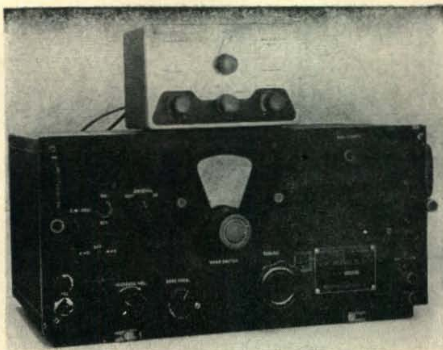
Fig 6—The Heath "Q" Multiplier used with a converted BC-348/0 aircraft receiver. The phone selectivity is 2400 cycles and the c-w selectivity is 750 cycles, 6 db down.
