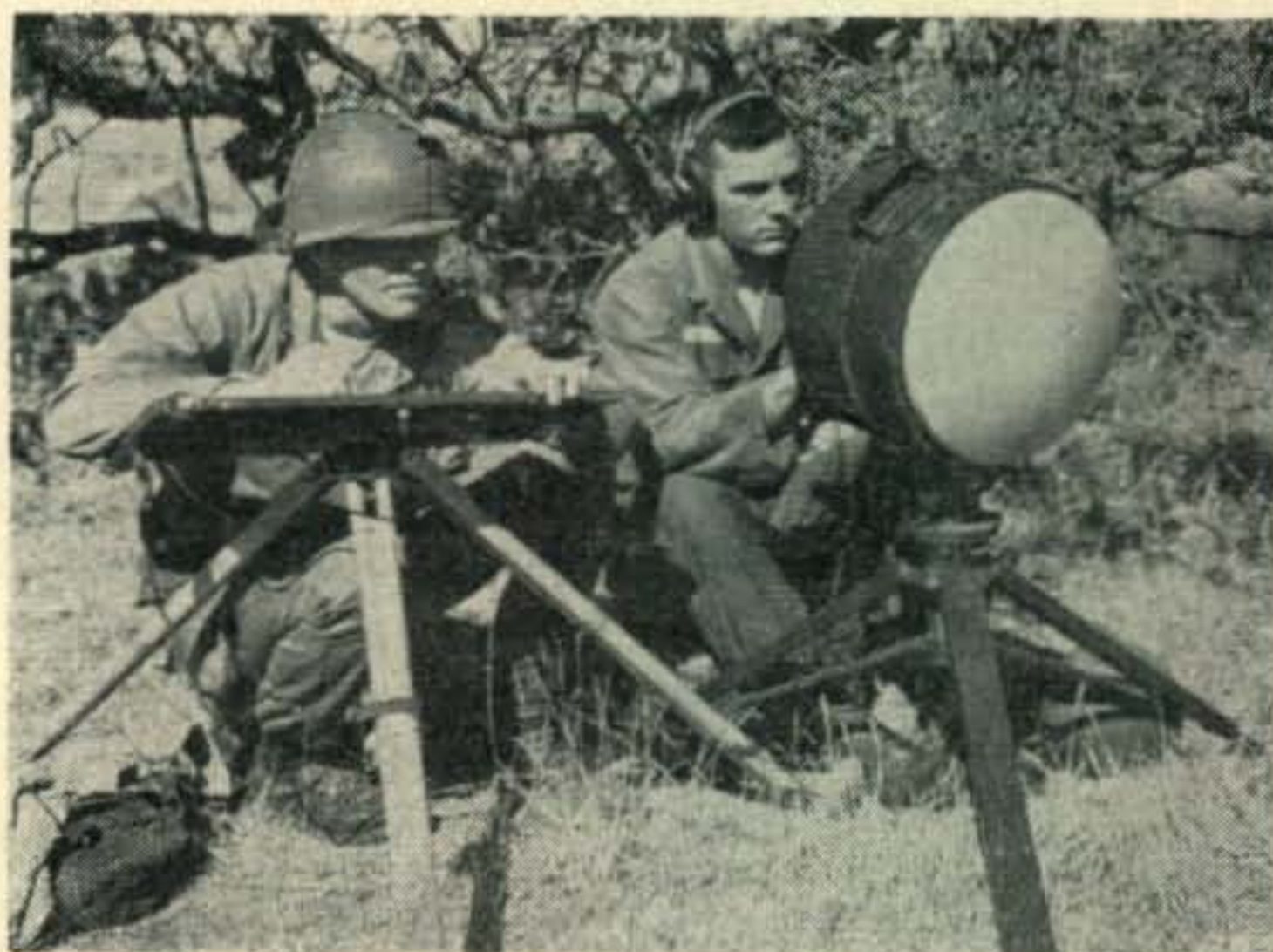
The new Army doppler radar system, the AN/PPS-4 in action. This unit has an effective range up to 3 miles in any weather.
