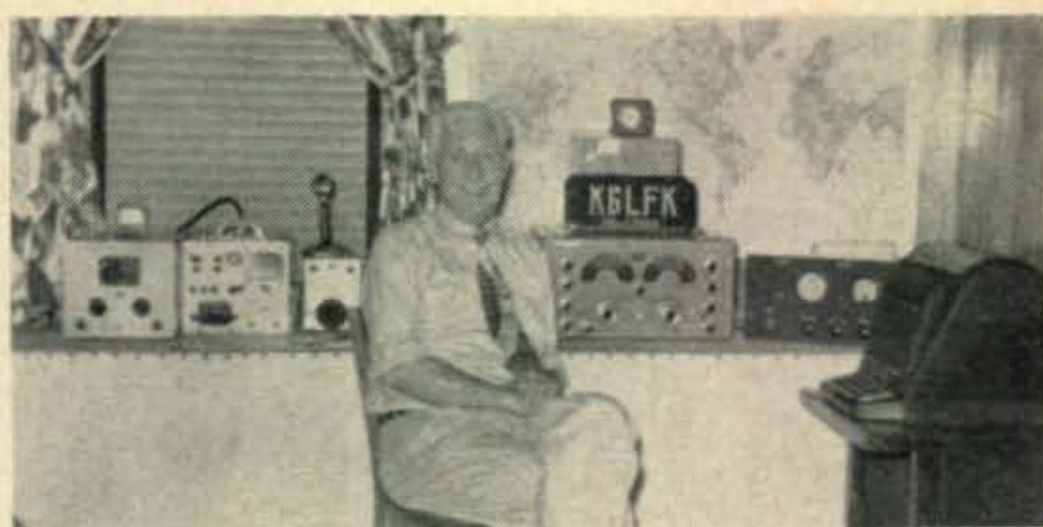
Mort Swingler, K6LFK, North Hollywood, California on 2, 6, and 40-meter RTTY. From right to left: Model 26, TU, NC-183, Mort, VFO, Communicator, and Linear Amplifier.
