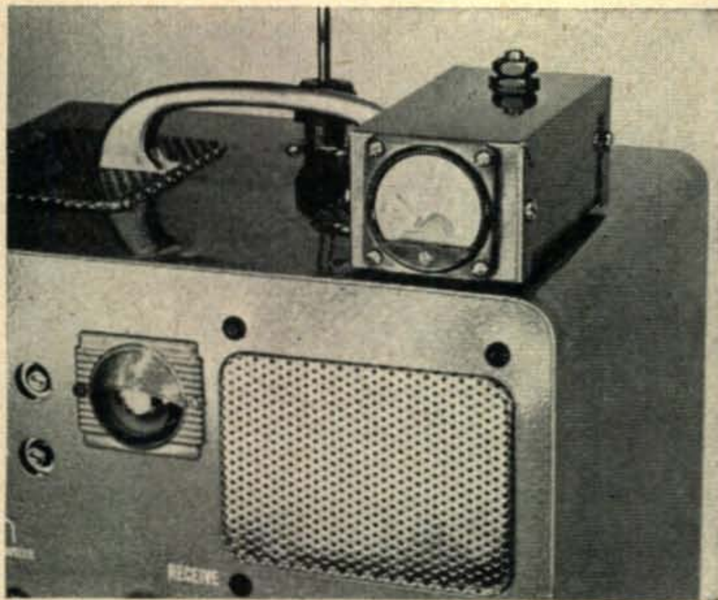
"Operator's eye view" of the plug in "S" meter as attached to a Gonset Communicator. The box is secured to the cabinet by a small screw through the ventilating grill.
