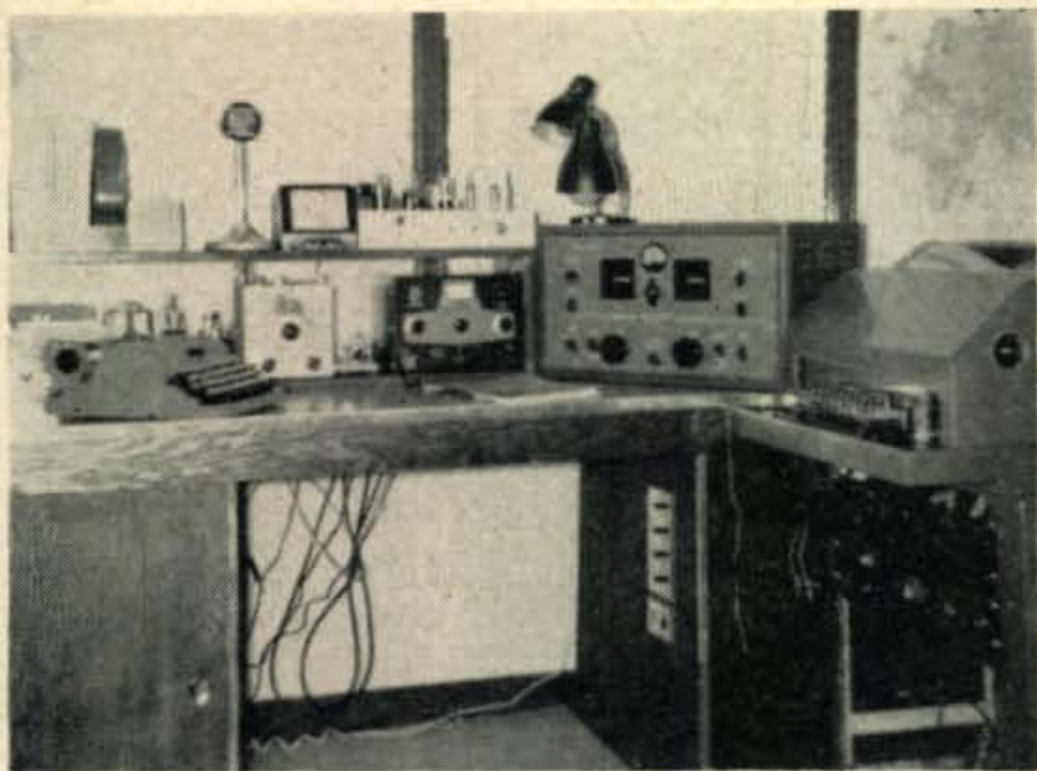
Charles Walker, K2IAZ, Union, New Jersey; on 80-meter RTTY. Equipment includes a Model 12, Heathkit VF-1, Viking Adventurer, and a 1/2-wave doublet antenna.
