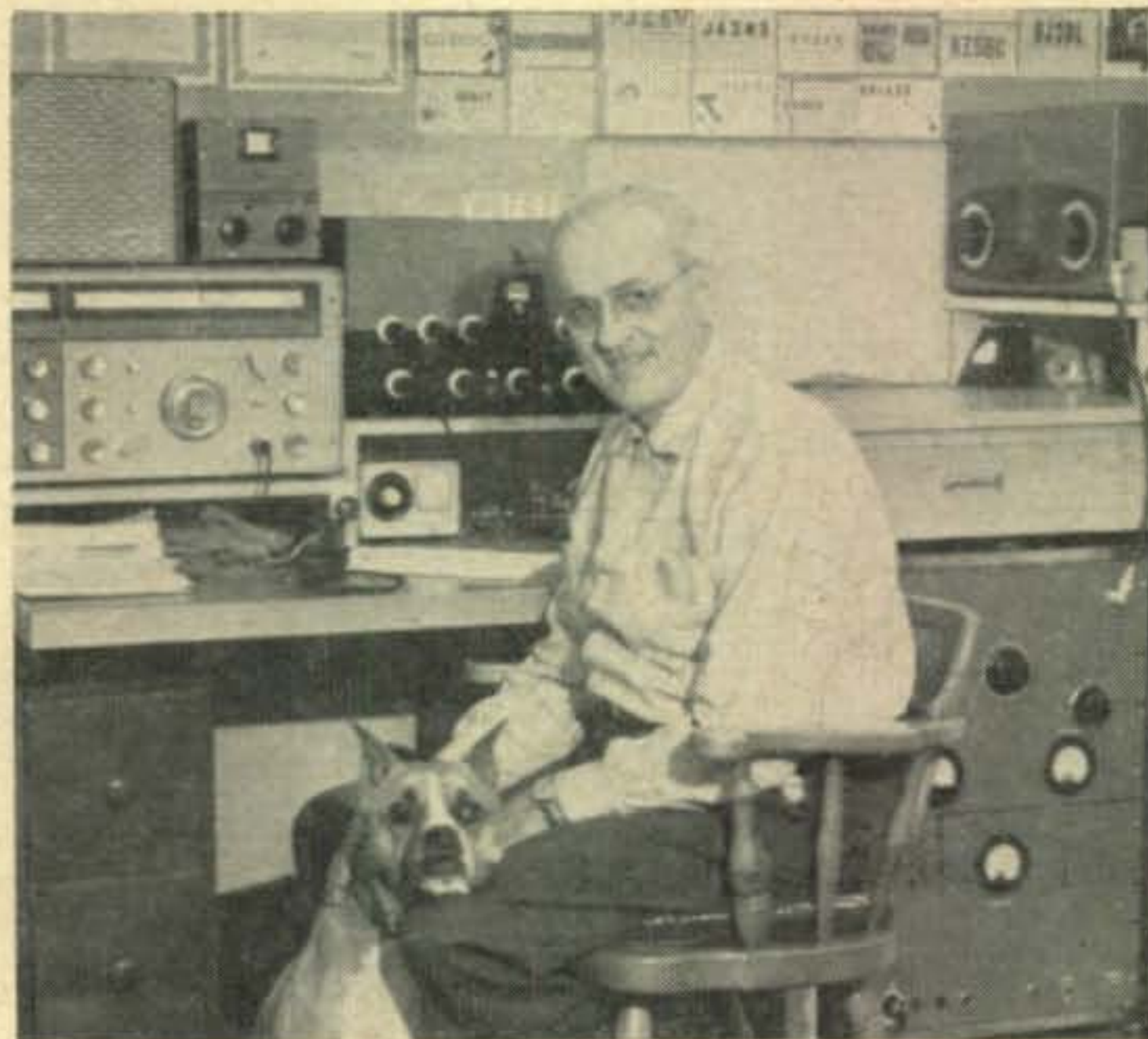
Neat set-up of W8FGZ, Earl Ensign, Bowling Green, Ohio runs a 304TH in a grounded grid final.
