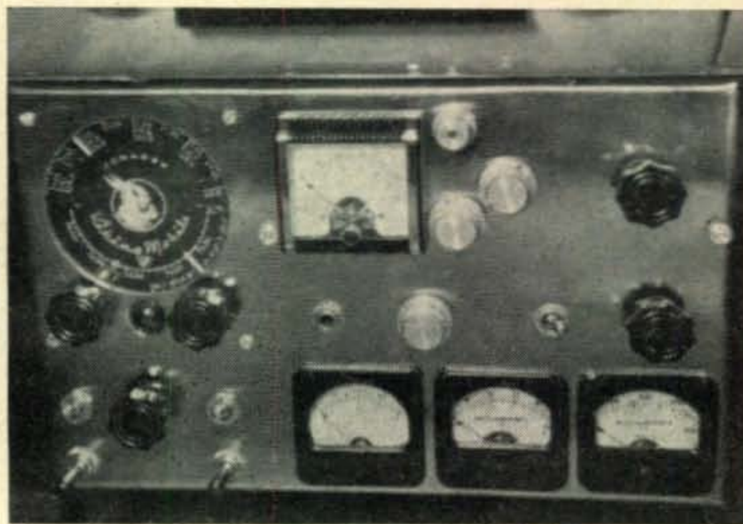
Fig 8. Close-up of the dash-mounted exciter unit which includes remote controls and metering for the final.
