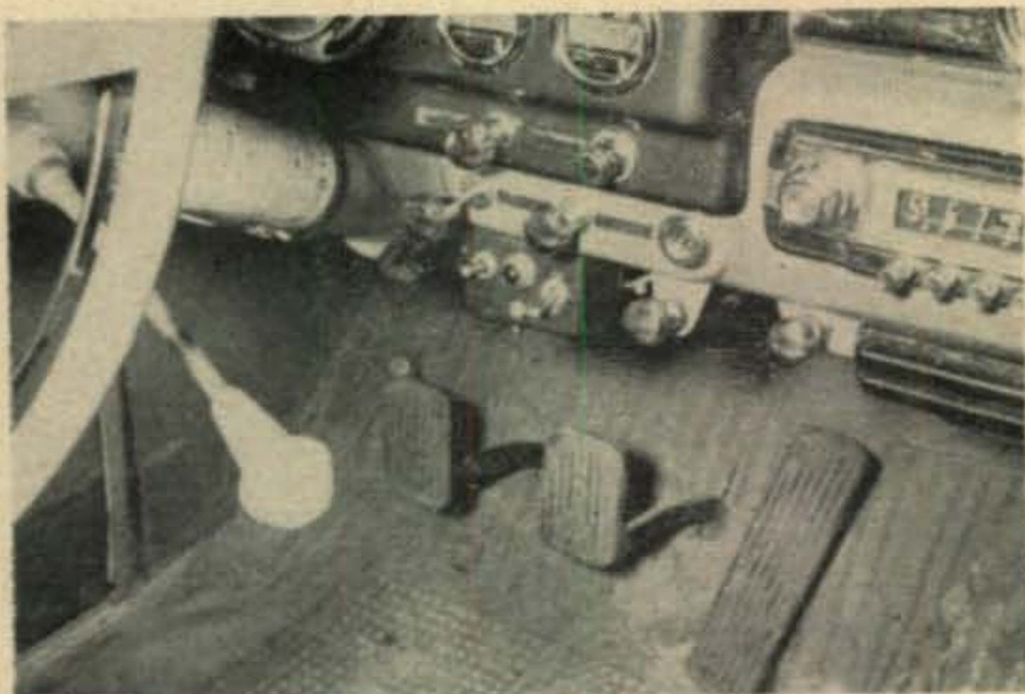
Only dashboard evidence of a mobile in the W60WP-W65XG family car is the small control box containing indicator light, tuning and transmit switches. The main on-off switch is located on the under side, out of sight and a guard against unauthorized turning on of the mobile equipment. Reception is via a crystal-controlled broadband converter.
