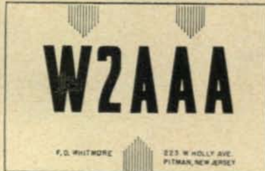
Fig. 9 (a) Slugs inserted by printer in form to print narrow lines creating design in bare card areas. (b) Example of printer's border styles used for separation and "boxing".
