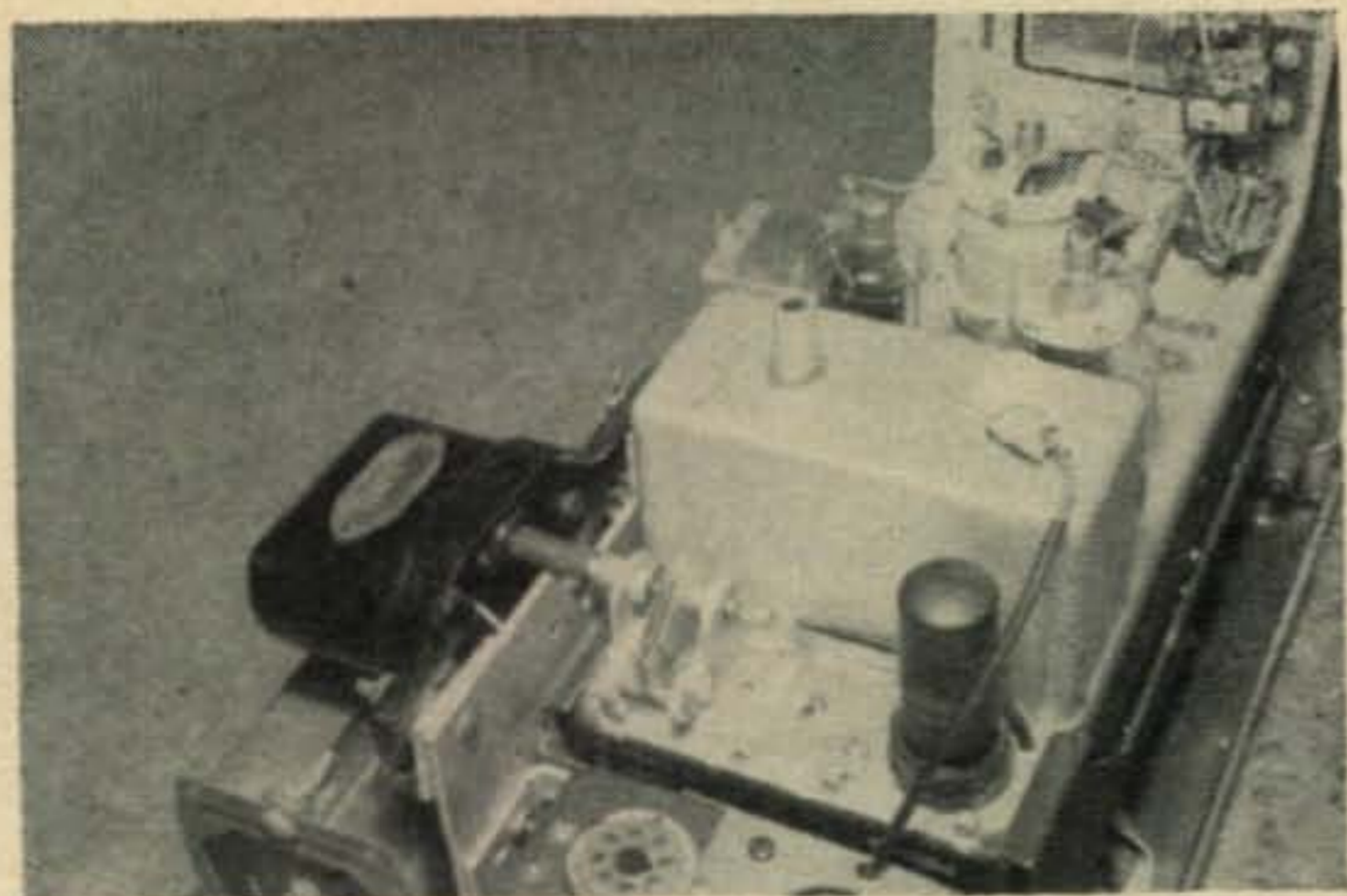
Mechanical aspects of the remote VFO control are shown in this close-up view. Old timers may recognize the electric windshield wiper motor, a once-common item on Model A Fords. The slug-adjustment between the condenser and oscillator tube is for the plate coil added in the transmitter modification process outlined in the text.
