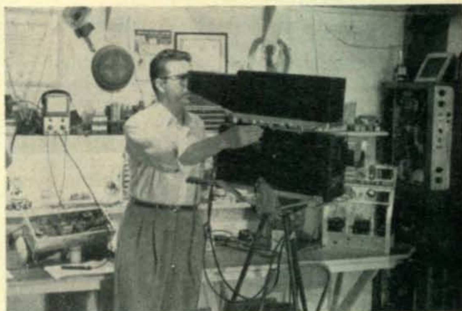
The ATJ camera converted by Carl Alsheimer. Note the beautiful focus, pan and tilt adjustments, also the viewfinder monitor (atop the camera).
