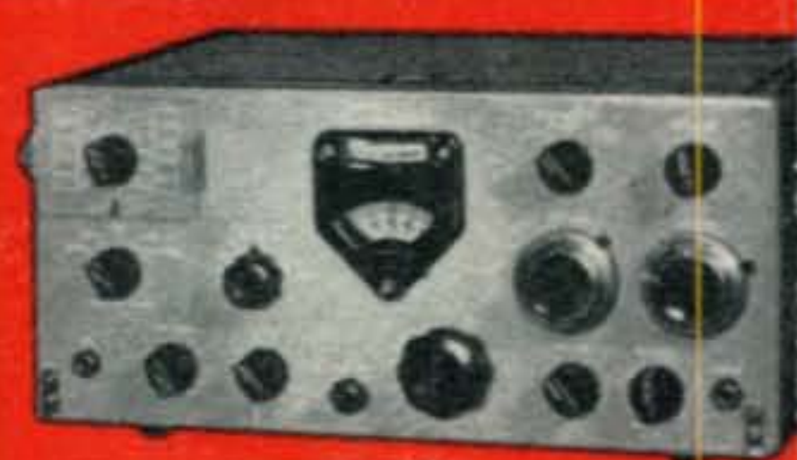
Collins KWM-1 Transceiver uses two RCA-6146's
