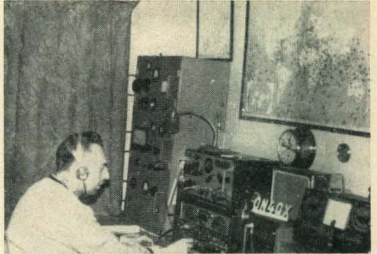
ON4QX, Bob Berge, Anvers, Belgium, runs 150 watts to an 814. Antenna is a 14 mc ground-plane. Receiver is an SX-100. Bob has 165 countries to his credit and regrets that he cannot visit San Marino this year, as planned, due to pressure of work.
