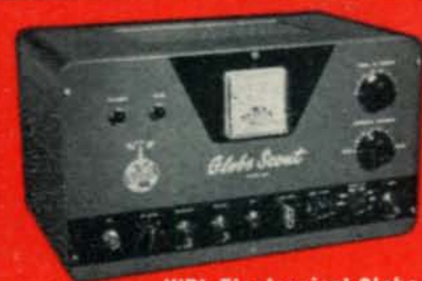
WRL Electronics' Globe Scout uses one RCA-6146
