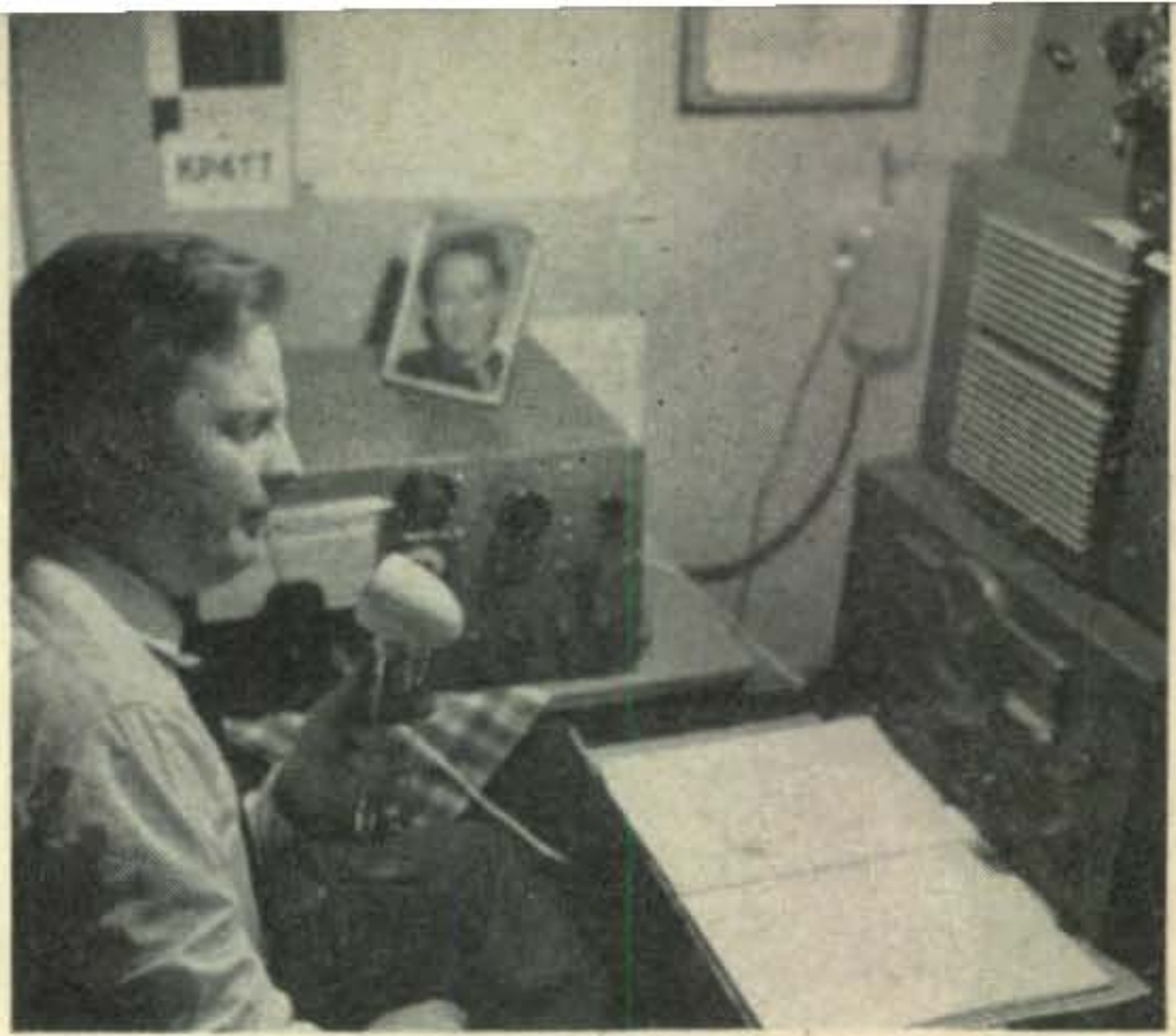
SM5BFR, Charlie Svard, Katrineholm, Sweden, runs parallel 807s at 150 watts on A3 and 200 watts A1 plus Gtloso V8O. Rx is SX-23 with converter. Charlie has worked 122 countries and 40 zones.
