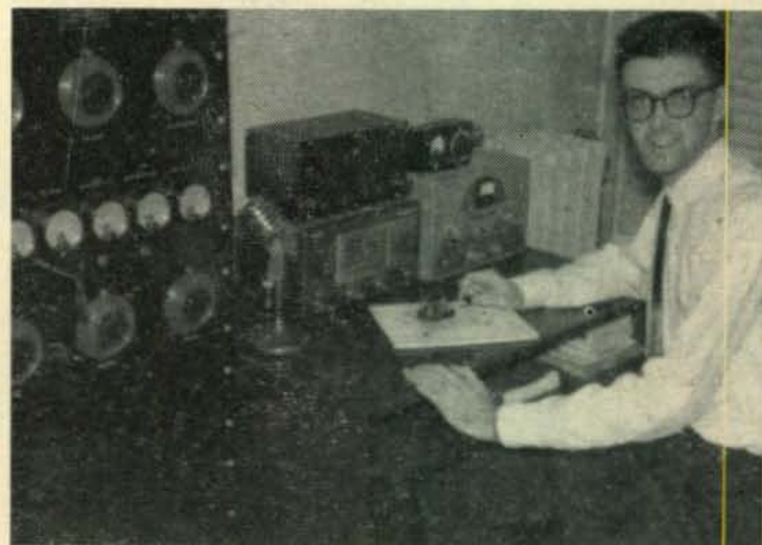
Don Wilbur, Jr., WN2MGW, 754 Myrtle Ave., Albany, New York likes to see pictures in the Novice column so he sent his in. His rig is an S-53A and a Heath DX-35. Don uses the famous T2FD antenna.
