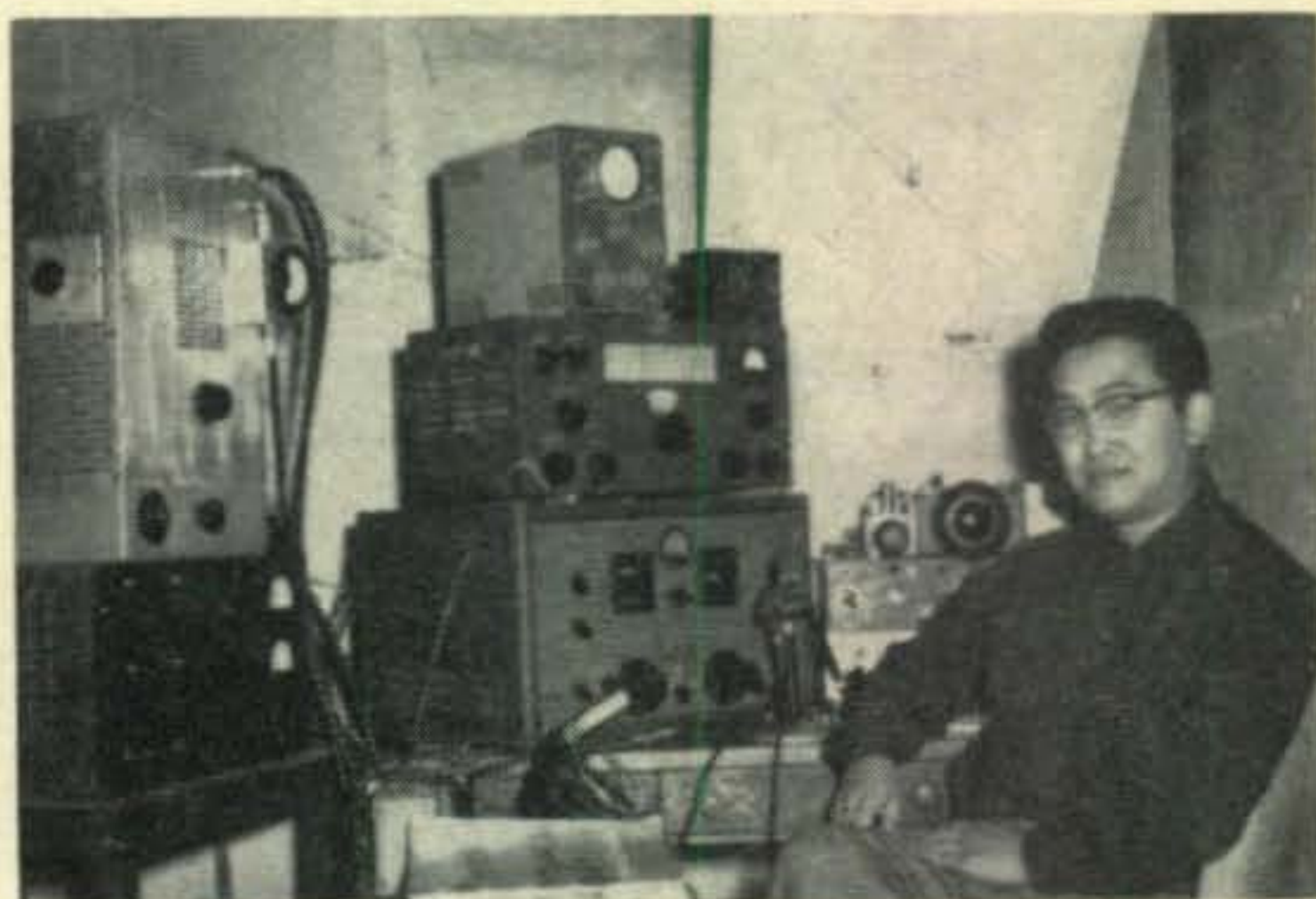
W7GXA, Joe Naemura, was first licensed in 1938. Present setup consists of a 6C21 (450TL) final to a three element telrex beam 85 feet up. Receivers are a SP40OX for phone work and a home brew job for DX. Joe has worked 240 countries and, in June, was due to add the letters "M.D." after his name. QTH is Portland, Oregon. (Photo courtesy Willamette Valley DX Bulletin)
