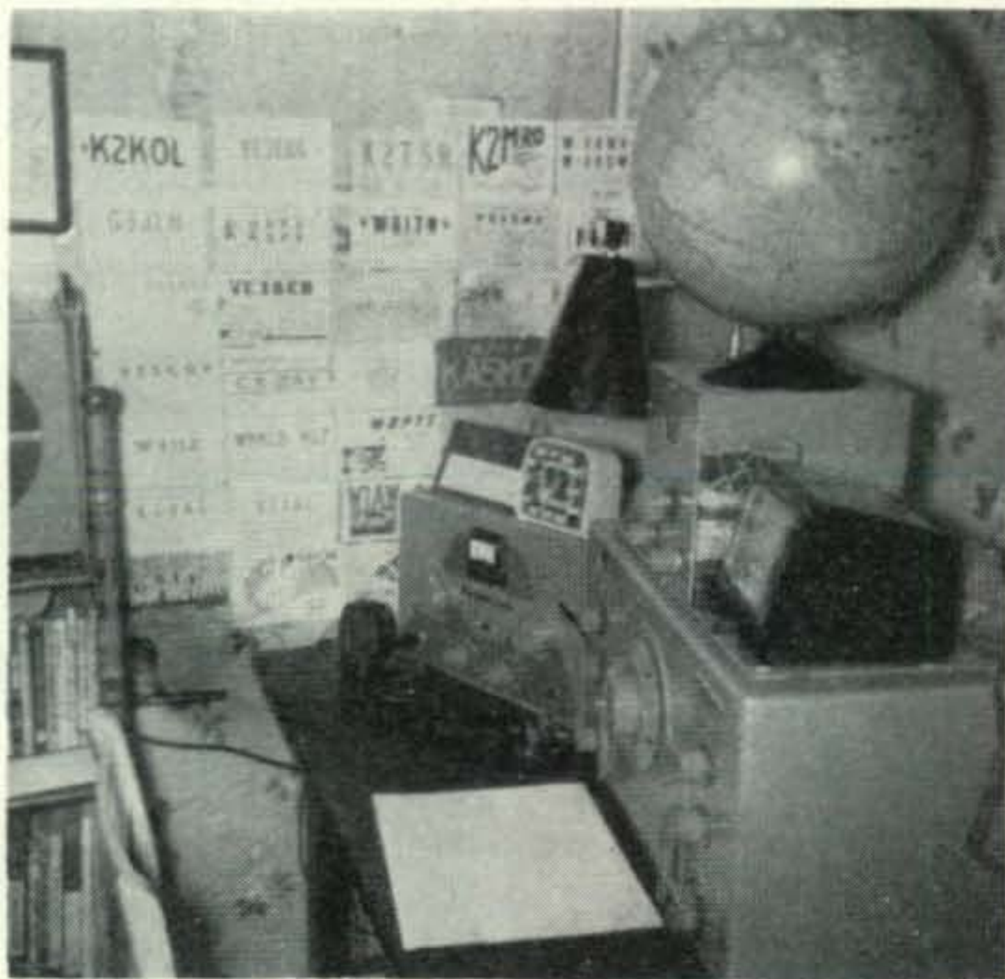
Boy, look at those DX cards on the wall of K2TLQ, Bruce D. Jenkins, shack, located on 3797 Redman Road, in Brockport, New York. Although Bruce is now a General, he still likes to work cw especially on 15 meters with his 40 meter dipole. Other antennas include an 80 meter dipole and a 10 meter rotary beam.
