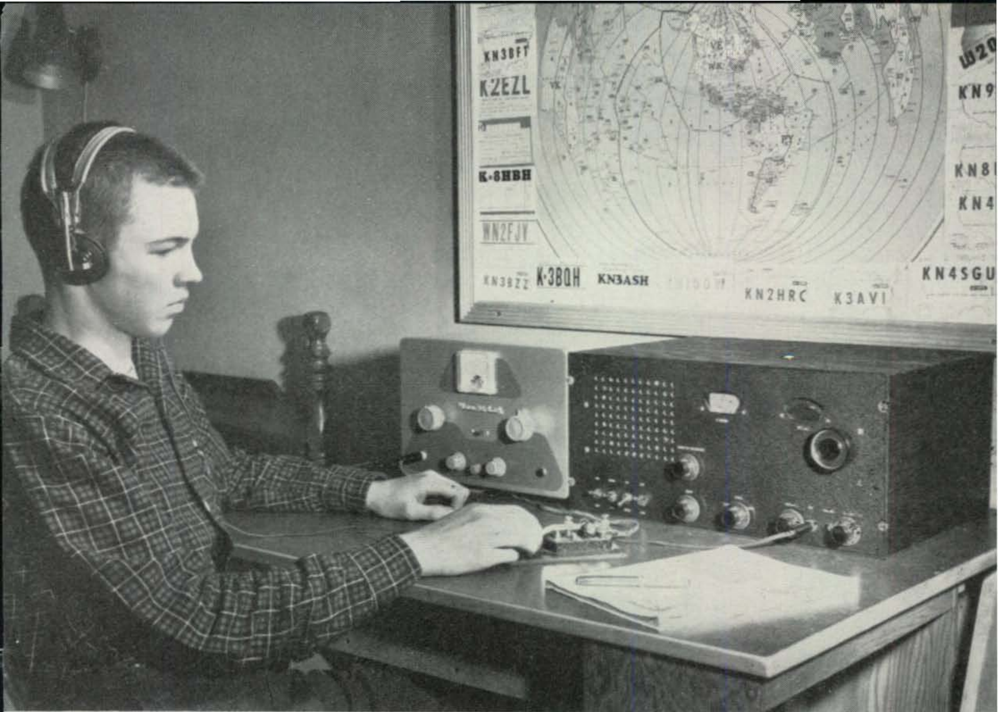
Dick, KN2DLX, 220 Taylor Avenue, Endicott, N. Y. made a beautiful communications receiver out of the war surplus BC-453 (The SSB Q5'er) as shown
