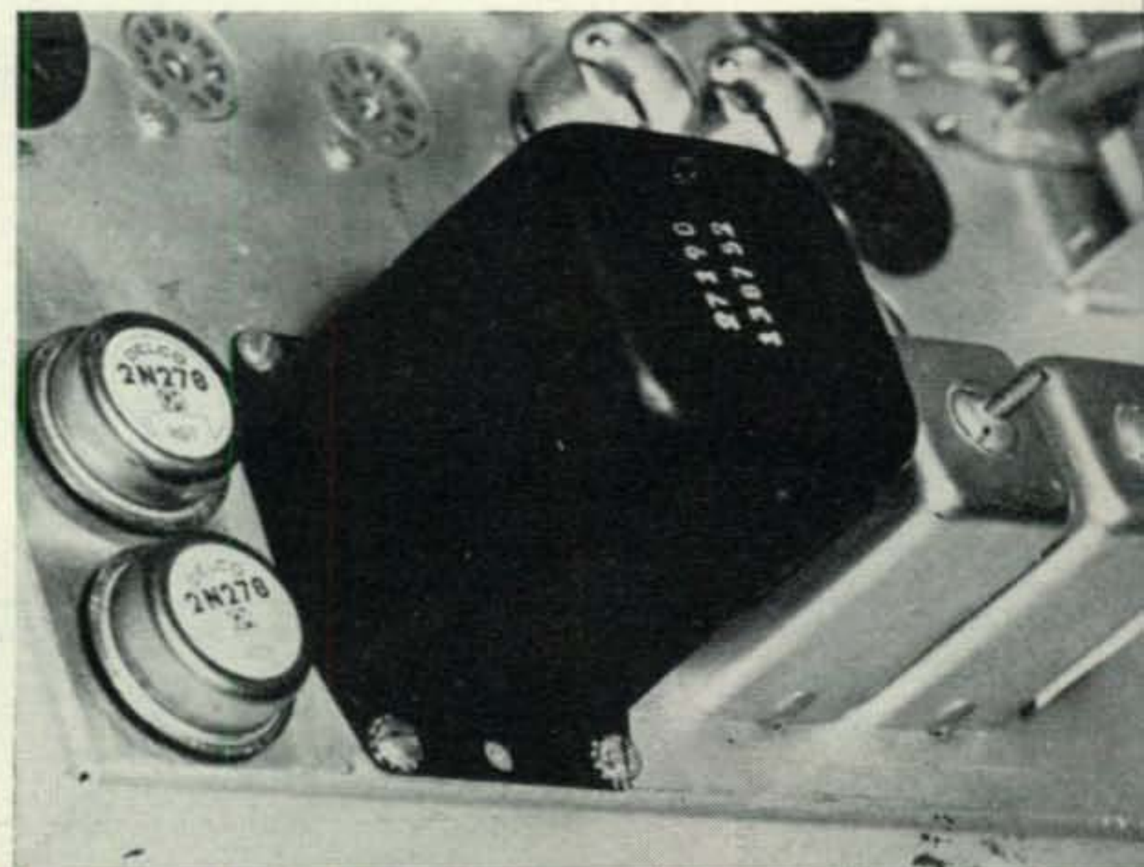
Transistorized power supply incorporating the Chicago DCT-2 transformer. The 2N278's are insulated from the chassis by mica washers.
