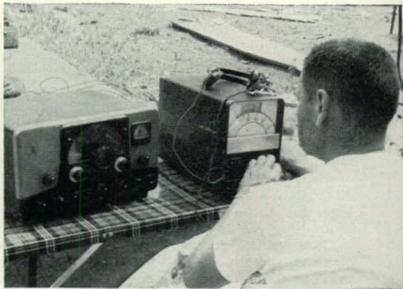
The Johnson Ranger was taken along as a spare transmitter and turned out to be real handy for ten meter CW and meter operation since we were short on the necessary crystals for the HT-32's.
