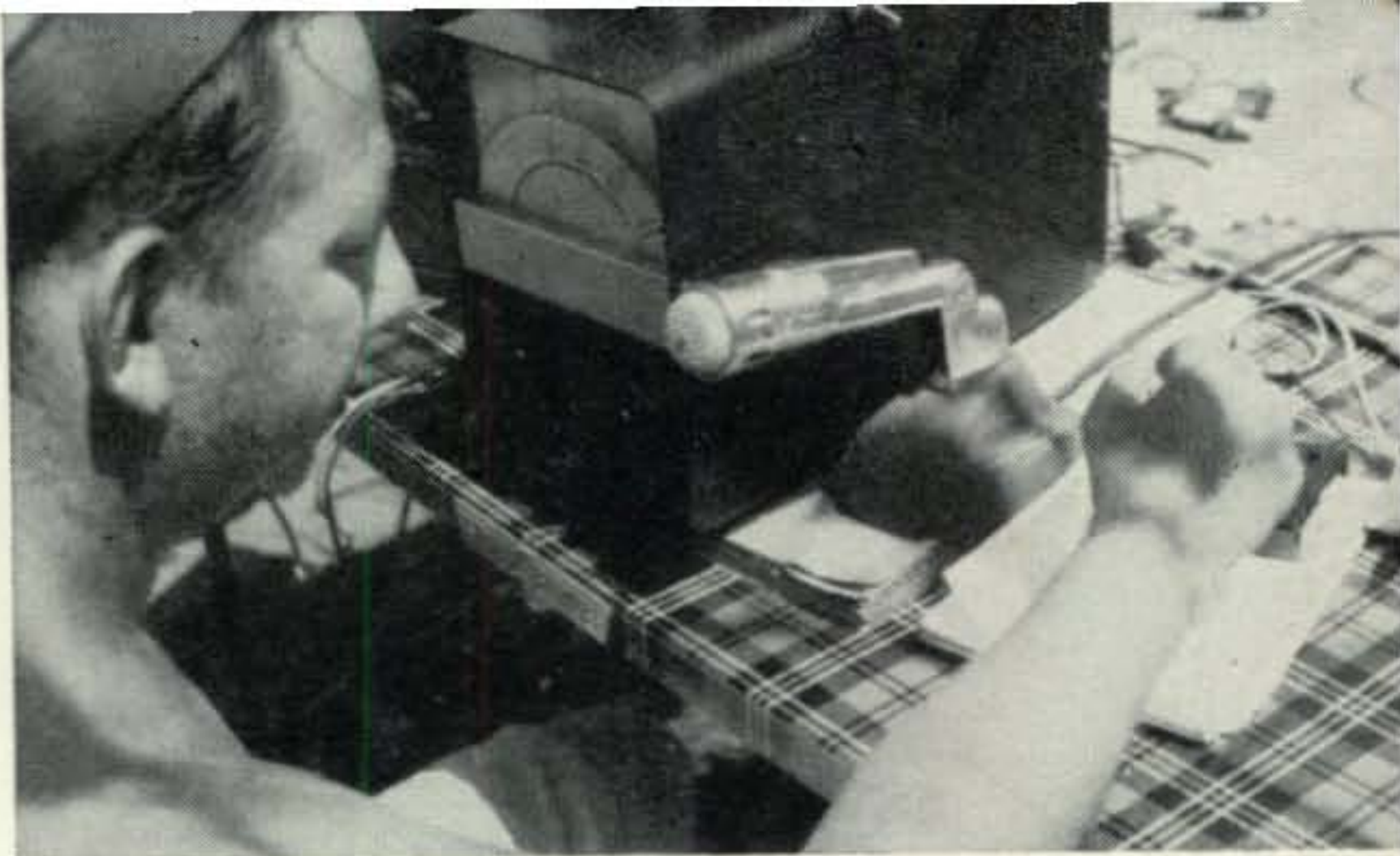
Frank, normally a straight CW man, gets in some phone operation using the Electro-Voice 664. This mike was chosen for the trip because it could withstand the heat and high salty humidity.
