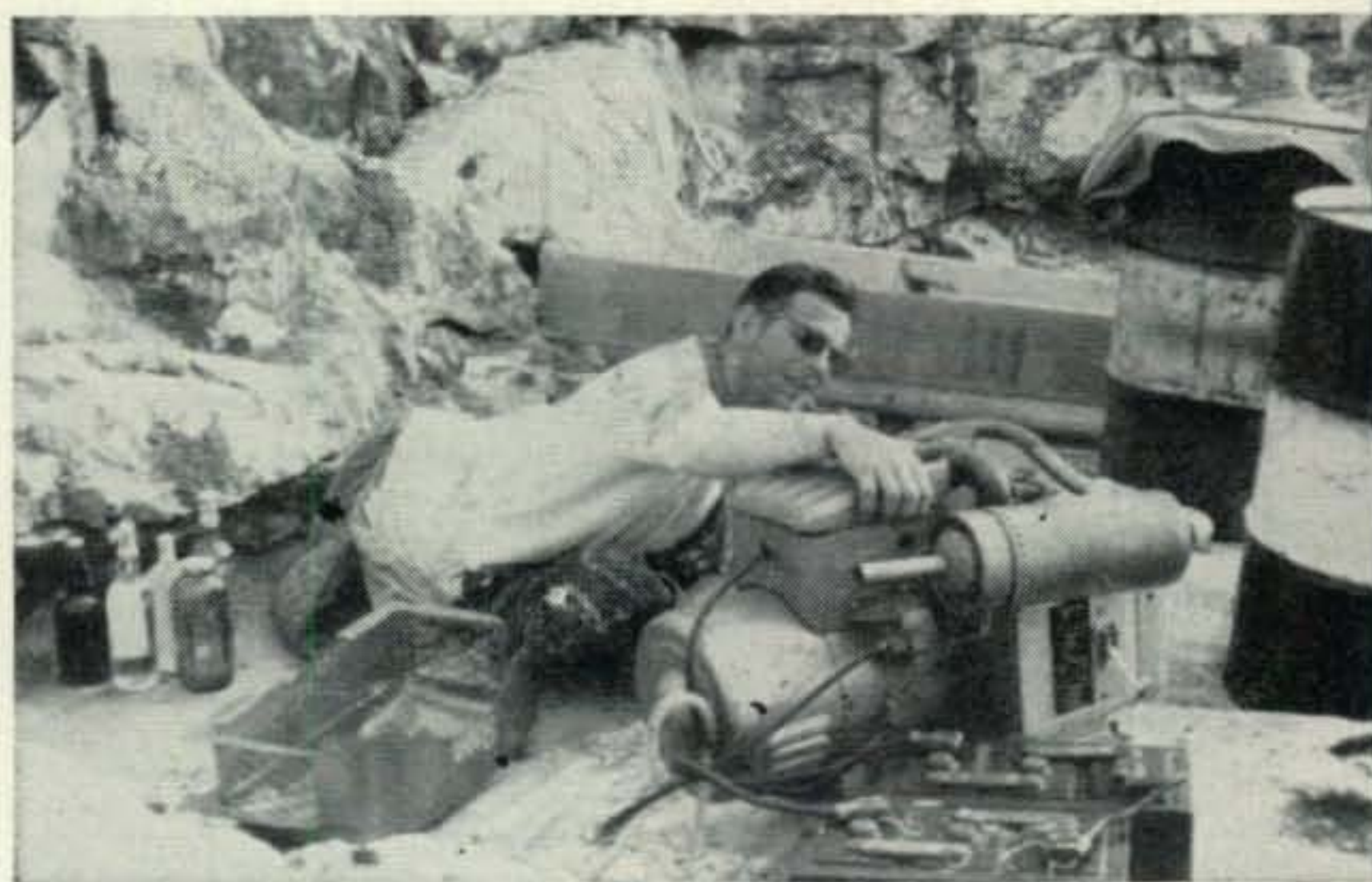
Dale servicing the Onan generator. The Onan gave us little trouble outside of its tremendous weight and the need for batteries to run it.
