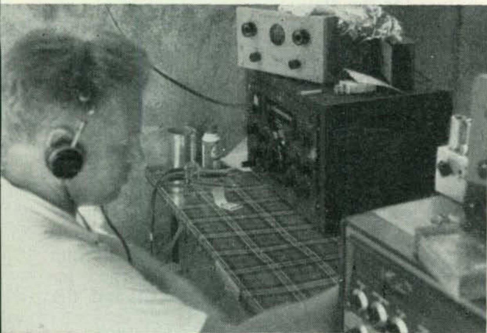
Don Chesser W4KVX operating station inside old cistern. Equipment is 75A3, HT-32, Harvey-Wells Z-Match used for loading long wire on 40 and 80.
