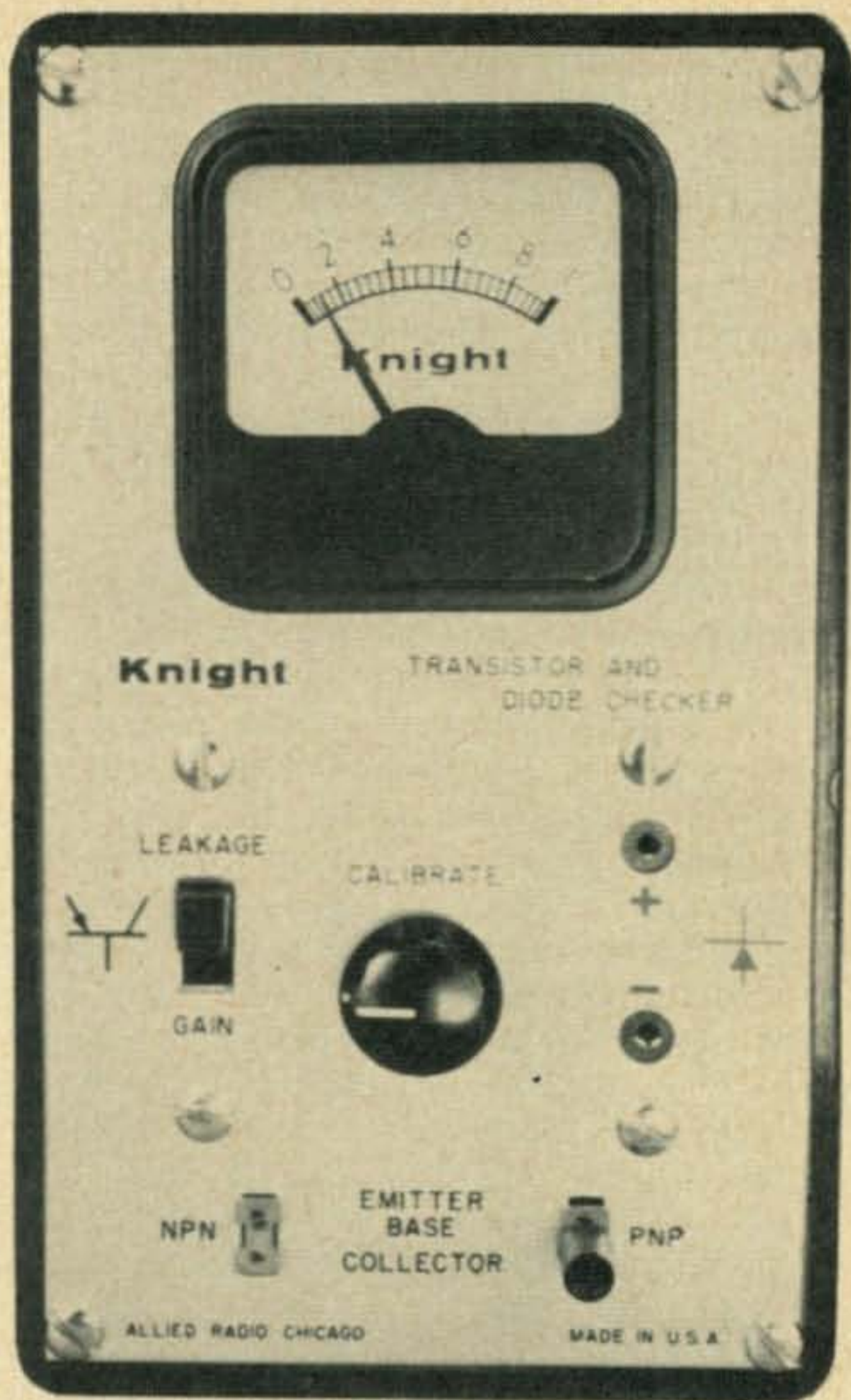
Tester set to show the leakage of a 2N109 transistor. The leakage/gain switch is spring loaded.
