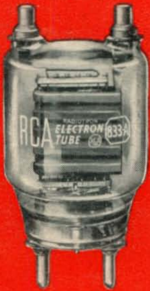
POWER TRIODE 1500 watts input CW; 1300 watts SSB; 1000 watts AM. Full input to 30 Mc.
