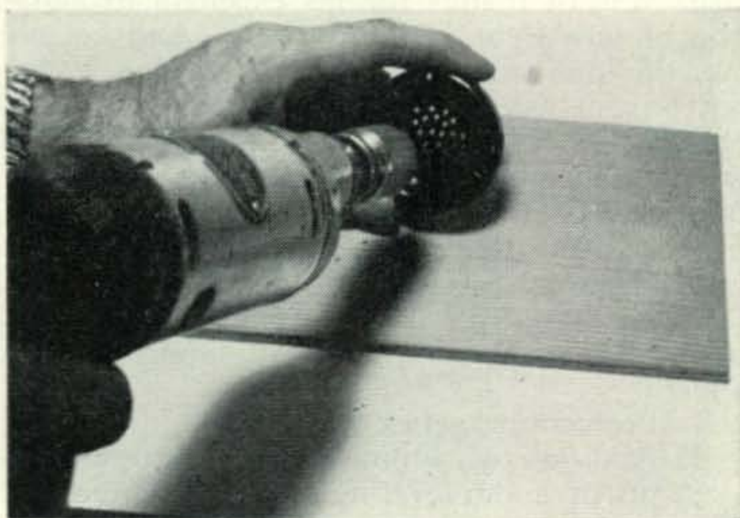
4—Microphone cover is drilled to increase pressure sensitivity.
