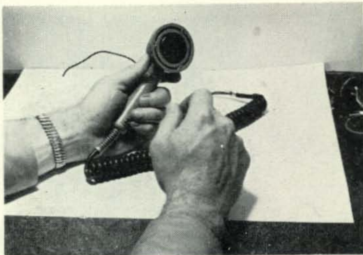
3—T-1 transmitting unit is mounted in microphone cup after two connecting wires from curl cord are carefully soldered to center button and outside ring. Minimum heat should be used for this soldering.
