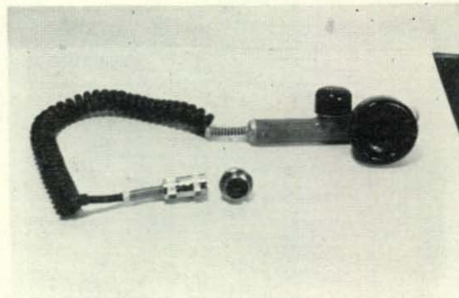
5—Microphone is reassembled and desired plug attached. Most T-17 microphones contain wire connection diagrams pasted inside of button switch.
