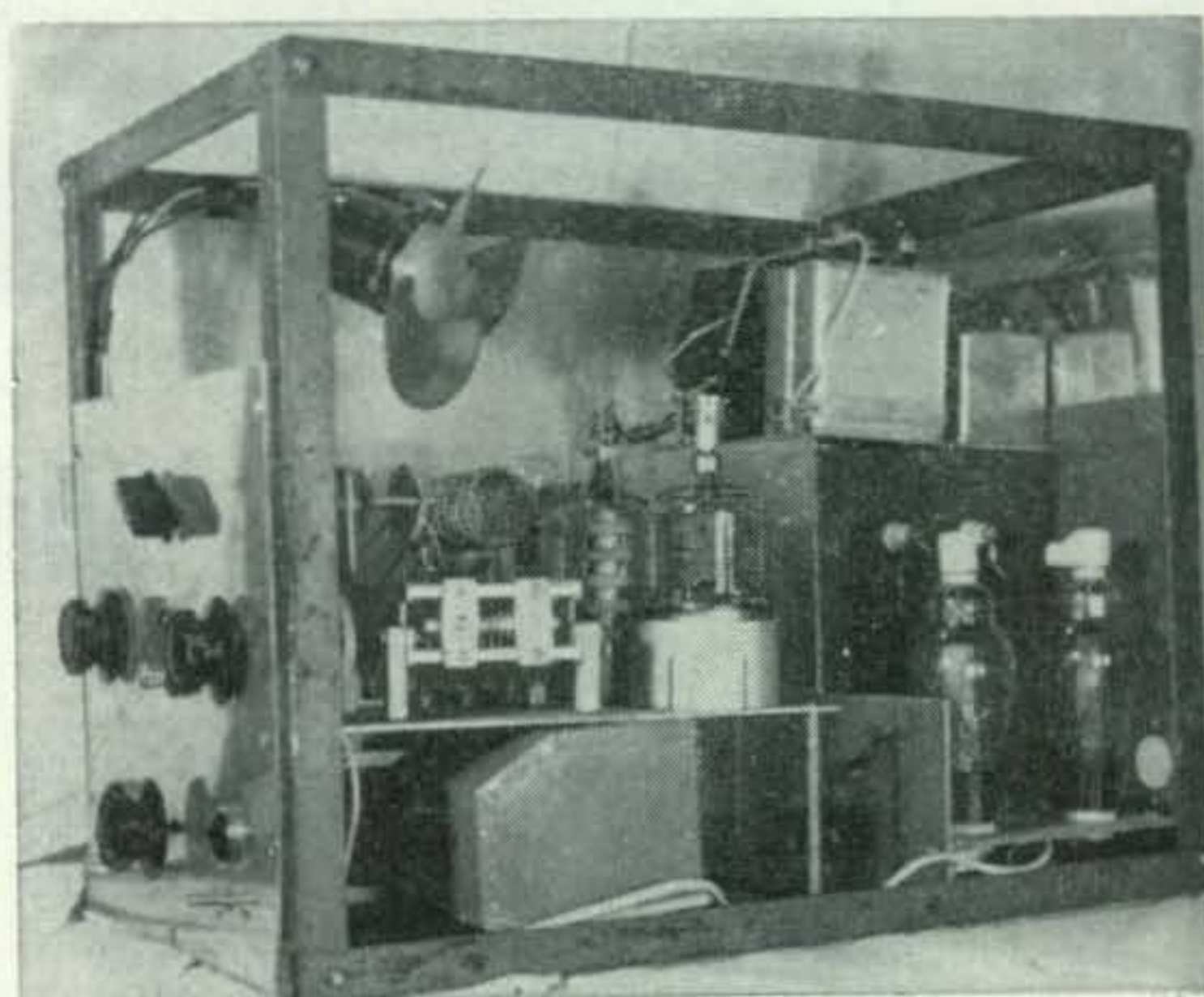
High-power amplifier in its chassis holding framework. Transformer at bottom lying on its side is a multi-filament type.
