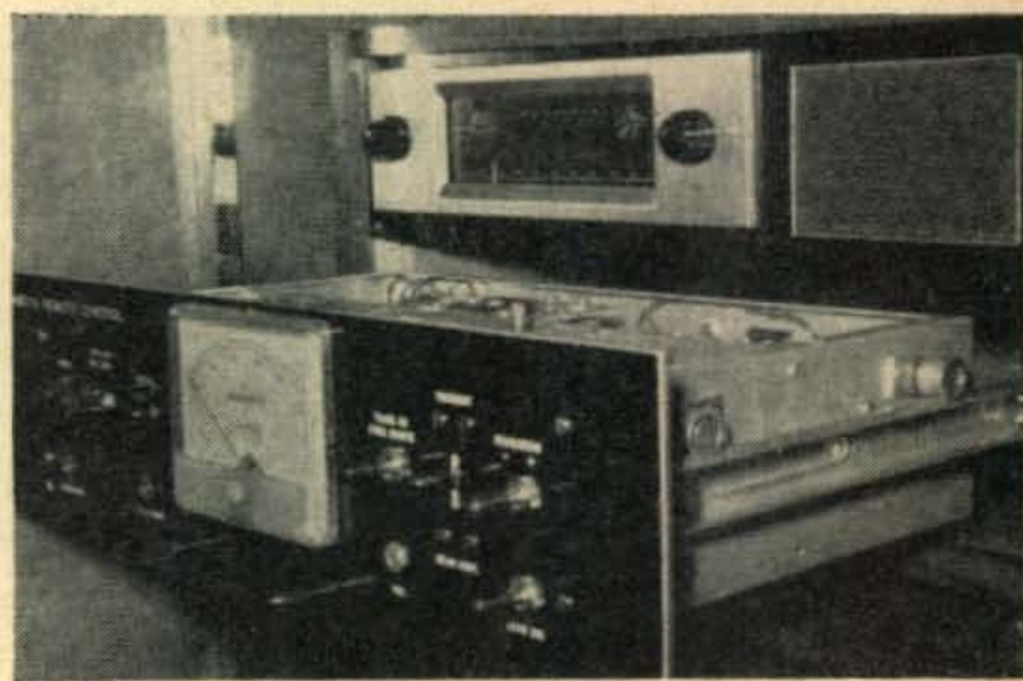
The remote control unit in its withdrawn position for adjustment. The unit will lift clear of the tracks for complete removal.
