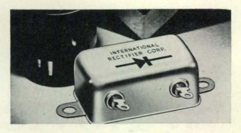
Although it looks like a "bath-tub" capacitor, it is actually the new International Rectifier high voltage silicon zener voltage regulator, and will replace the gas discharge OC3 shown in the picture.
