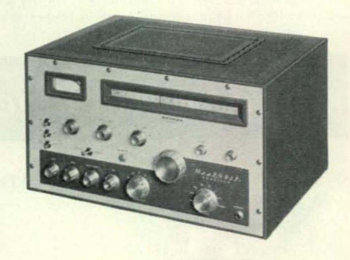
bridged T-notch filter is employed for maximum heterodyne rejection. Complete accuracy is obtained with the use of a built-in 100 kc crystal calibrator and the set features 10 db signal-to-noise ratio at less than 1 microvolt input. S-meter and many other fine features built-in for top-notch signal reception. Shpg. Wt. 90 lbs.
