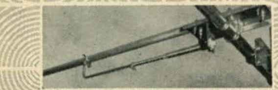
Now a feature of all three monobanders, the new, precalibrated (GAMMAXIAL) Gamma Match assembly with coaxially formed reactance cancelling capacitor built-in, makes possible for the first time a perfect 1:1 SWR. Coax connector for 52 ohm feed included. Developed by hy-gain's engineering staff and used exclusively in the hy-gain monobanders.
