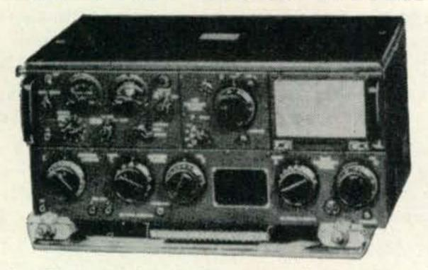
Designed to provide radio communication by voice, (MCW) or CW telegraphy. Class "B" audio modulator system capable of modulating the carrier at least 90% on voice or MCW. Incorporates automatic tuning mechanism which may be used to select any one of 11 frequencies, range 2000 KC to 18,100 KC. Frequencies 200 KC to 1500 KC range is provided by addition of oscillator O-16/ART-13A.
