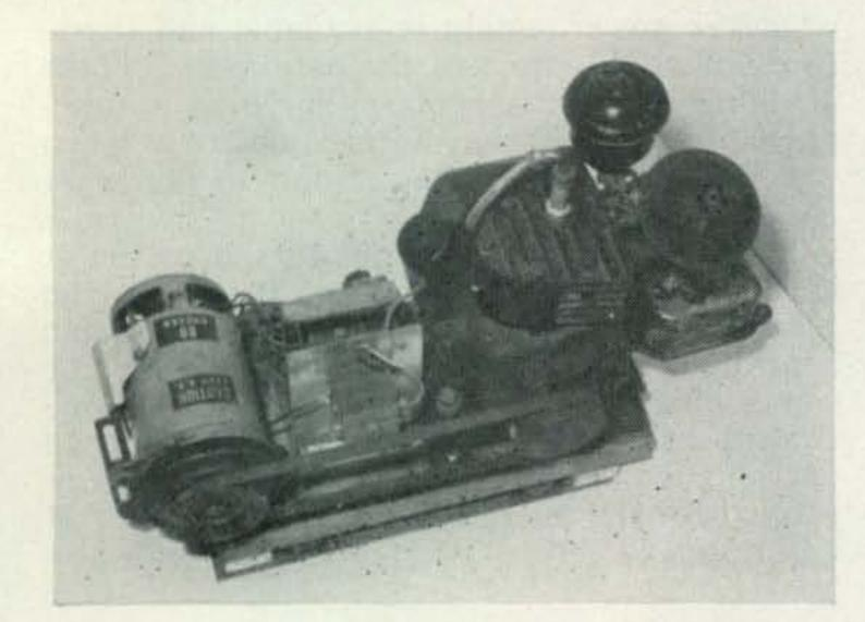
Here is a home-made puttputt that is inexpensive to build, very portable, and delivers just about 350 watts of 115 volt 60 cycle ac, enough to operate a receiver, 30 watt transmitter, electronic bug, Conelrad monitor, and a 40 watt lamp.
