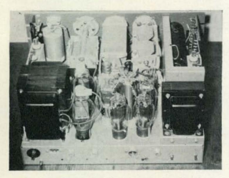
Despite use of all surplus parts, W9WNL's table top linear looks quite professional. The unit works all bands from 160 down to 10 meters, is completely self contained, has both pi and L networks in the output circuit and has a 2AP1 'scope built in for continuous monitoring. Five 837's in parallel, grounded grid operate at 1400 volts for a PEP input of 900 watts.
