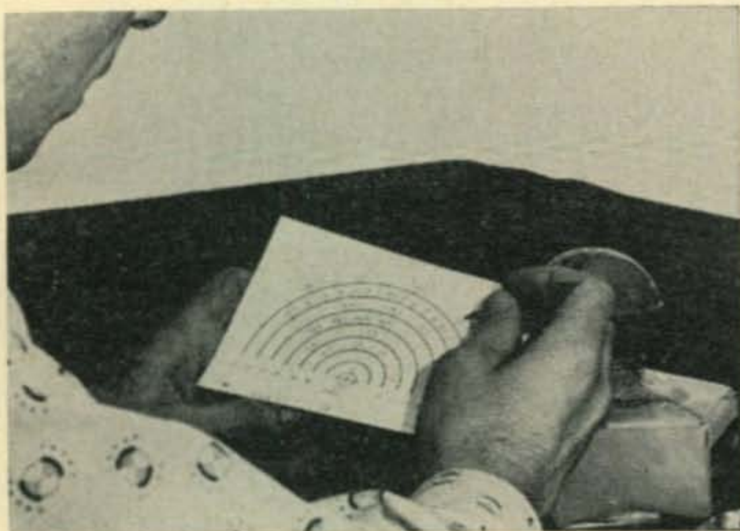
Fig. 3—A variety of numbers are available for the finished work dial. Electric typewriter numbers are shown being glued into place on the work dial, but a sheet of artype numbers worked out better on later dials for other gear.
