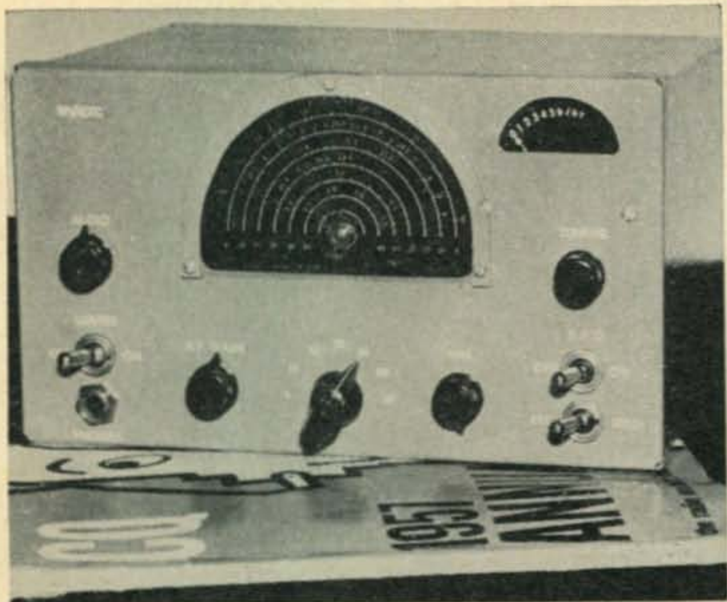
Fig. 1—Accurate, professional looking dial in place on a home brew all-band receiver. S-meter dial face was made the same way the main dial was.
