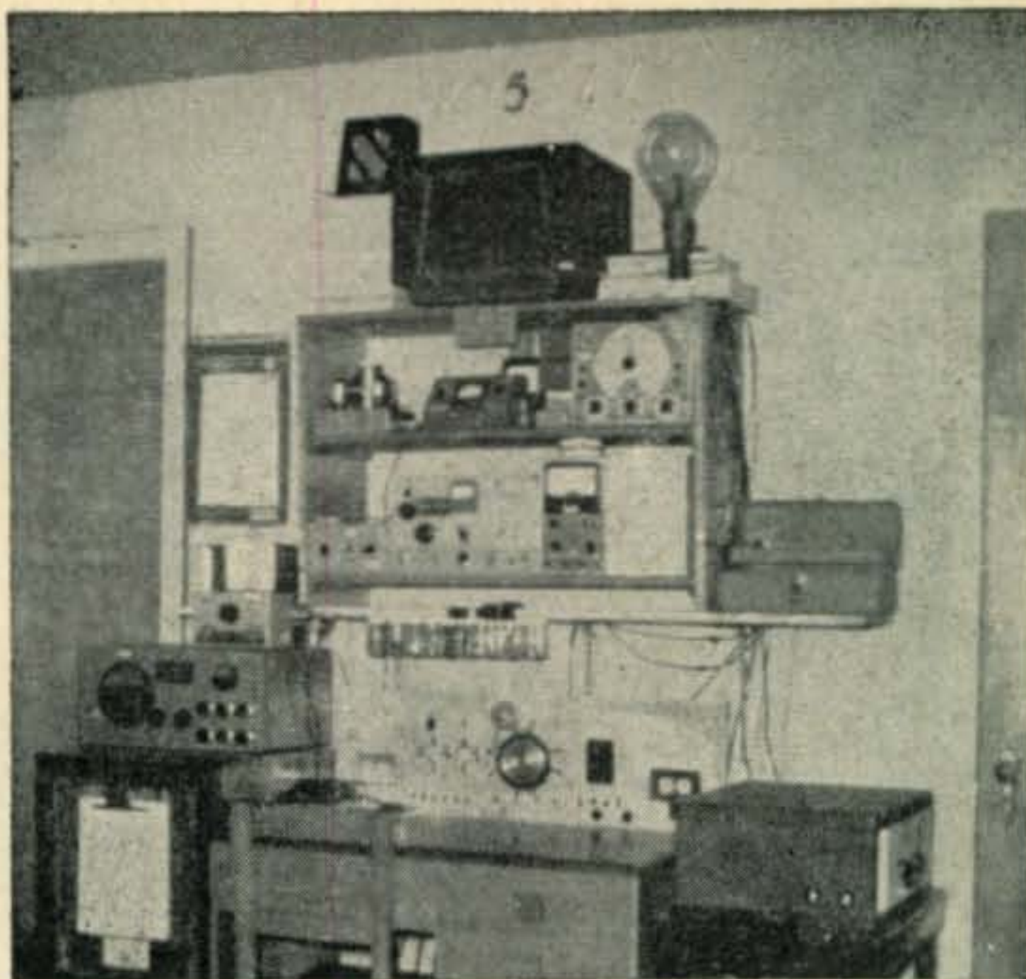
This is the neat station of Steve Moore, KN5SZV, 1504 Panhandle St., Denton, Tex. Steve runs an AT-1 modified with a 6146 in the final and an AC-1 antenna coupler. The receiver, as you can see, is an SX-43 with a Heath QF-1 for selectivity. Home brew QSL's are sent 100% if anyone wants a sked.
