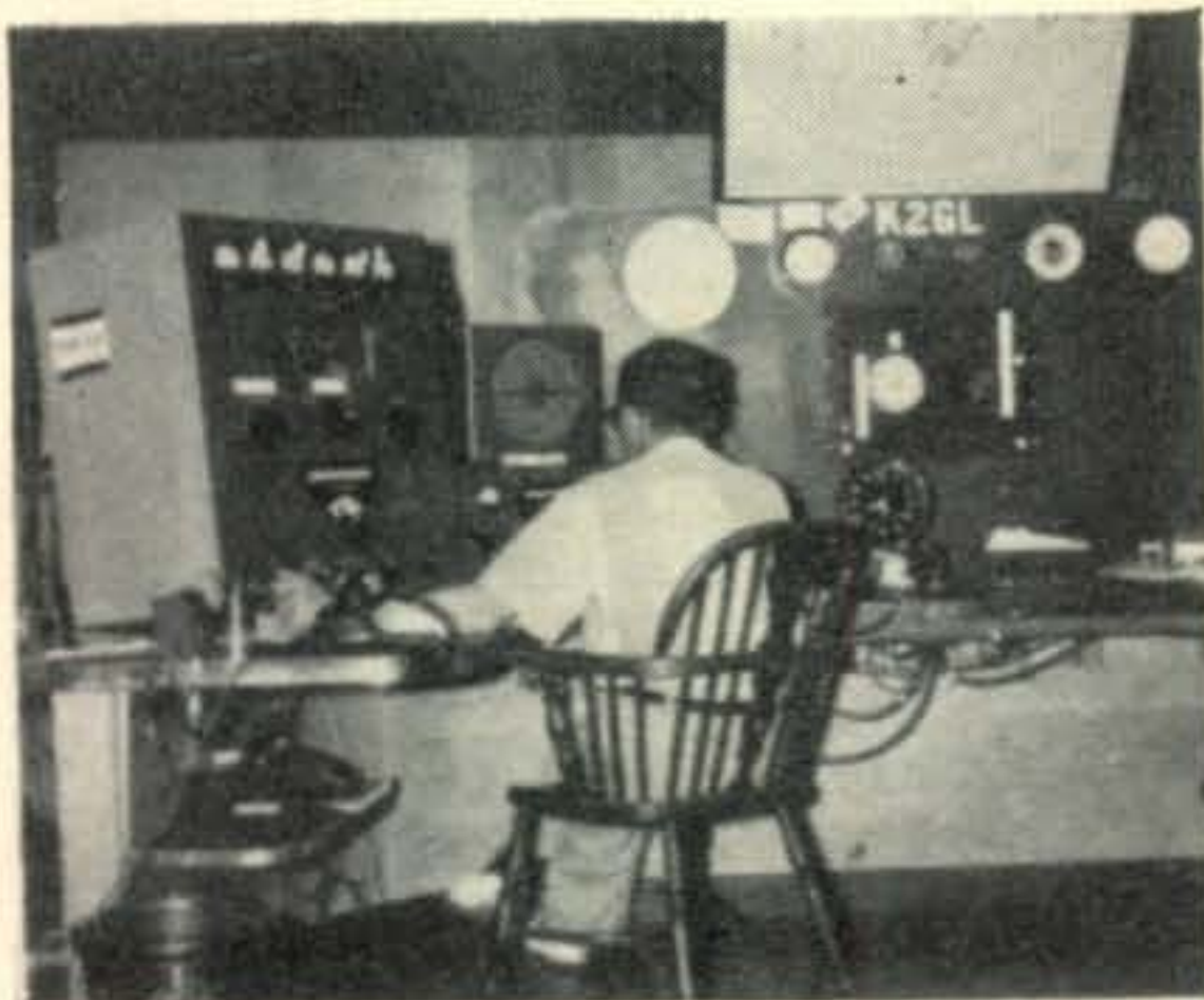
"Master control" of K2GL from which the activities of all four kw. phone rigs and an auxiliary KWM-1 were coordinated. Equipment included four 75A-4 receivers and choice of 12 different antennas.
