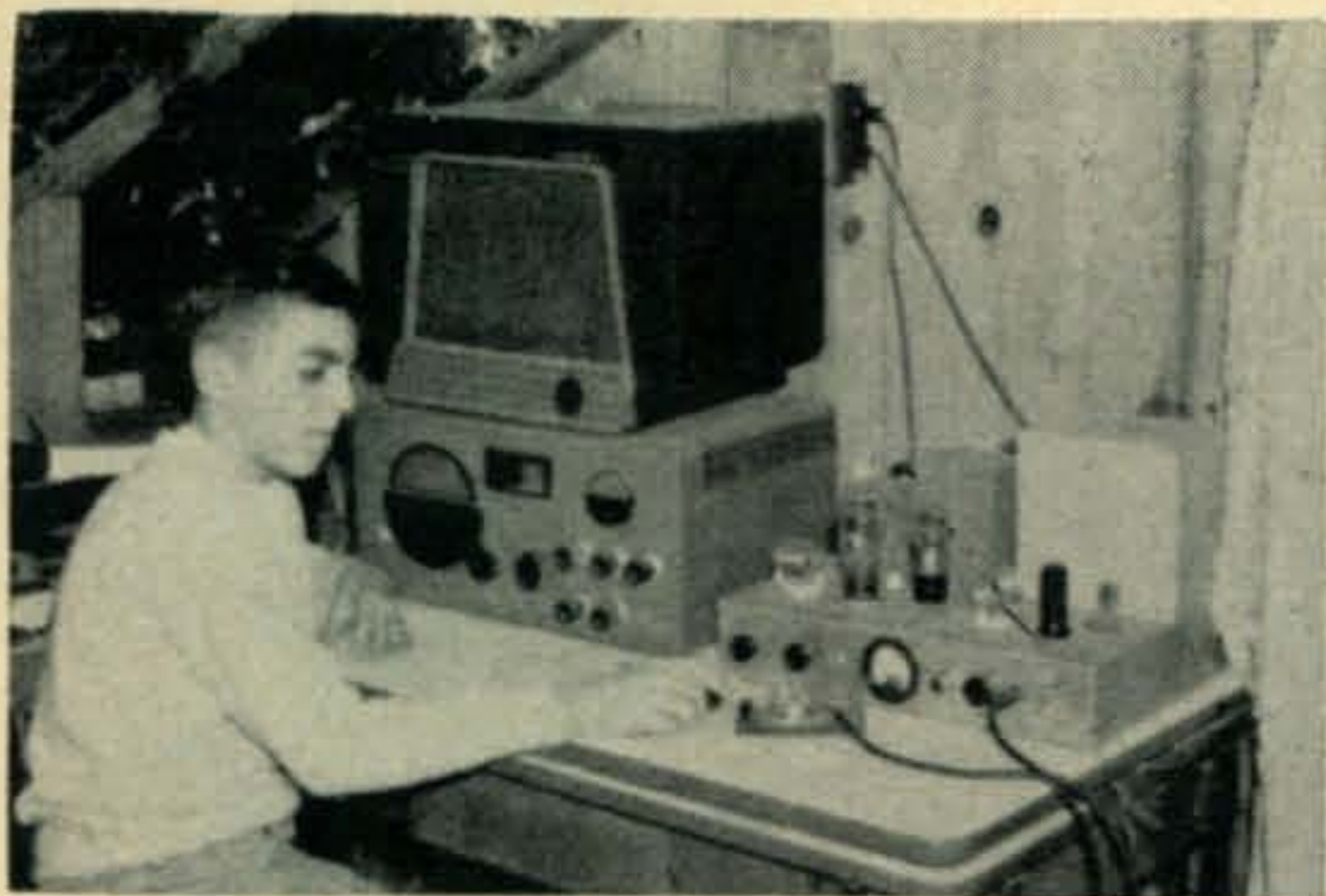
Michael Hunt, KN5TCQ, Rt. 1, Box 243, N. Biloxi, Miss. runs 25 watts to a home brew exhaler, and reproduces 'em with an SX-43 receiver. Look for Mike on 40.
