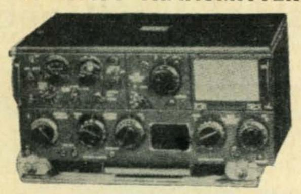
Designed to provide radio communication by voice, (MCW) or CW telegraphy. Class "B" audio modulator system capable of modulating the carrier at least 90% on voice or MCW. Incorporates automatic tuning mechanism which may be used to select any one of 11 frequencies, range 2000 KC to 18,100 KC. Frequencies 200 KC to 1500 KC range is provided by addi
