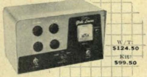
For 6-80M, complete with well-filtered power supply, 200w input AM Class B. 300w DC or 420w PEP input Class B linear SSB or DSB, 300w Class C for CW. Pi-Net 80-10M: 52 ohm Pi-Link coupled on 6M. Extensively TVI-protected, Meter for monitoring final plate currents also indicates approx. RF output voltage enabling operator to tune for max. efficiency and output.
