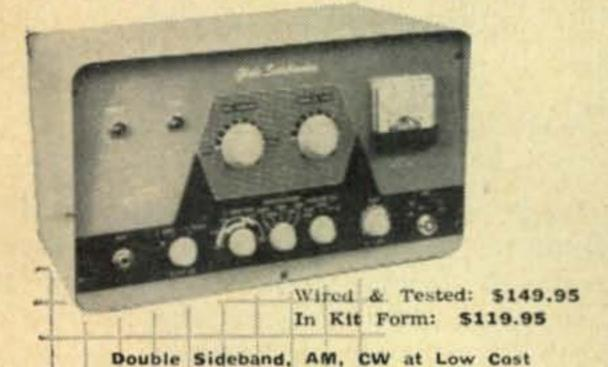
A complete Xmttr., self-contained, bandswitching 80-10M, 100w PEP DSB Suppressed Carrier, 40w AM, 50w CW. Min. 45db carrier suppression. 3-stage RF section allows straight through operation. Automatic balancing & floating grid circuit. Speech clipping & filtering for min. band width. Accessory socket on chassis rear apron. Use barefoot or as driver for higher power Xmttr. Covers most MARS and CAP fre-
