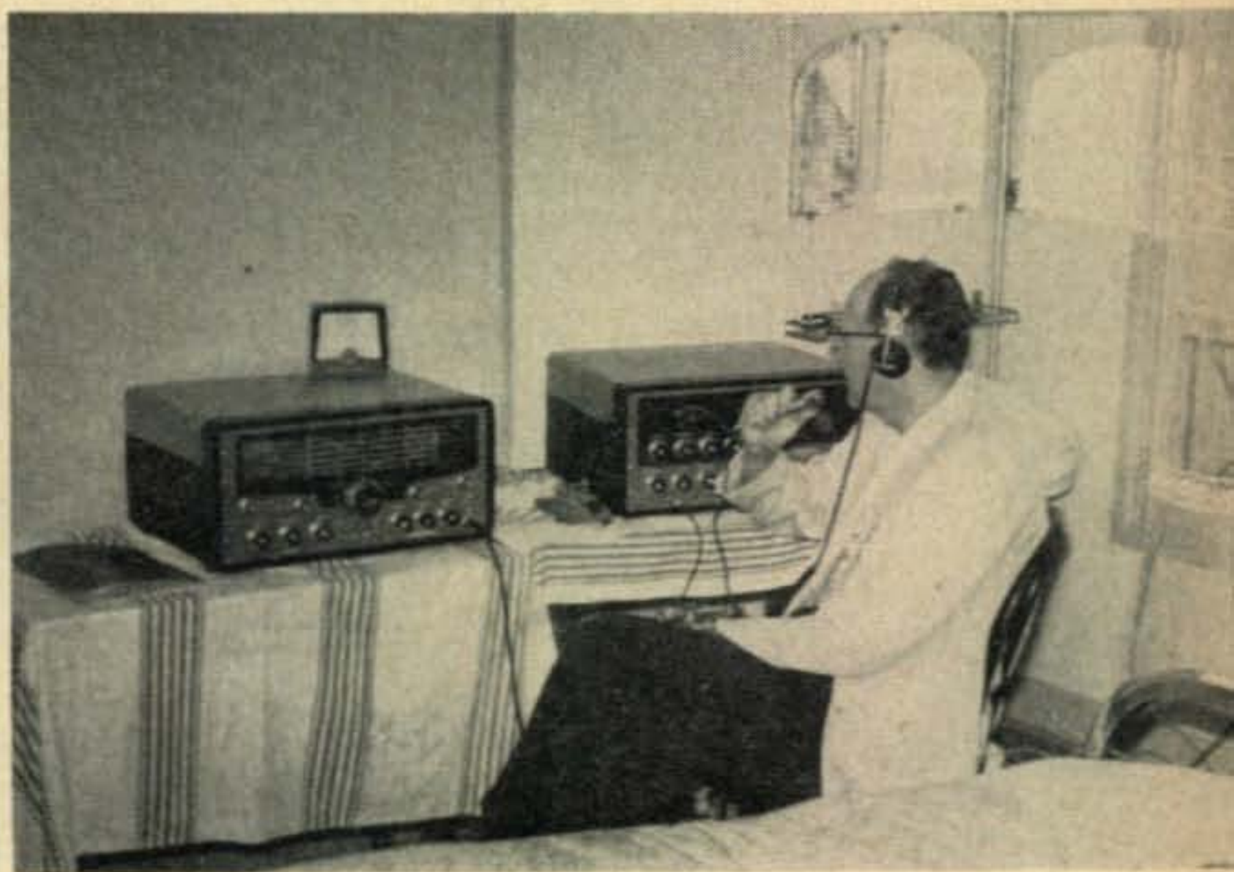
3A2AF was installed in a small room on top floor of Hotel Le Siecle. SX-101 and HT-32 performed in tip-top fashion in spite of surging line voltages, and light lines made of #22 wire. Over 1600 contacts were made with trouble-free operation. Occasional lightning storms were occupational hazard while working DX.
