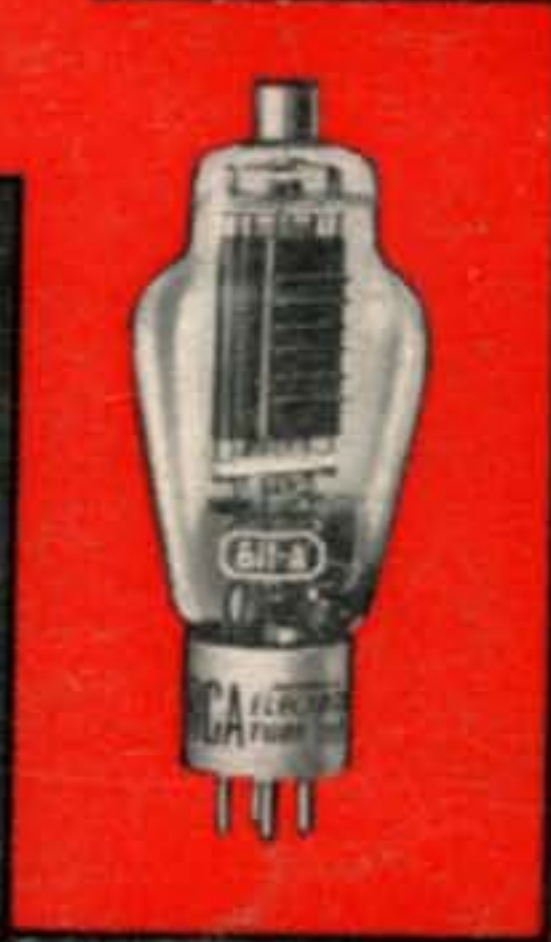
RCA-811-A. High-perveance power triode. Input: 260 watts, CW; 235 watts, SSB; 175 watts, AM- phone.
