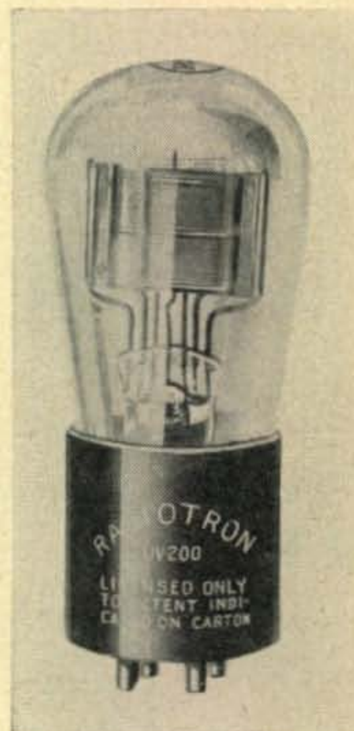
UV-200 detector tube. Similar in size to the 201As, these tubes were 50% more sensitive than crystal detectors.
