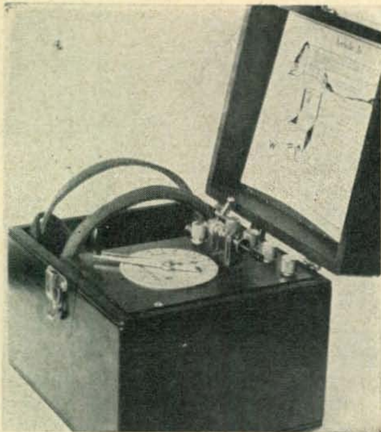
Single circuit crystal set. First popular-priced home radio receiver, the Westinghouse Aeriola, Jr. Courtesy of Westinghouse Mfg. Co.
