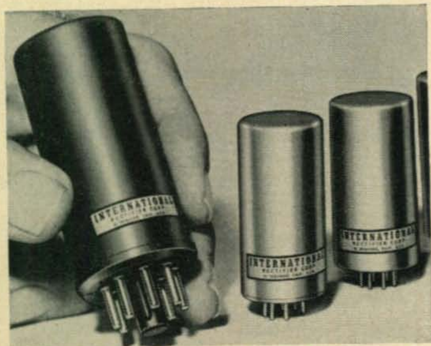
International Rectifier Corp. has a new series of plug-in silicon replacements for vacuum tube rectifiers, with piv's between 1500 and 2800 volts at 85 to 600 ma.
