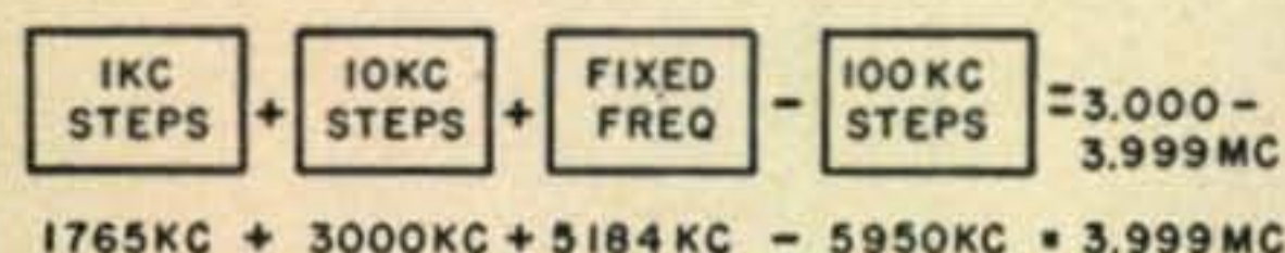
Fig. 2—Mixing procedure used to produce a minimum of spurious outputs.
