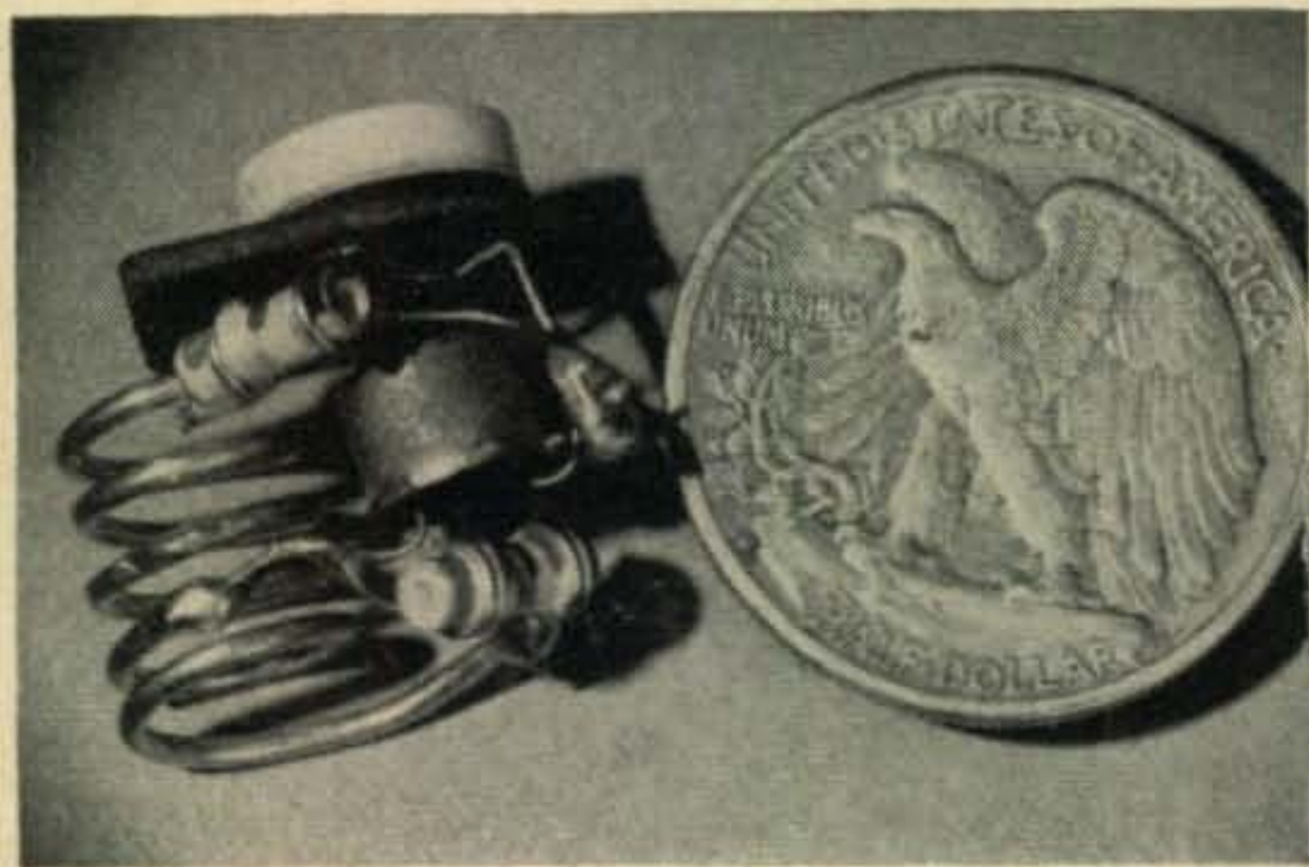
A complete tunnel diode transmitter compared to a 50-cent piece. It consists of a variable and two ceramic capacitors, a coil and the tunnel diode.
