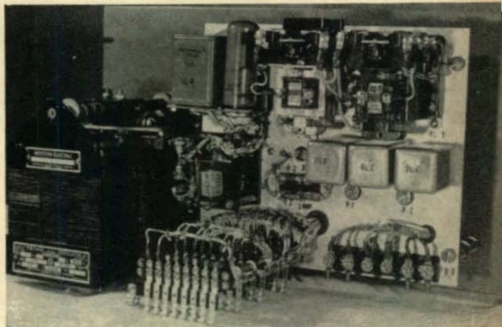
Rear view of the Panel. Note the removable relay mounting plate and terminal strips for interconnection with other units of the transmitter.
