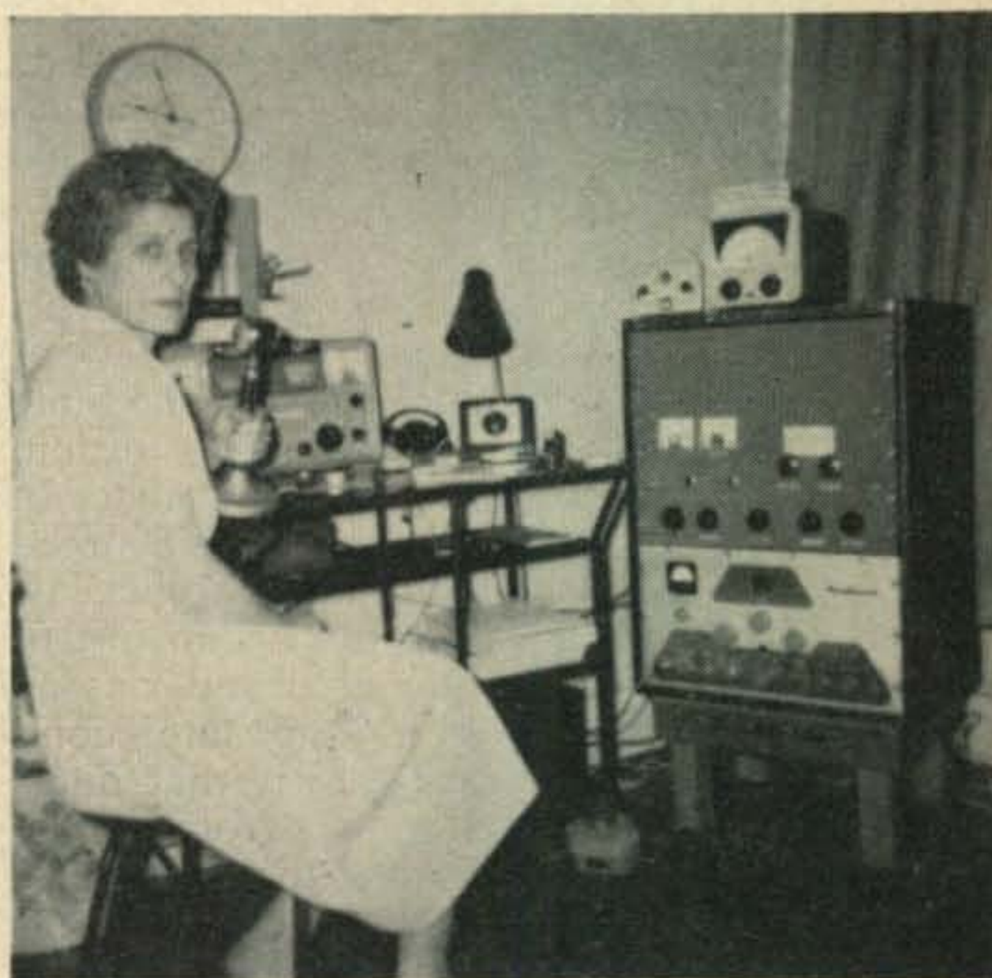
Ethel Robison, K4HPX, one of the active YL's on six meters. Equipment: DX100 to 829B final, about 160 watts to 8 element HyGain Beam.
