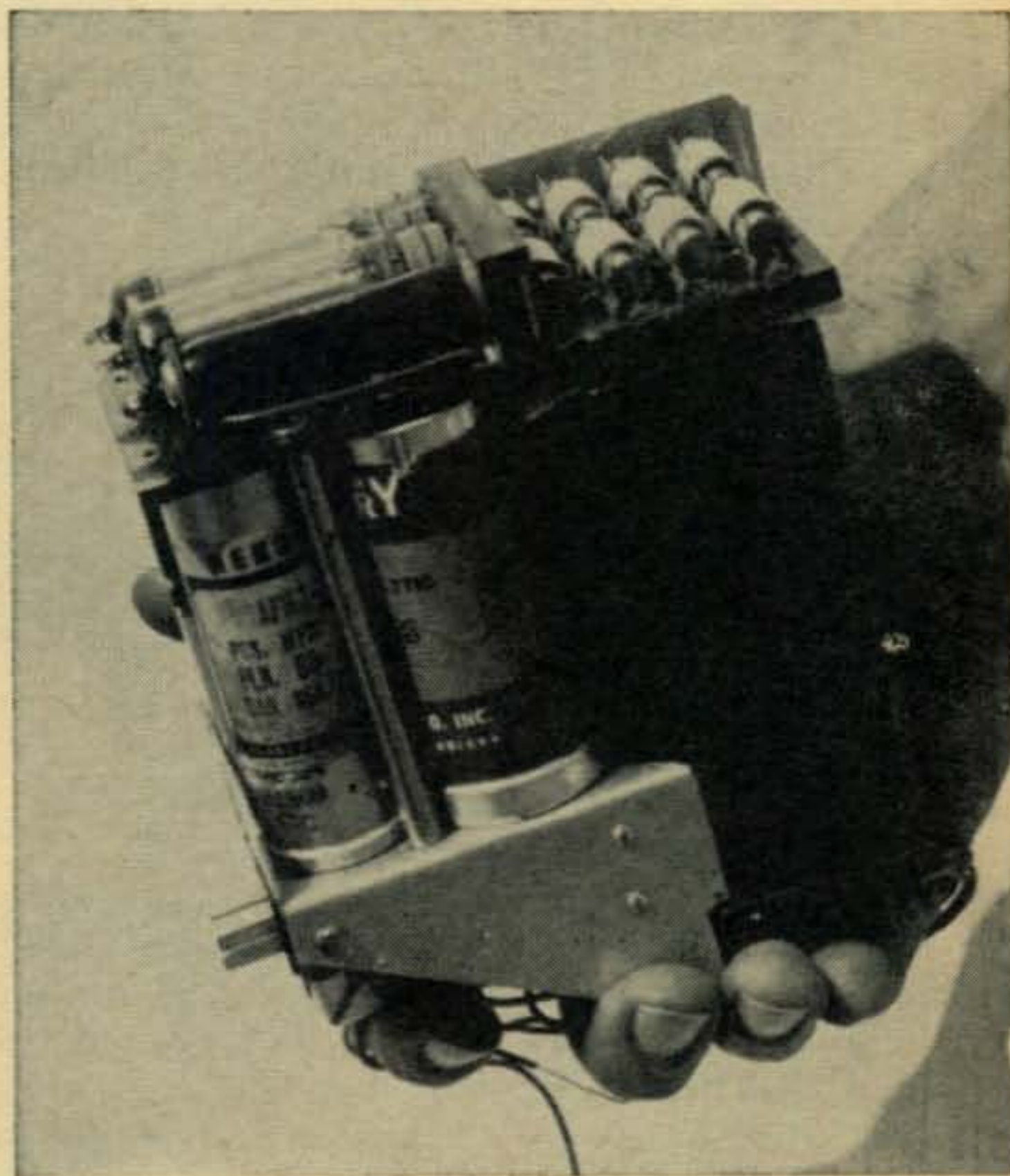
The 110-220 vac power supply. It delivers 450 volts at 125 ma, 125 volts at 120 mg, 300 volts regulated and 6.3 volts for filaments.
