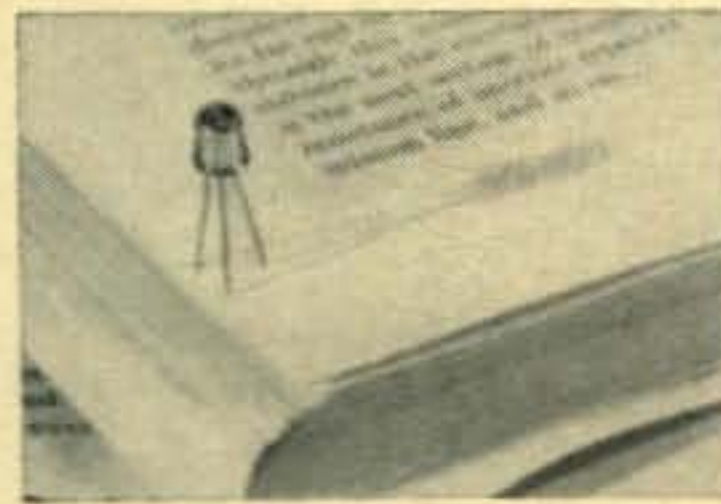
Contrary to earlier reports in this column, General Electric is currently selling gallium arsenide tunnel diodes. This unit is packaged in the standard JEDEC TO-9 case and is rated to 1,000 mc .
