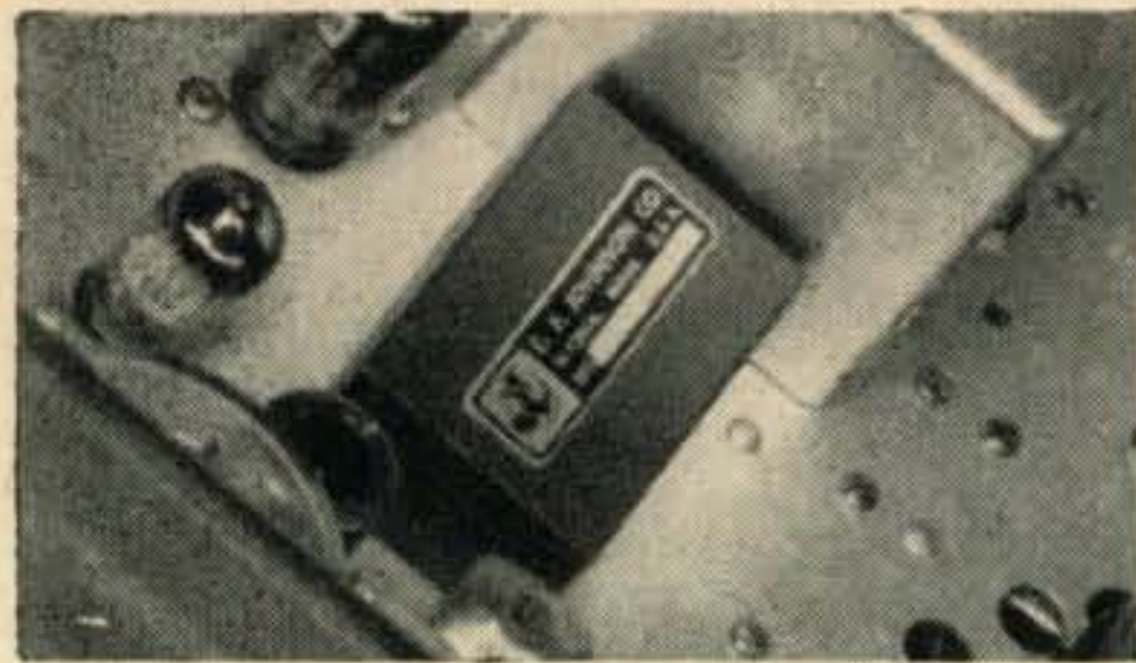
FILTER-TYPE SIDEBAND —Exclusive high frequency bandpass filter gives you more than 60 db of unwanted sideband and carrier suppression! Select upper or lower sideband instantly with front panel "mode" switch.
