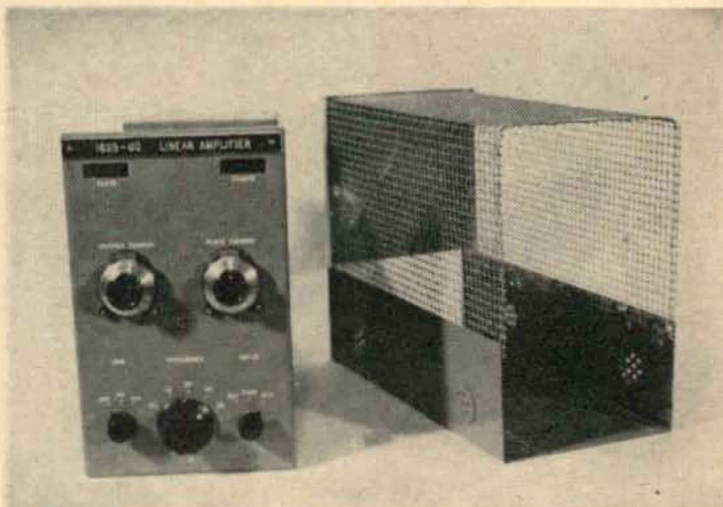
Front panel layout and enclosure design of the 1625 grounded grid amplifier. Vent holes in the bottom of the shield enclosure match with holes drilled in the ARC-5 chassis. Forward and Reflected positions of the meter switch are used with an external bridge.
