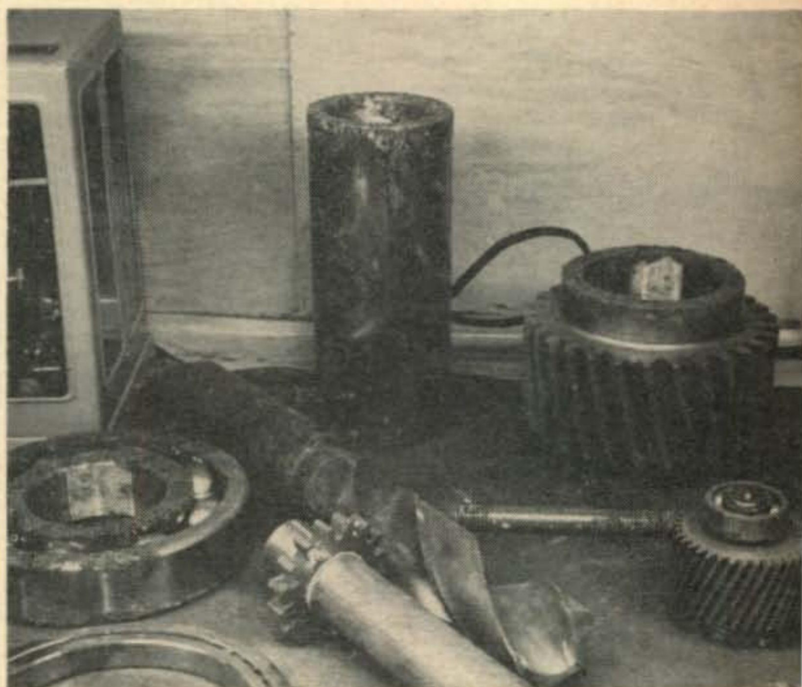
Fig. 2—Specimens exposed to 70 to 80% relative humidity continuously. Steel specimens show localized pitting and encrusted rusting. Organic specimens (not shown) were mildewed.
