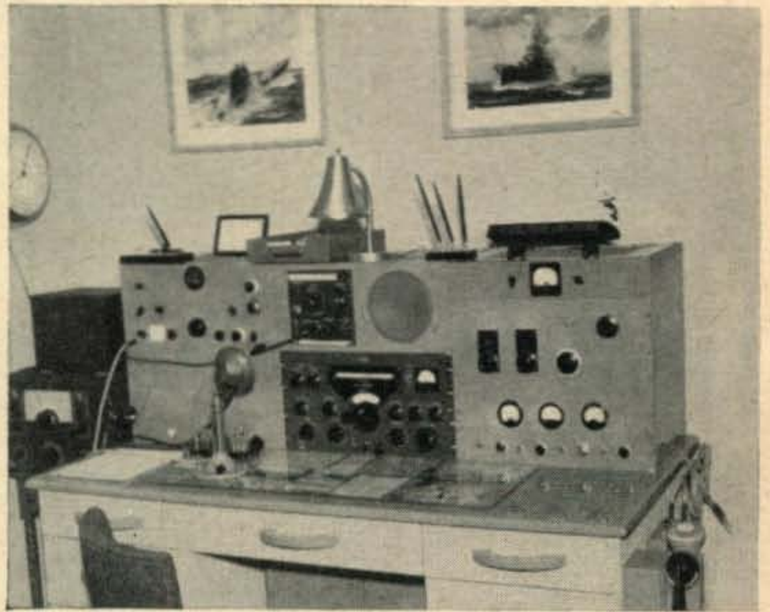
Operating position at W3JHR. To the left of the BC-221 is the exciter and to the right of the Collins 51J receiver is the linear amplifier.
