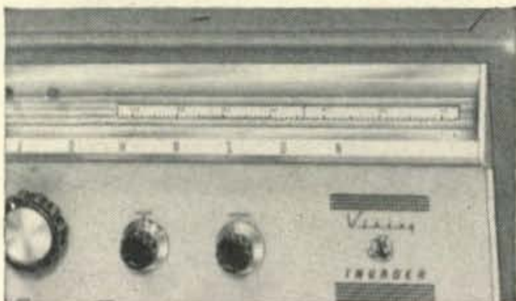
FREQUENCY CONTROL —Instant bandswitching coverage of the full 80, 40, 20, 15 and 10 meter bands... no extra crystals or retuning required. Highly stable, built-in VFO is differentially compensated and factory adjusted for maximum stability—exclusive "keep warm" heater element keeps VFO at operating temperature even with equipment turned off... NO WARM-UP DRIFT!
