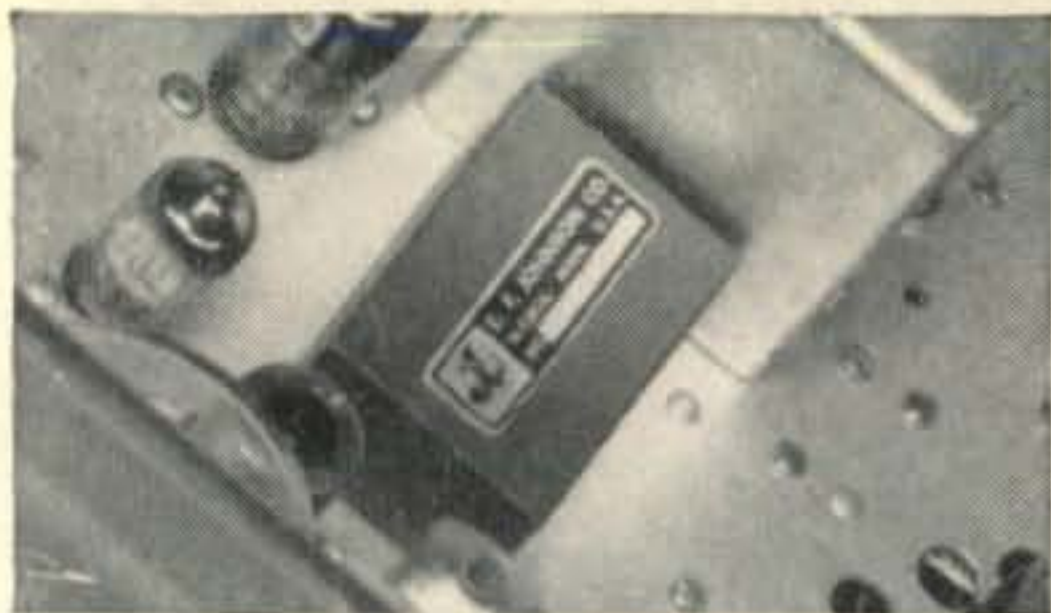
CRYSTAL FILTER-TYPE SIDEBAND —Exclusive high frequency bandpass crystal filter gives you more than 60 db of unwanted sideband and carrier suppression! Select upper or lower sideband instantly with front panel "mode" switch.
