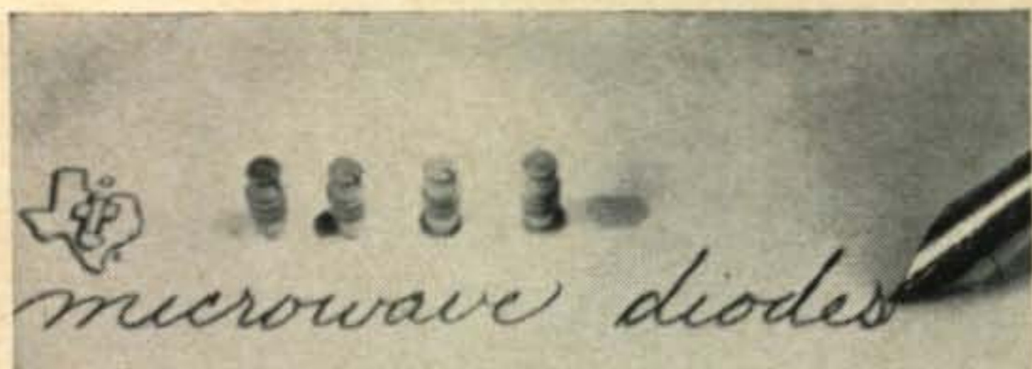
Varactor diodes made by Texas Instruments are capable of operation up to 144 kmc .
