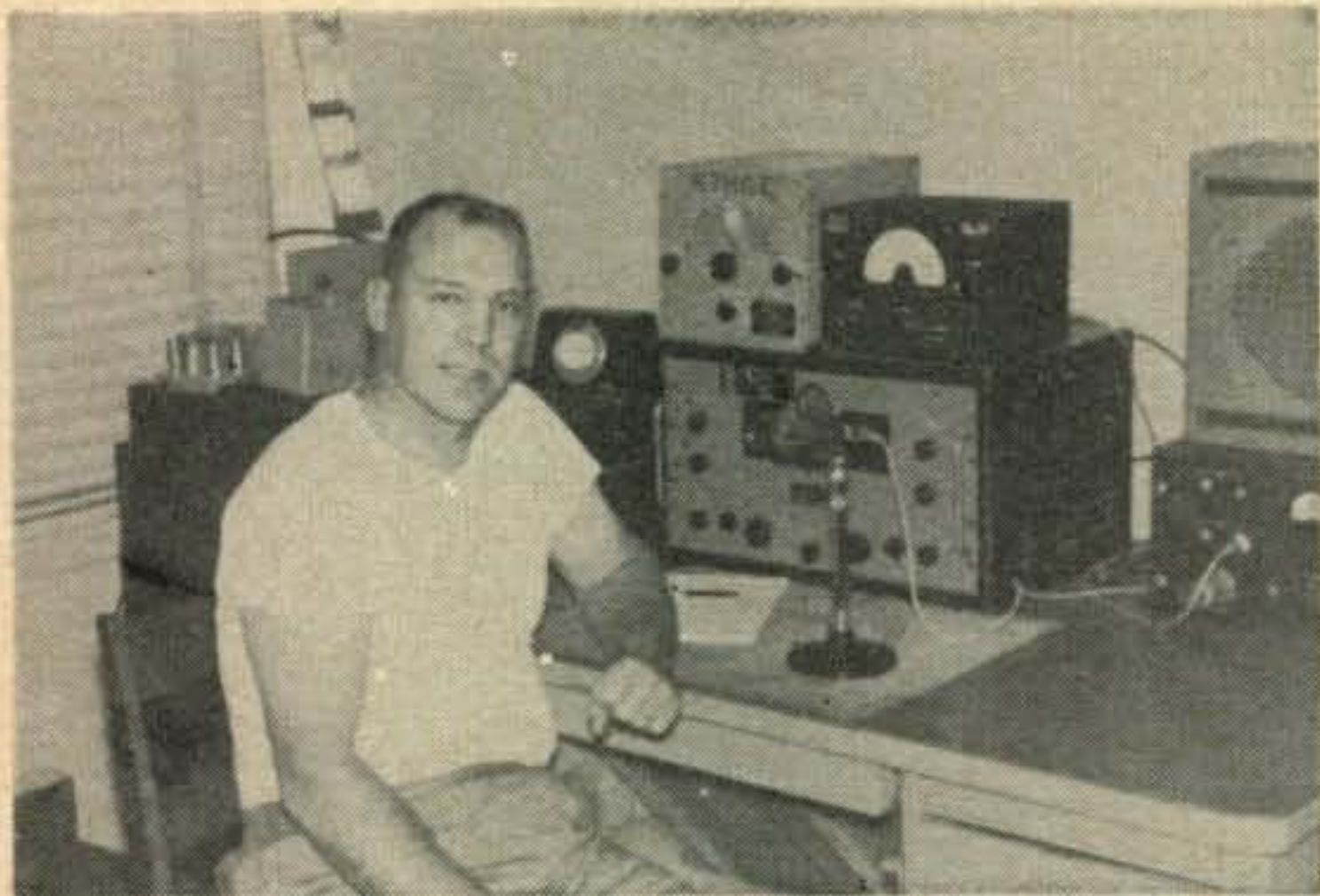
Bill, KA2BF sit comfortably in front of his BC-610. A consistent signal on 14 mc, Bill will soon be on 21 and 28 mc.
