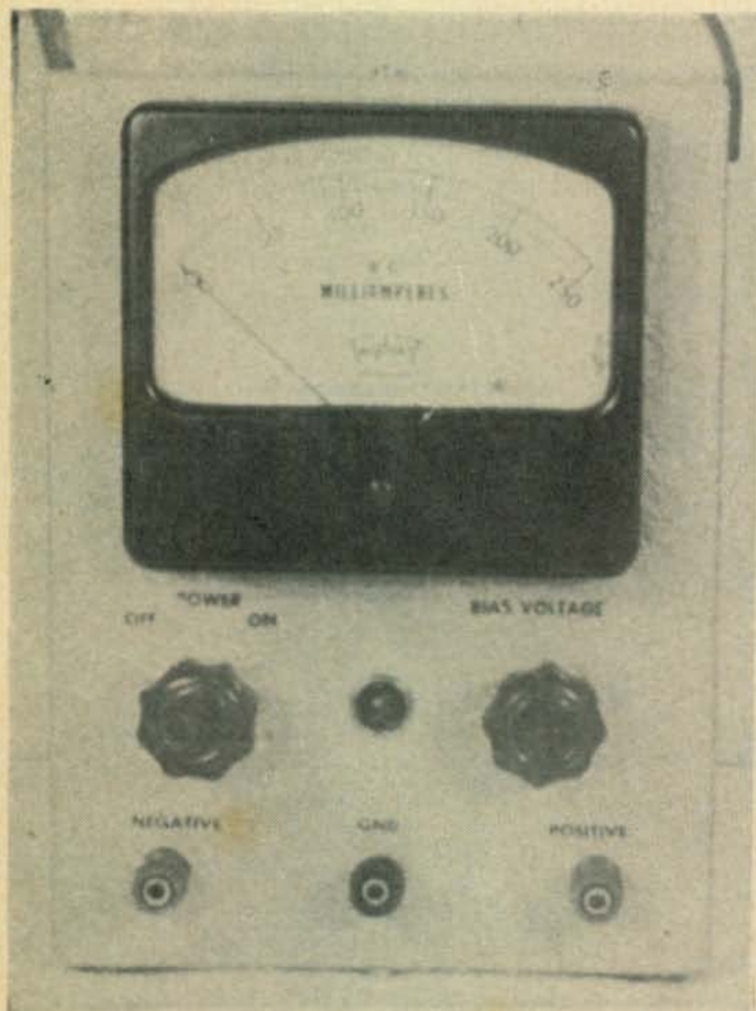
Front panel of the adjustable load. Varying the bias voltage control varies the current drained by the parallel 6BG6s. The load current is measured by the milliammeter. Direct connection to the meter can be made through the terminals marked - +.
