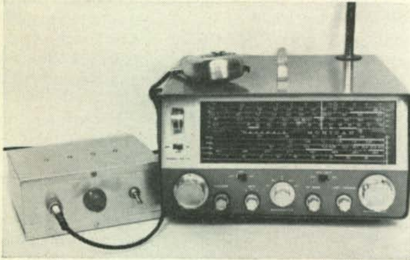
Overall view of the completely transistorized two meter station described herein.
