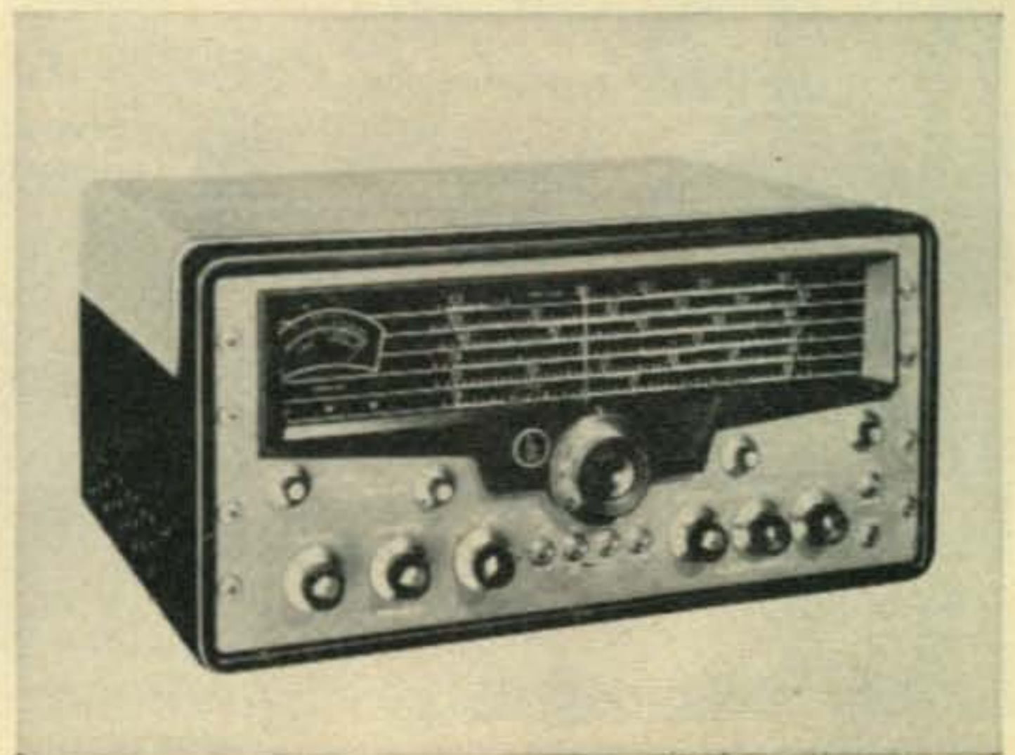
A Hallicrafters restricted coverage receiver. Note the single dial, one knob tuning and wide spacing of the dial frequency markings.
