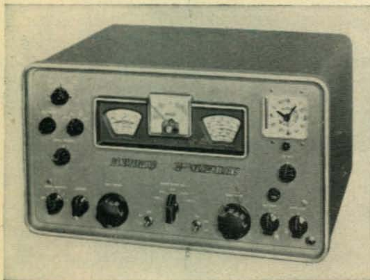
A Hammarlund general coverage receiver incorporating a separate dial for general coverage and one for bandspread.
