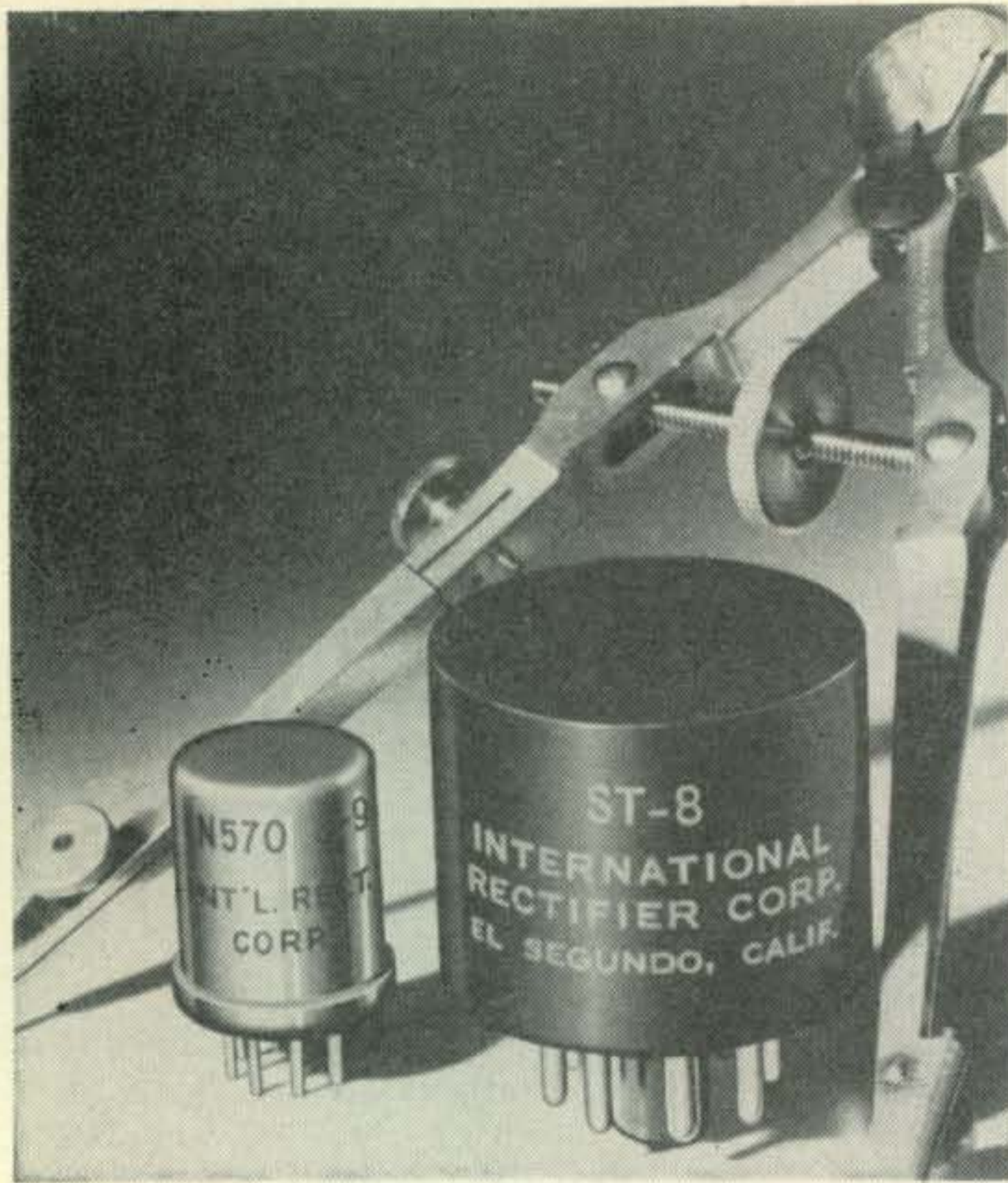
International's tube replacement type high voltage silicon rectifiers. (Courtesy of International Rectifier Corp.)
