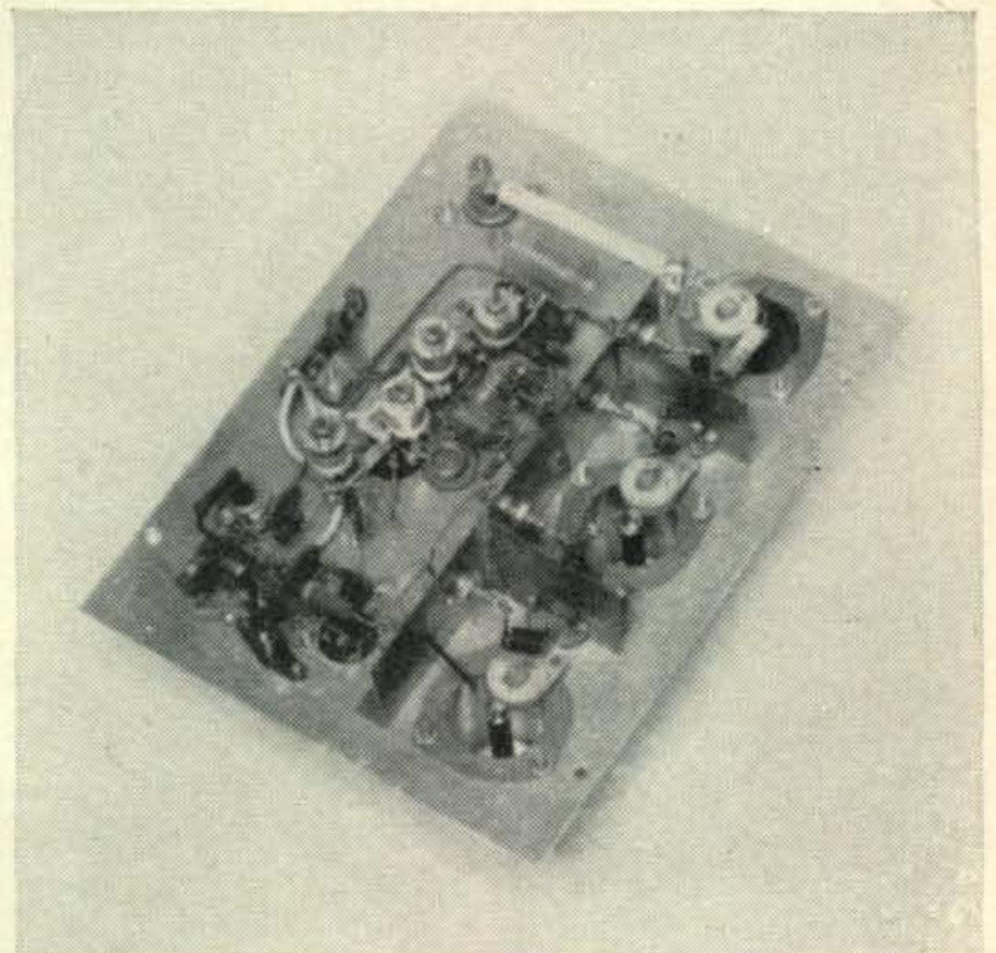
Underside of the crystal controlled converter for 432 mc in use at LU3DCA.
