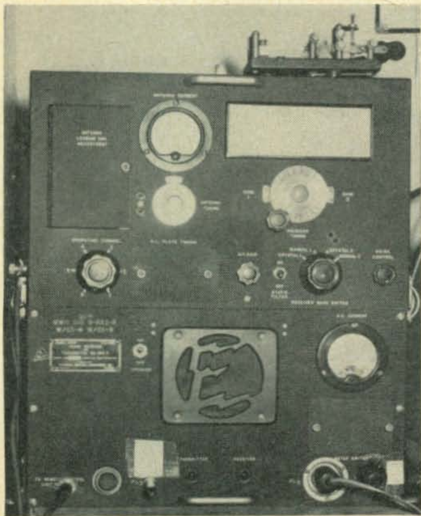
Front view of the BC-669. The upper deck contains the transmitter and receiver and the lower deck houses the modulator and speaker. An outboard power supply, described on page 28, must be added.
