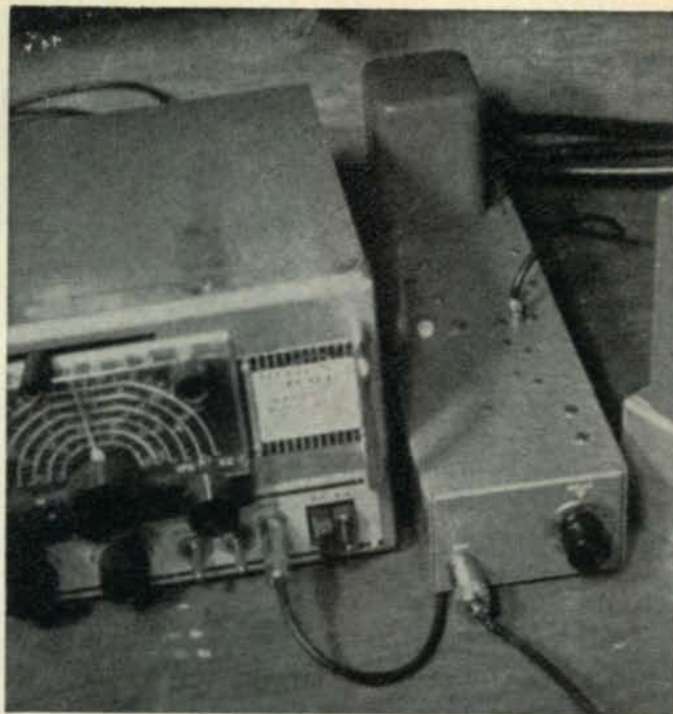
The unit in operation. Rear lead connects to transmitter key jack. The monitor is not shown.
