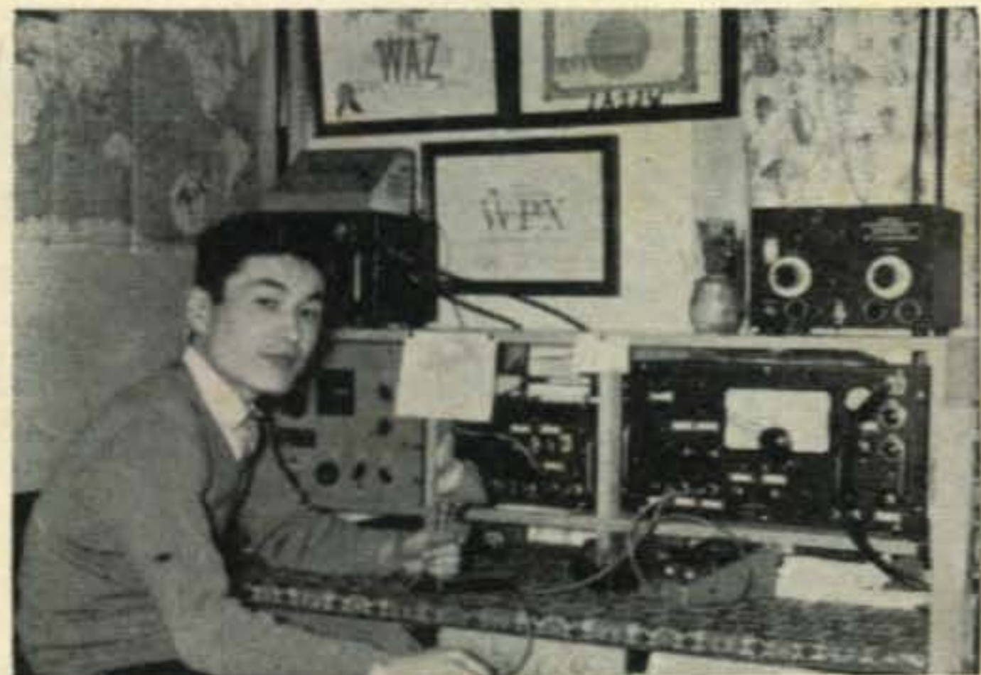
Yoh, JA2JW, can always be counted on to put a signal into the states when the band is open. Here we see his complete home-brew station, with the exception of a BC-778. The exciter is used on c.w., a.m. and s.s.b. (Txn K2UKQ)
