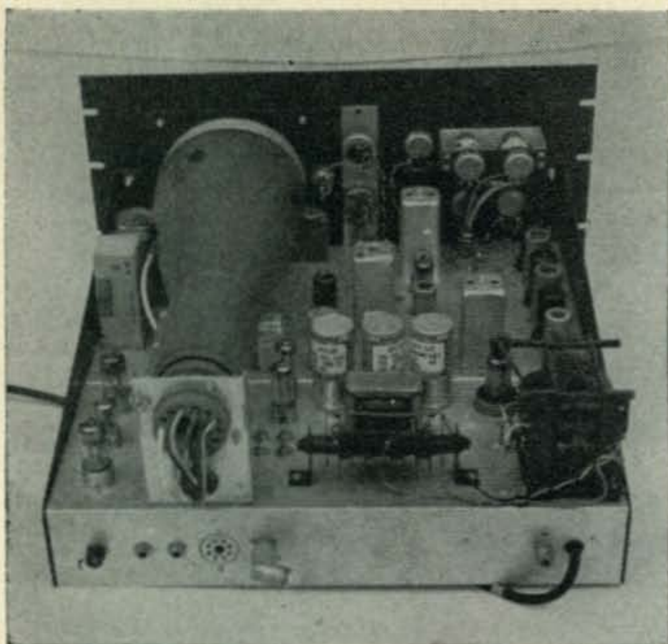
Rear view of the spectrum analyzer. The components on the rear of the chassis are, l to r; R_{25} , Sweep Linearity; J_4 , Horizontal Output; J_3 , Vertical Output; J_2 , Accessory Socket; J_1 , 455 kc Input and Hum Balance pot. The stud mounted silicon rectifiers, CR_2 to CR_5 , used in a bridge circuit for d.c. filament supply, may be seen to the right of the neck of the 5CP7A.
