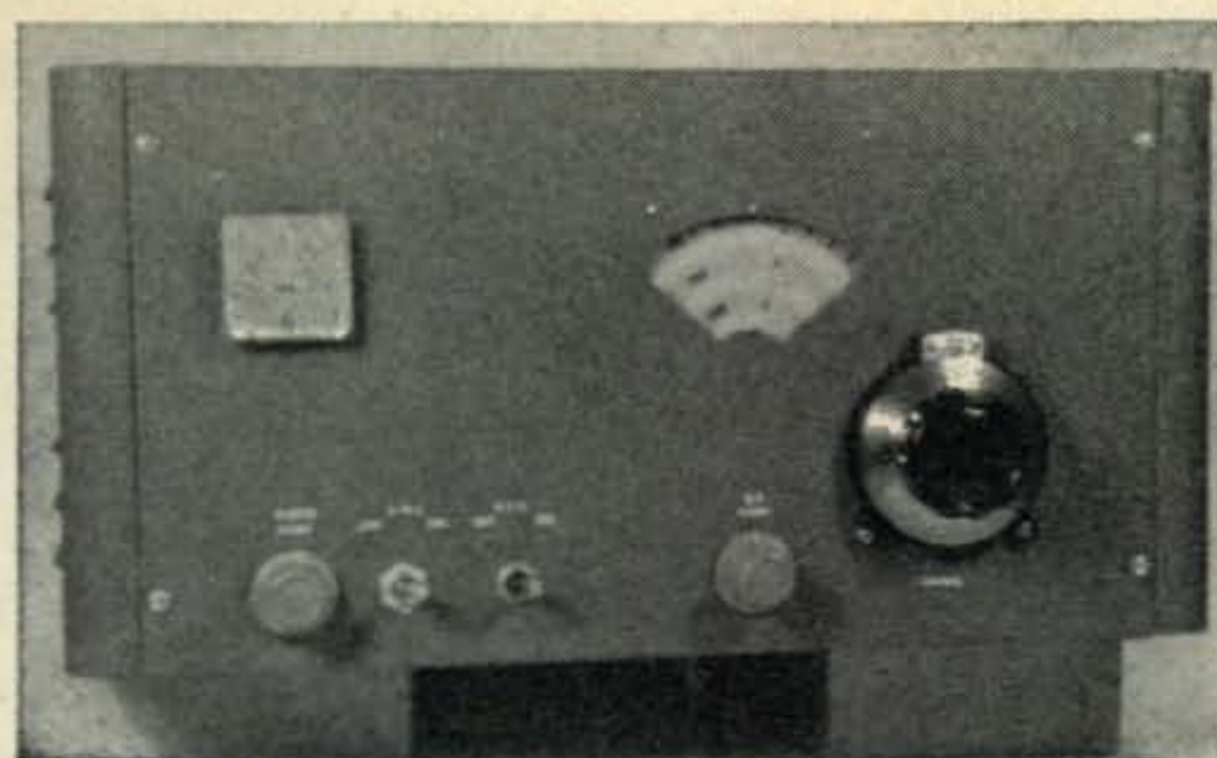
Front view of the 6 meter receiver. The controls are, from l. to r., Audio Gain, A.N.L., A.V.C., R.F. Gain and Tuning. The dial system, home brew, is driven by a vernier dial mechanism.
