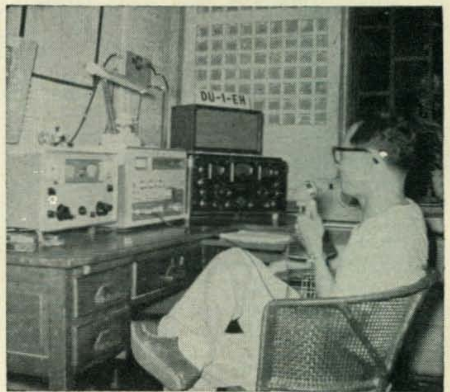
The shack, operator, and antenna of DU1EH, who is one of the newer Philippine hams. The rig is an HQ-110, Apache and homebrew minibeam and rotator. That's a fine looking job on the tower and beam. (Tnx DU1RTI)
