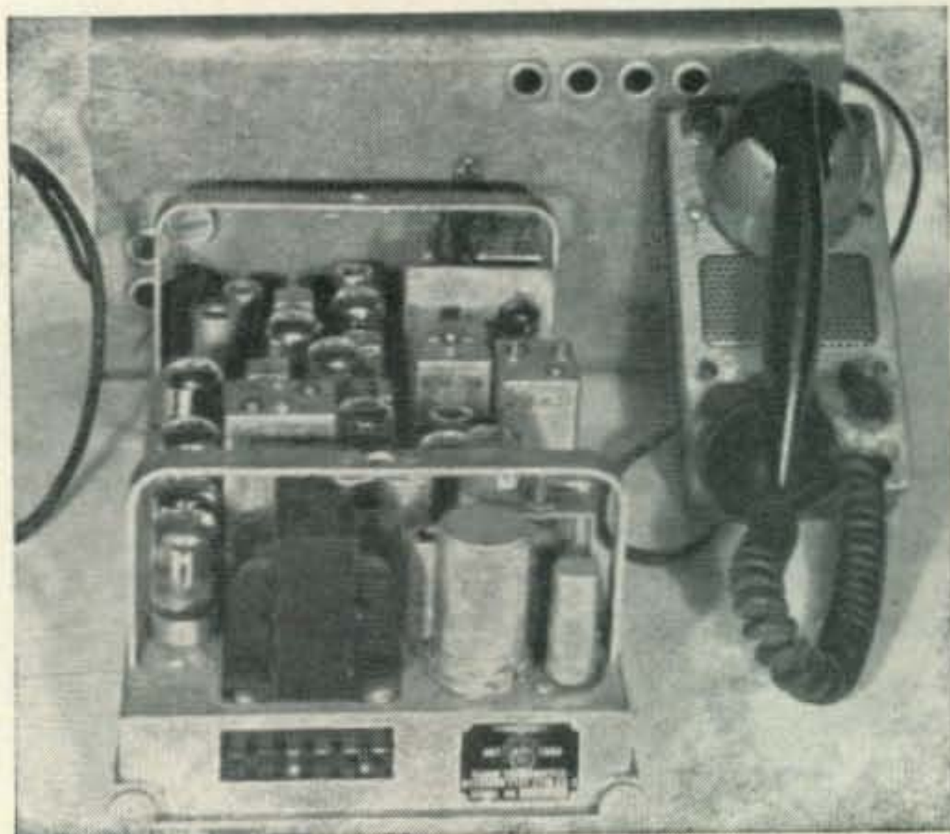
View of the Link 2210 showing the chassis, chassis cover and control head. The Jones plug on the chassis is for connection to the control head. The 2365 unit is identical in size but slightly different in appearance.
