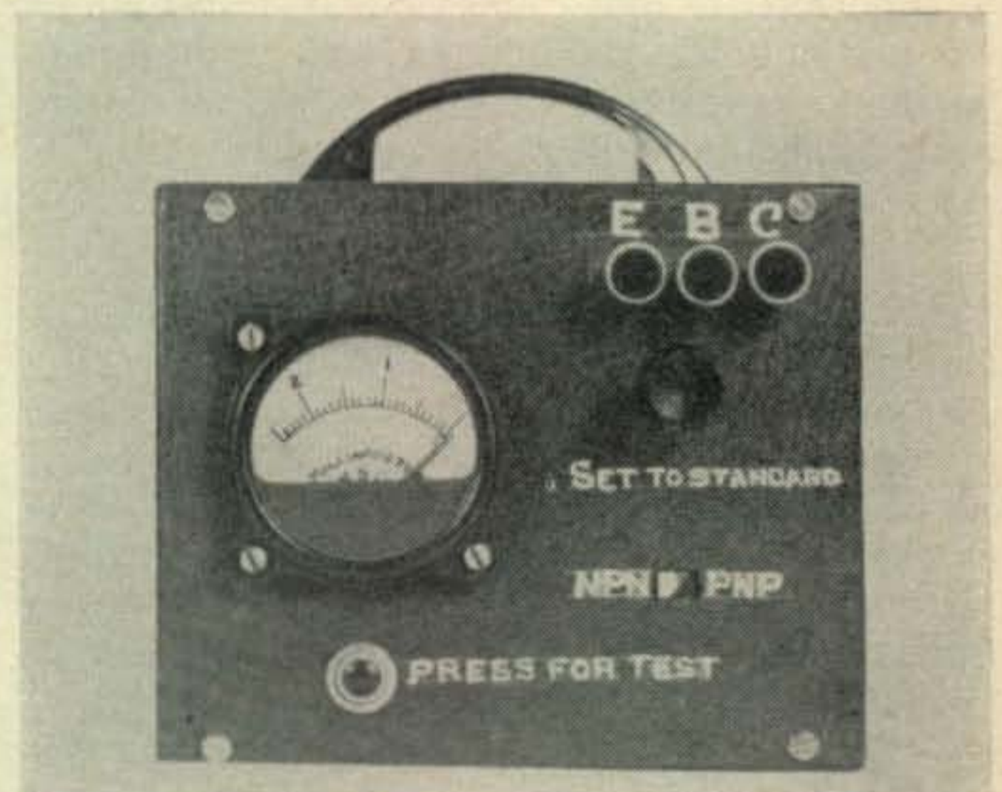
Panel view of the handy transistor tester. The zero to 2.5 ma meter may be replaced with a zero to 1 ma meter if greater sensitivity is desired. See text.
