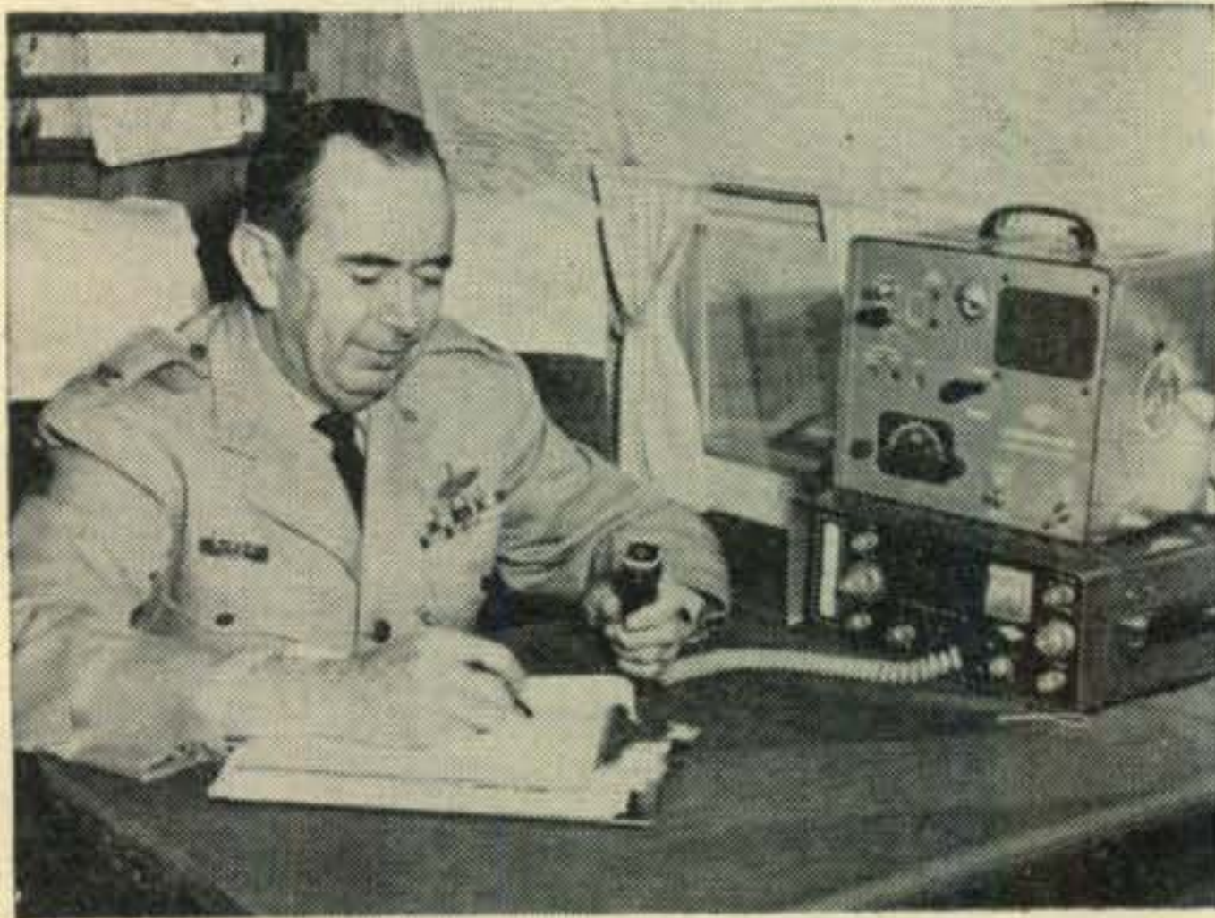
Col. John W. Riggs, K8WRT/AFA8WRT, 1223 Earlham Drive, Dayton, Ohio is shown at the operating position in the C-47 used as an experimental air-borne net control station for the 2 m MARS net. Col. Riggs is the MARS director at the Dayton Air Force Depot, Dayton, Ohio. The experiment was a great success.
