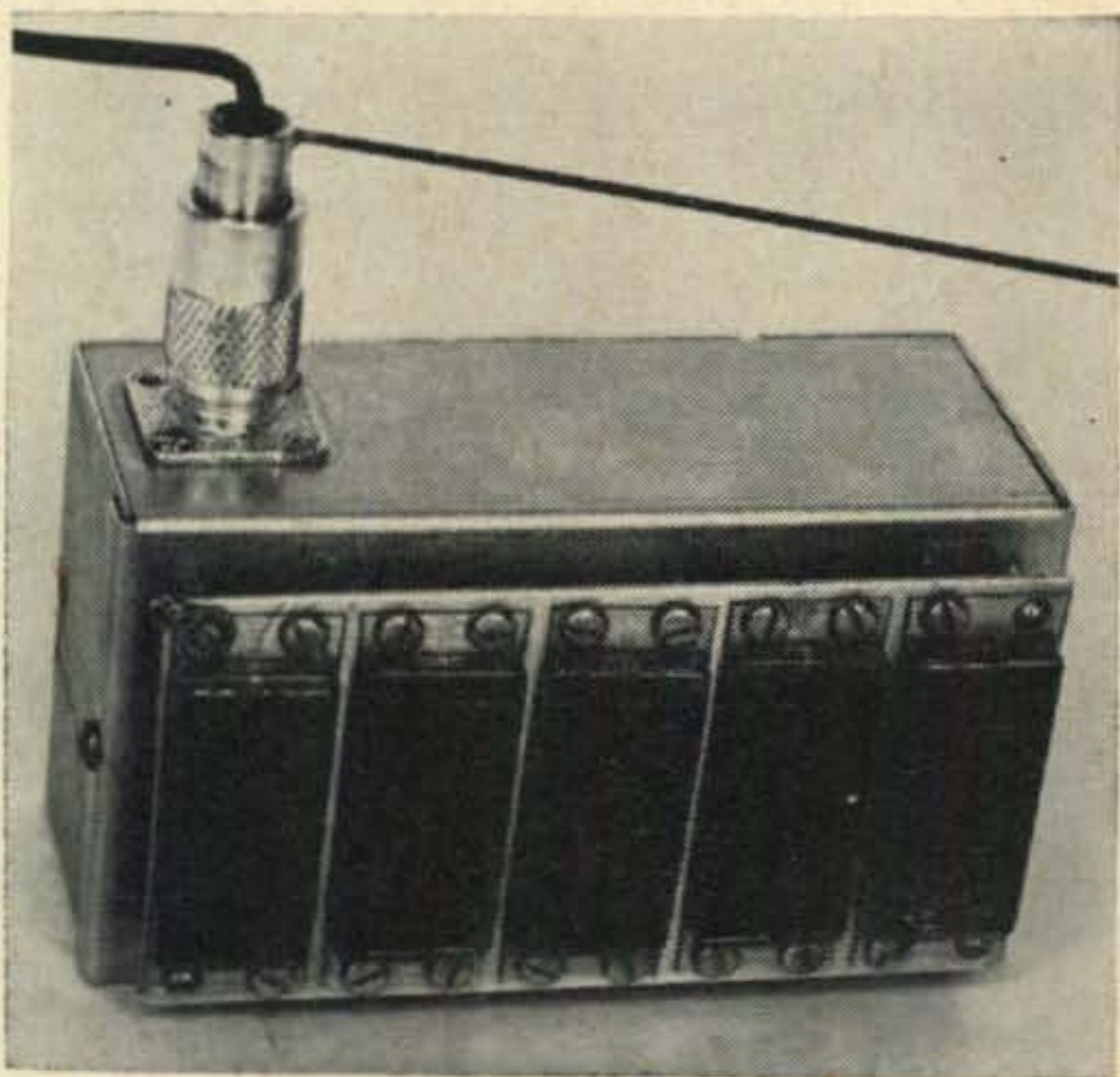
Front view of the QRP transmitter showing the solar cell shingles. The dipole antenna was mounted directly on the case.
