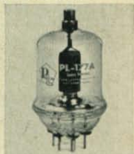
PL-177A 75W beam pentode. To 175mc. Highly efficient at plate voltages as low as 600v.
