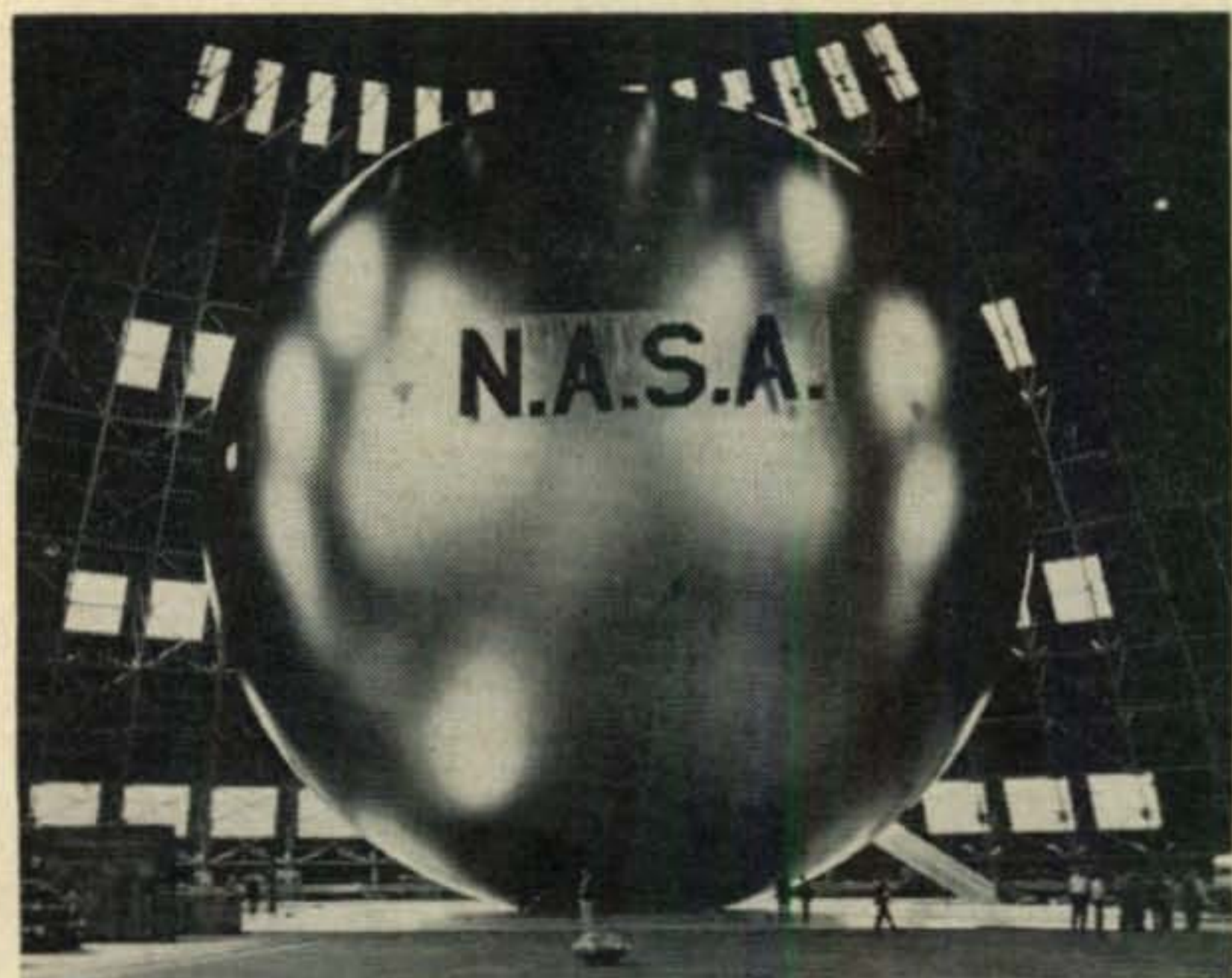
Shown here is ECHO II, the 135 foot diameter rigidized inflatable balloon satellite which NASA plans to launch this coming summer as a passive reflector of radio signals. When folded, the satellite is packed into the 41 inch diameter canister shown in the foreground. (Official NASA Photo).
