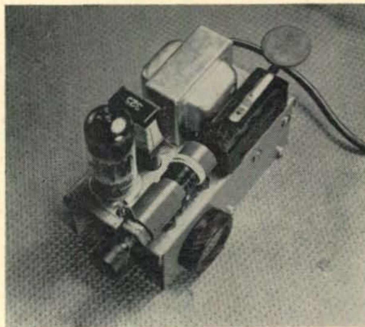
Top view of the transmitter showing component locations. The key is a microswitch with a home made knob attached.
