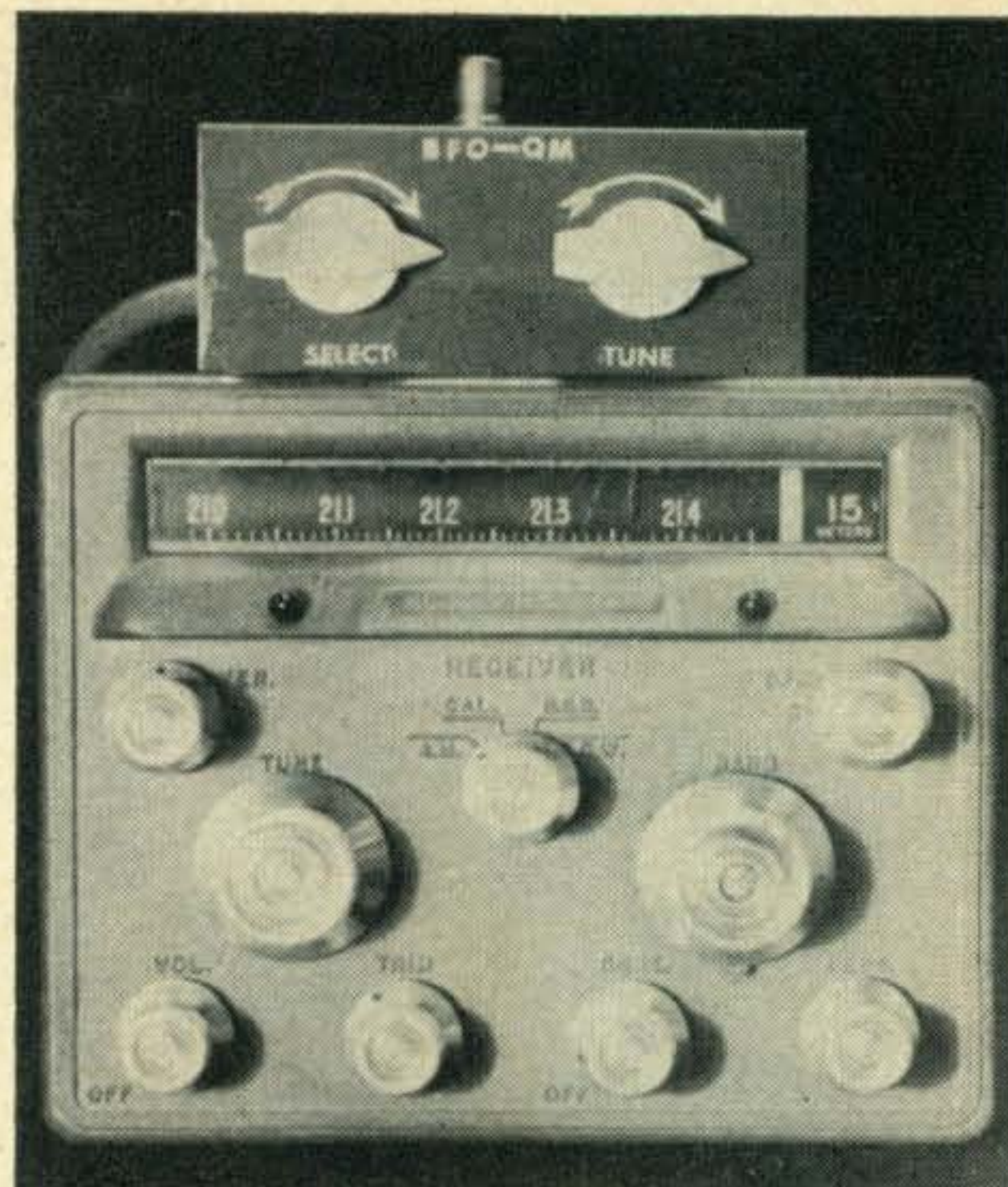
The Combo-B.F.O.-Q-Multiplier in use on a Peirson KE-93 receiver. The KE-93 has a 265 kc i.f., so the information in the preceding article was put to use for this installation.
