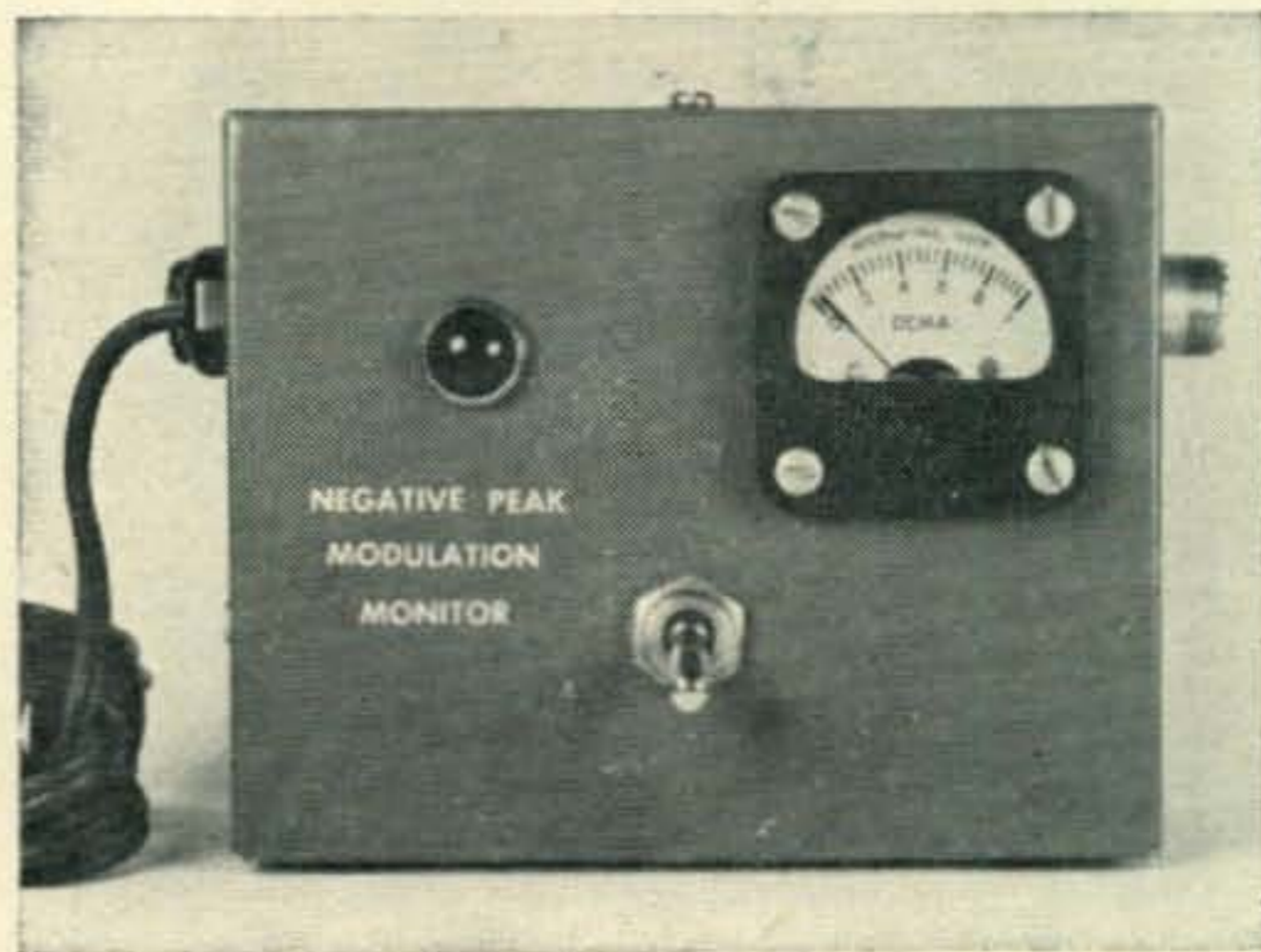
Front view of the trim looking modulation monitor. The pilot light serves as a ballast for the 1B3 filament as well as an indicator.
