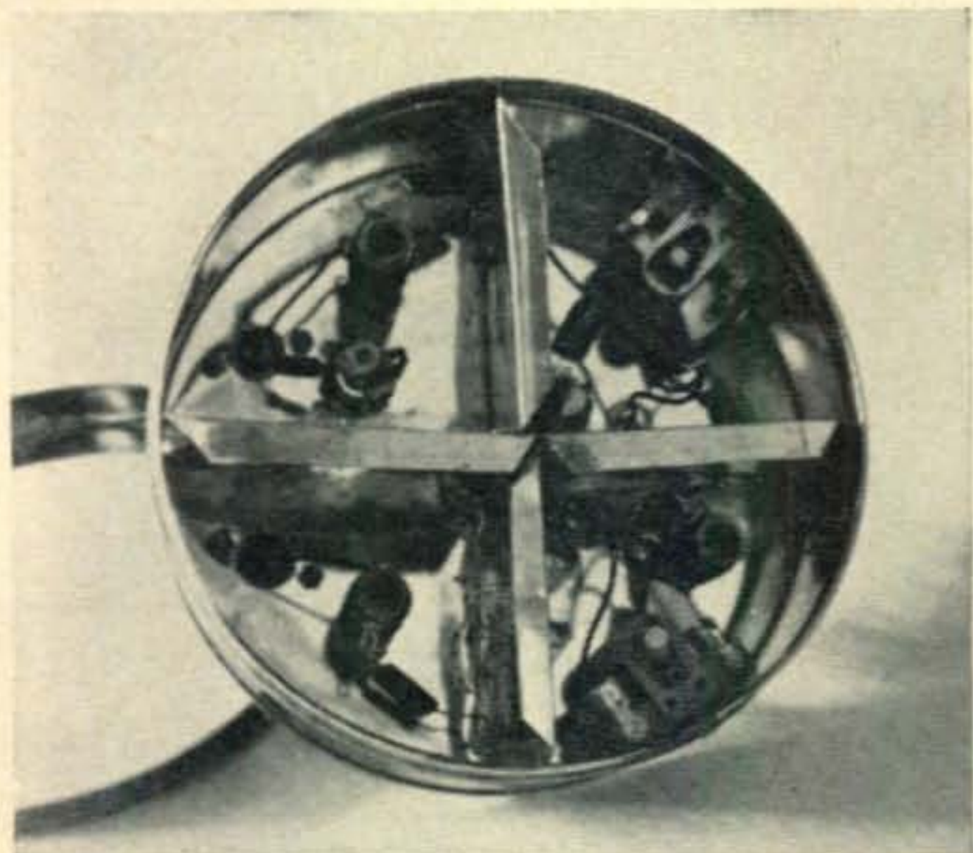
Underside view of the filter with cover removed. The signal enters at the lower left and travels around counter-clockwise, leaving the upper left hand compartment. Notice that the shielding is bent over at the top to provide a spring contact with the cover.
