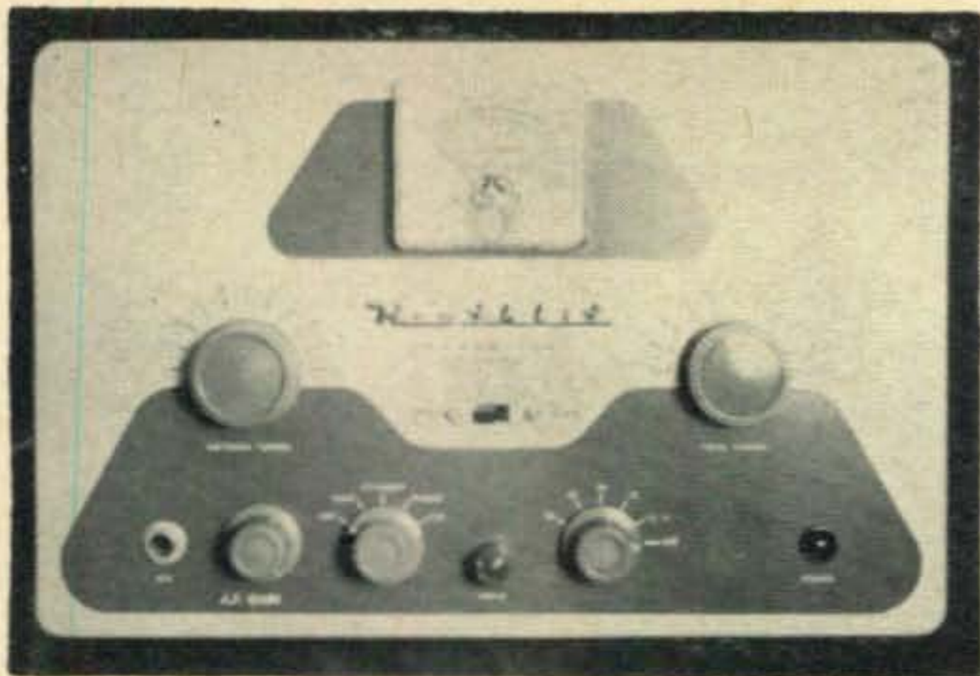
Front view of the DX-40 showing the location of the new audio gain control and the new 6 meter switch position.
