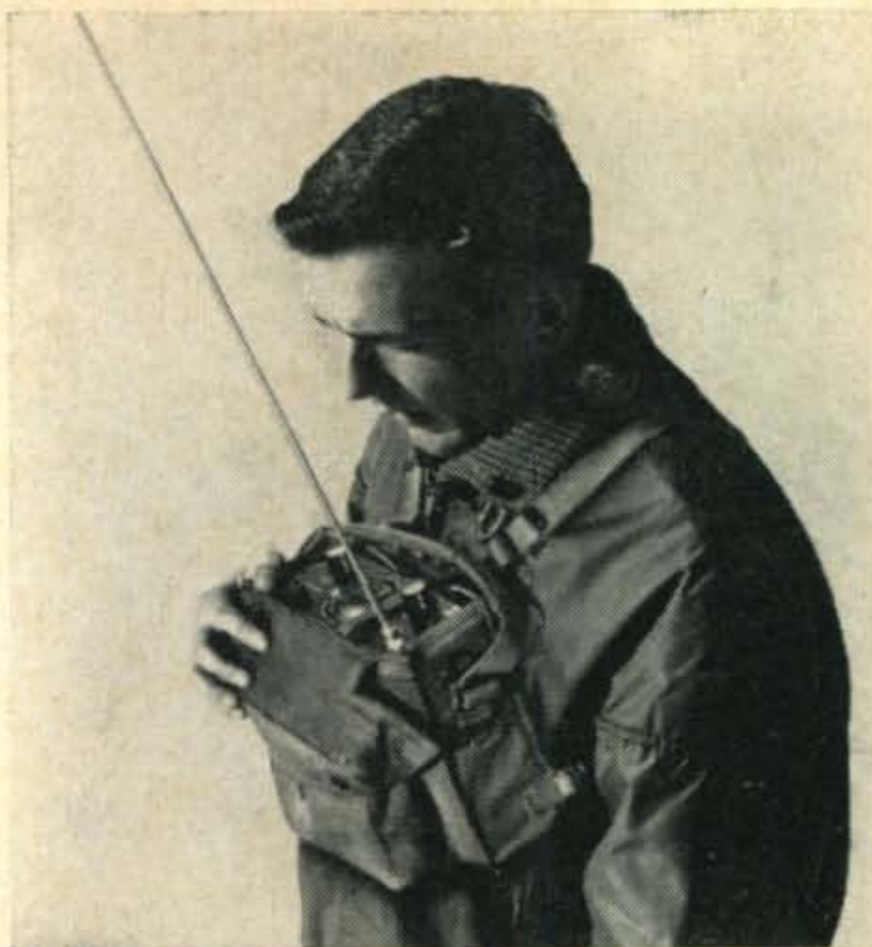
An English walkie-talkie manufactured by A. C. Cossor Co., Ltd. and used by firefighters in the London Fire Brigade. The unit, which weighs only five pounds, features a vox circuit. It operates in the low v.h.f. bands.
