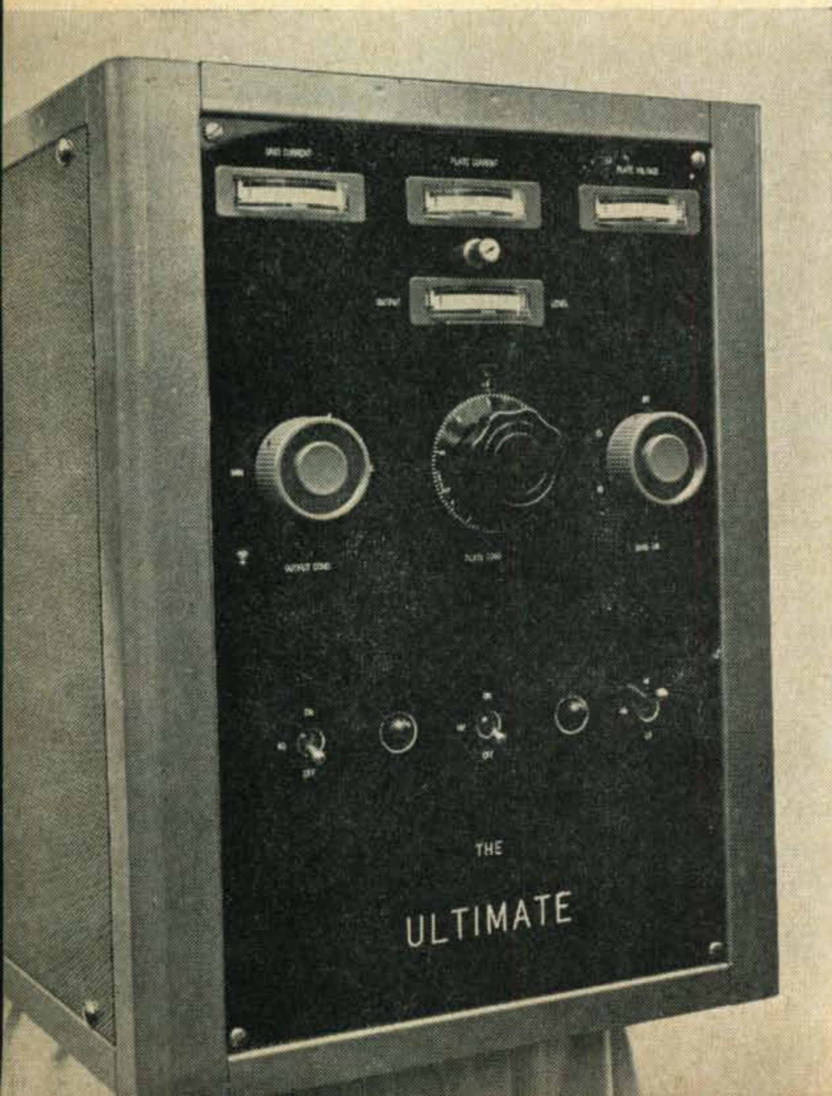
Front view of the "Ultimate" linear. The complete transmitter, including the power supply, is housed in a 16 \times 16 \times 20 " cabinet.
