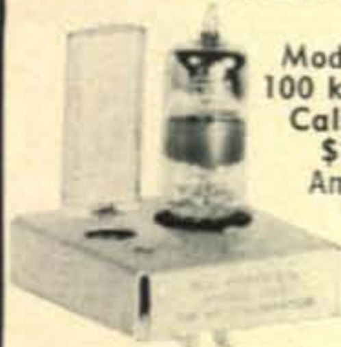
Model 2BQ Combination Q-Multiplier and Deluxe Speaker for notching heterodynes or single signal CW. $39.95 AMATEUR NET
