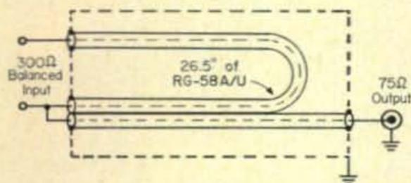
Fig. 2—A simple and compact 300 ohm to 75 ohm balun for two meters. The 26½" length of RG-58/AU may be coiled up to fit inside a minibox. Cables should be grounded to the minibox at both ends.
