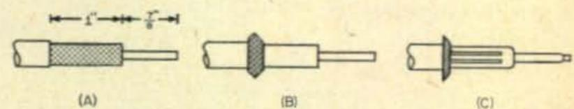
Fig. 1—Simple diagram showing how to solder coaxial cable into a Motorola type fitting. Strip covering back about 1 7/8" (A). Then push back the braid into a bead (B). Insert the plug until the bead touches the plug shell and solder the braid to the plug tabs. Solder the center conductor and cut-off any excess wire (C).
