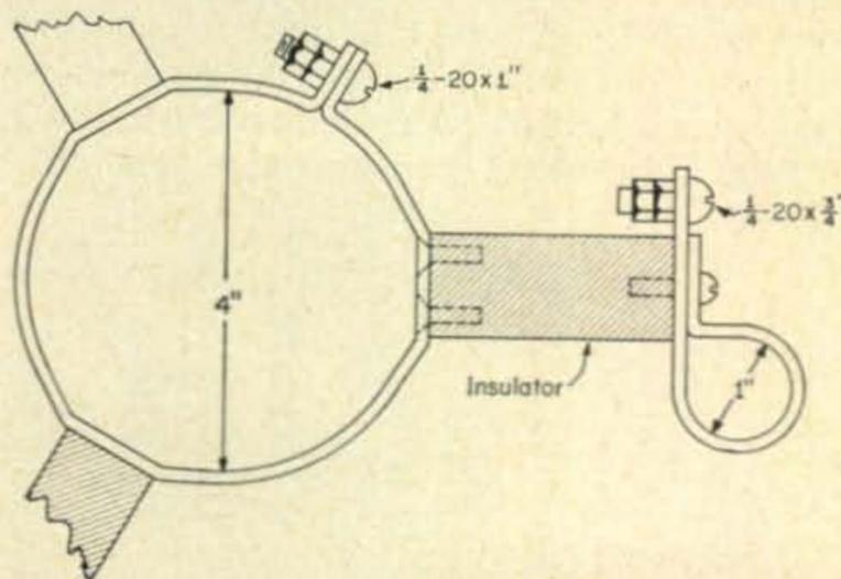
Fig. 10—Base mounting ring for the 3 feed lines. It is constructed from ⅛ × ¾" aluminum strap. The area beneath the 1⅛" × 1⅛" × 2½" insulators are flat for solid support. The tubing clamps (3) are also fabricated from ⅛ × ¾" stock. The hardware is brass of the dimensions shown.
