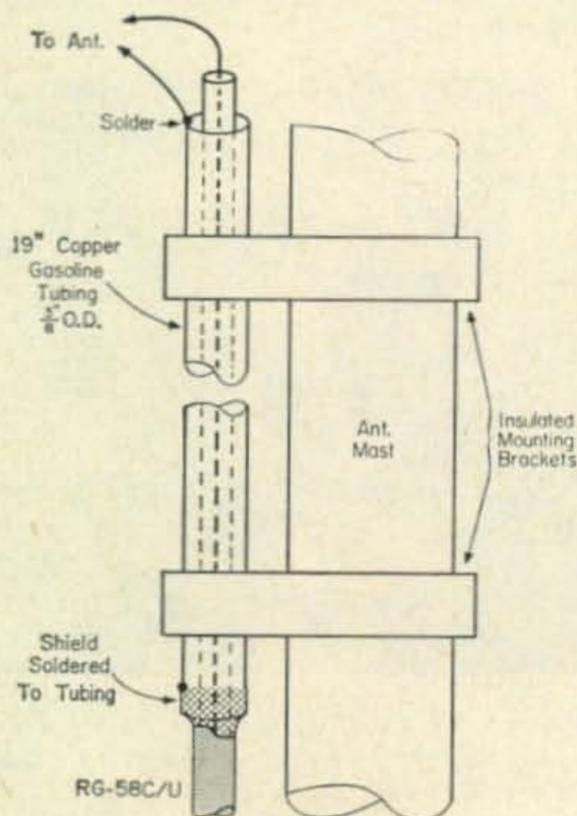
Fig. 2—Construction of the feeding section, showing mounting brackets in place.
