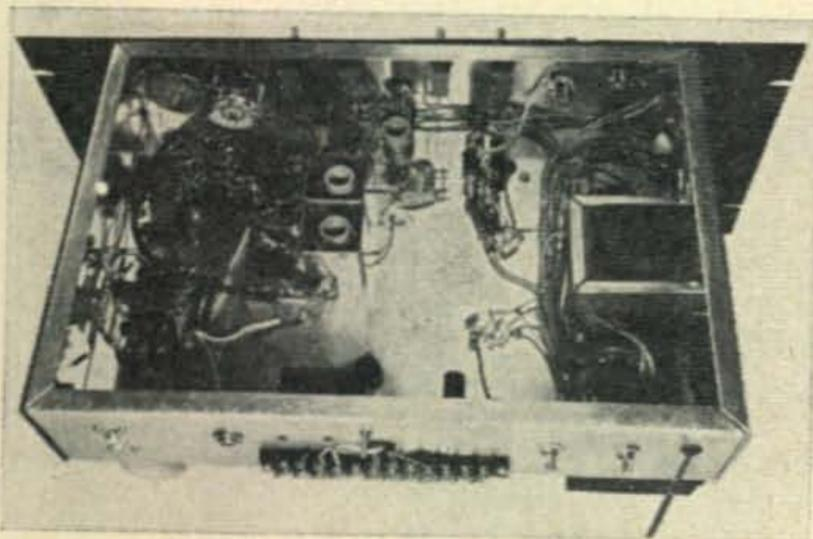
Bottom view of the ten meter receiver showing component layout. The r.f. and mixer coils are housed in the shields that came with the BC-455 while the h.f. osc. coil remains unshielded.
