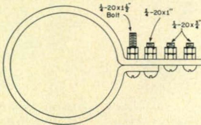
Fig. 11—Ground clamp details used to connect to the radials and the tuning unit. It is made from ¼ × 1" aluminum stock and furnished with brass hardware.
