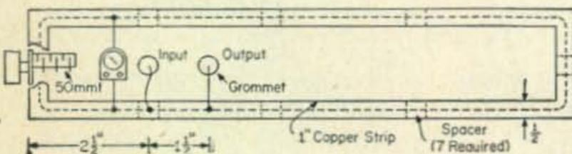
Fig. 1—Bottom view of resonator showing placement of essential components.
