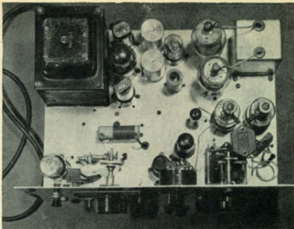
transformer, plate and screen modulates the final fully. The power supply consists of a full-wave bridge employing an RCA 630 type TV set power transformer. The two 6DE4's are the only new components (aside from the enclosure) in the entire transmitter.
