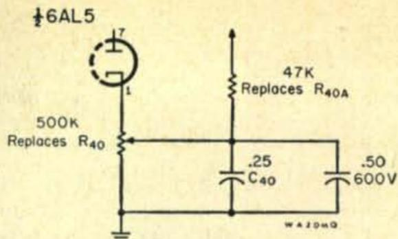
Figure 2—Modified vox circuit in the 20A to lengthen the delay time. See text.
