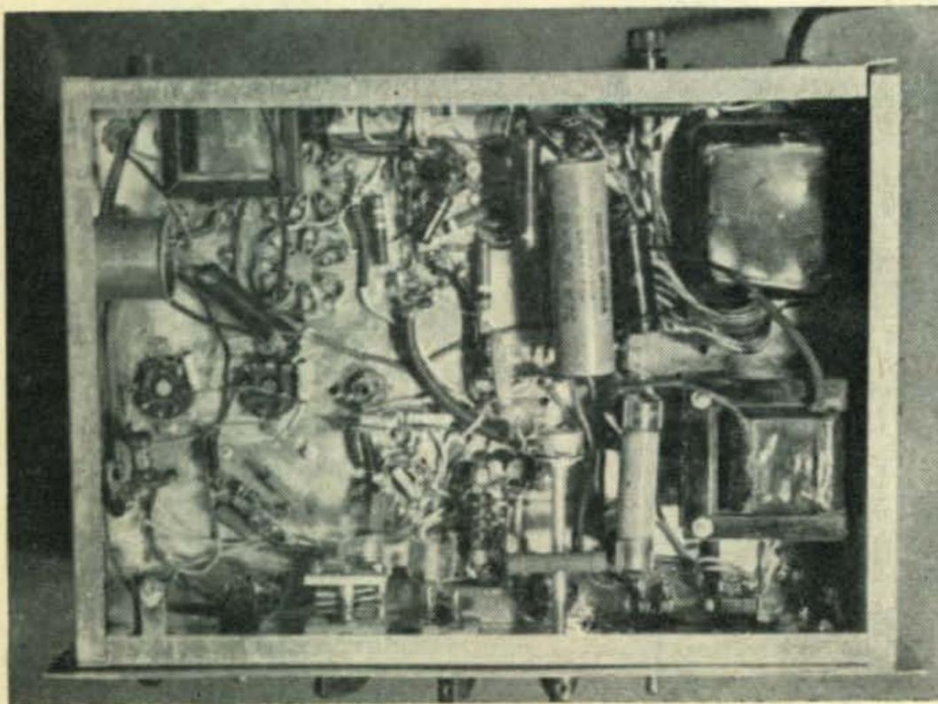
**Bottom view of chassis. R.f. section is to the left, modulator section in the upper center, and power supply on the far right. The larger transformer (upper right hand corner) is the main power transformer, while the smaller one in the upper left corner is modulation.**
