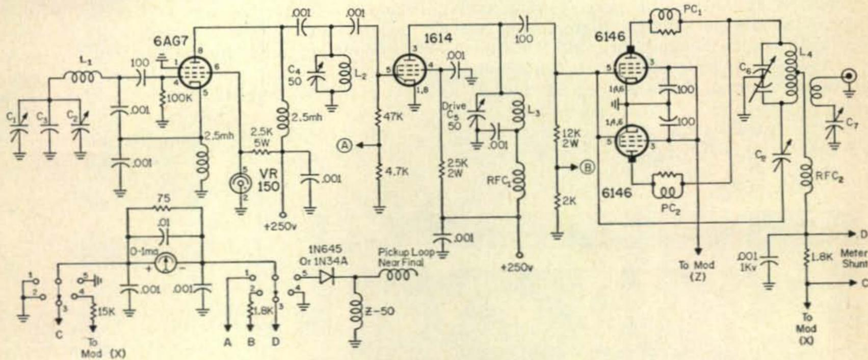
Fig. 1.—R.f. section of WA2NDM's medium power 50 mc v.f.o. controlled transmitter.
