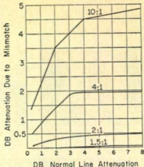
Figure 2—Line attenuation due to v.s.w.r.
