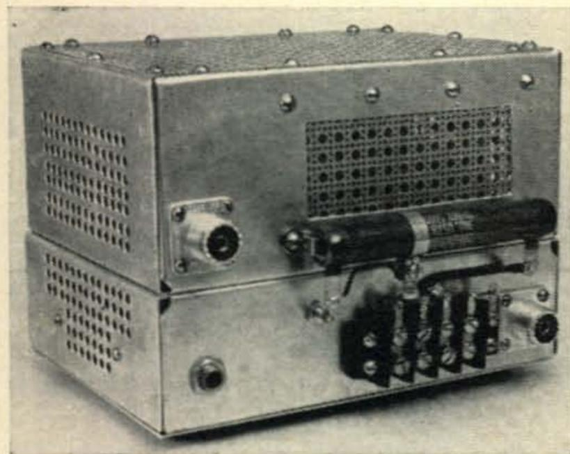
Rear view illustrates steps taken to provide ventilation. The large resistor is the main dropping resistor,  $R_{10}$ . Visible below it are the feedthrough bypass capacitors which filter the power leads. The output jack is at the upper left, the key jack just below it, and the v.f.o. input at the lower right.
