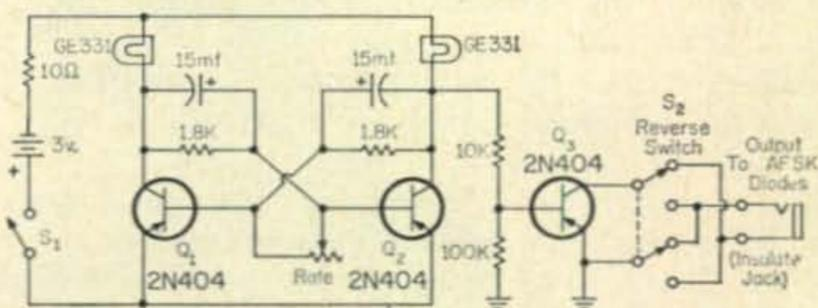
Fig. 1—Schematic diagram, W2JAV Dot Generator.
