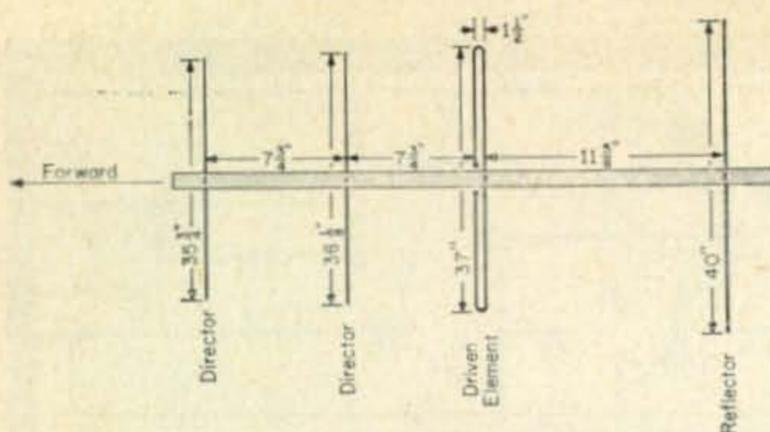
Fig. 1—Two meter four element close quarters antenna. All elements except the driven element are  $\frac{3}{8}$ " tubing. The driven element is constructed of  $\frac{1}{4}$ " o.d. copper tubing. Boom length is only 2'  $3\frac{3}{8}$ ".
