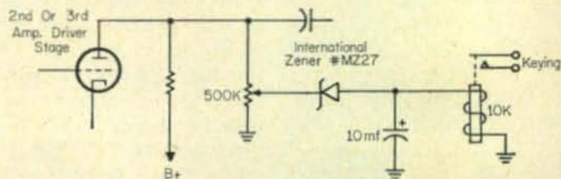
Fig. 3—One method for using tape recorded signals to drive a keying relay.
