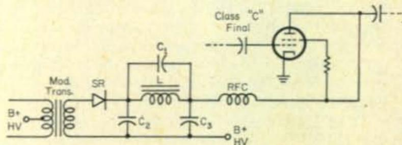
Fig. 2—High level speech clipper. See text for values.
