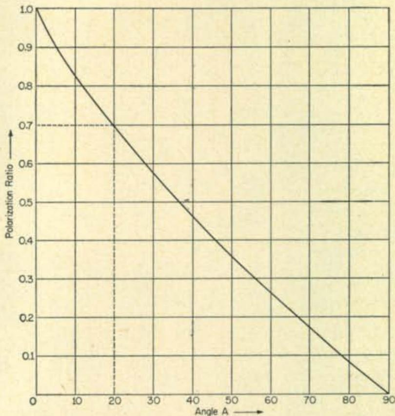
Fig. 3—The vertical axis is the ratio of the field strength in the shadow region for a horizontally polarized incident plane-wave to that of a vertically polarized wave.
