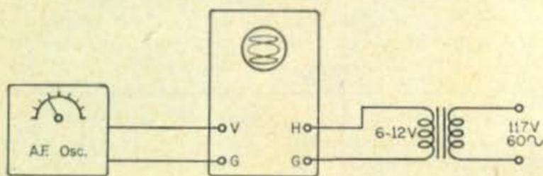
Fig. 1—System for calibrating an a.f. oscillator using a scope and employing Lissajous figures.
