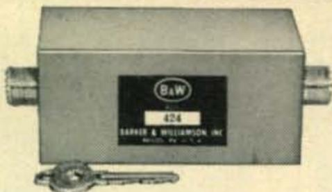
A B&W low pass filter will end interference with your neighbors TV reception. B&W Model 424 is a three-section low pass filter which installs in the antenna coaxial line. Reduces all frequencies within the TV band by 60 db (a reduction of 1-million times).
