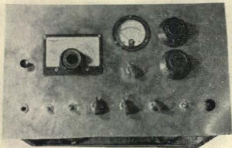
Front panel view of 50 mc transmitter. Left to right: mike jack, power switch, transmit/receive, audio gain, excitation, drive, tune/operate, pilot light. Top controls: spot button, meter, plate and coupling.
