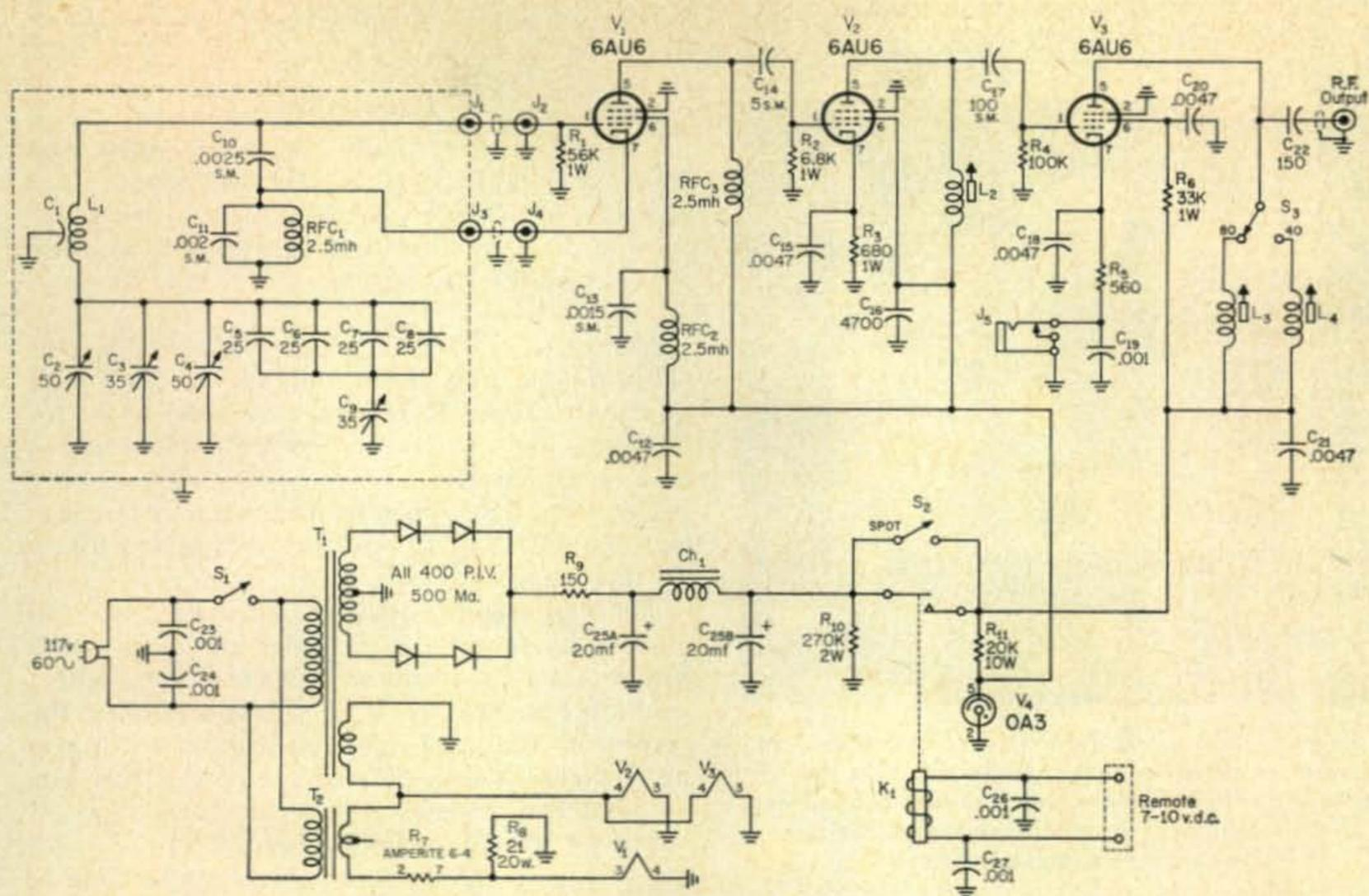
Fig. 2—Circuit diagram of the "Silver Sentry" an ultra-stable variable frequency oscillator with r.f. output on 80 and 40. All decimal value capacitors are disc-ceramic unless otherwise noted.
