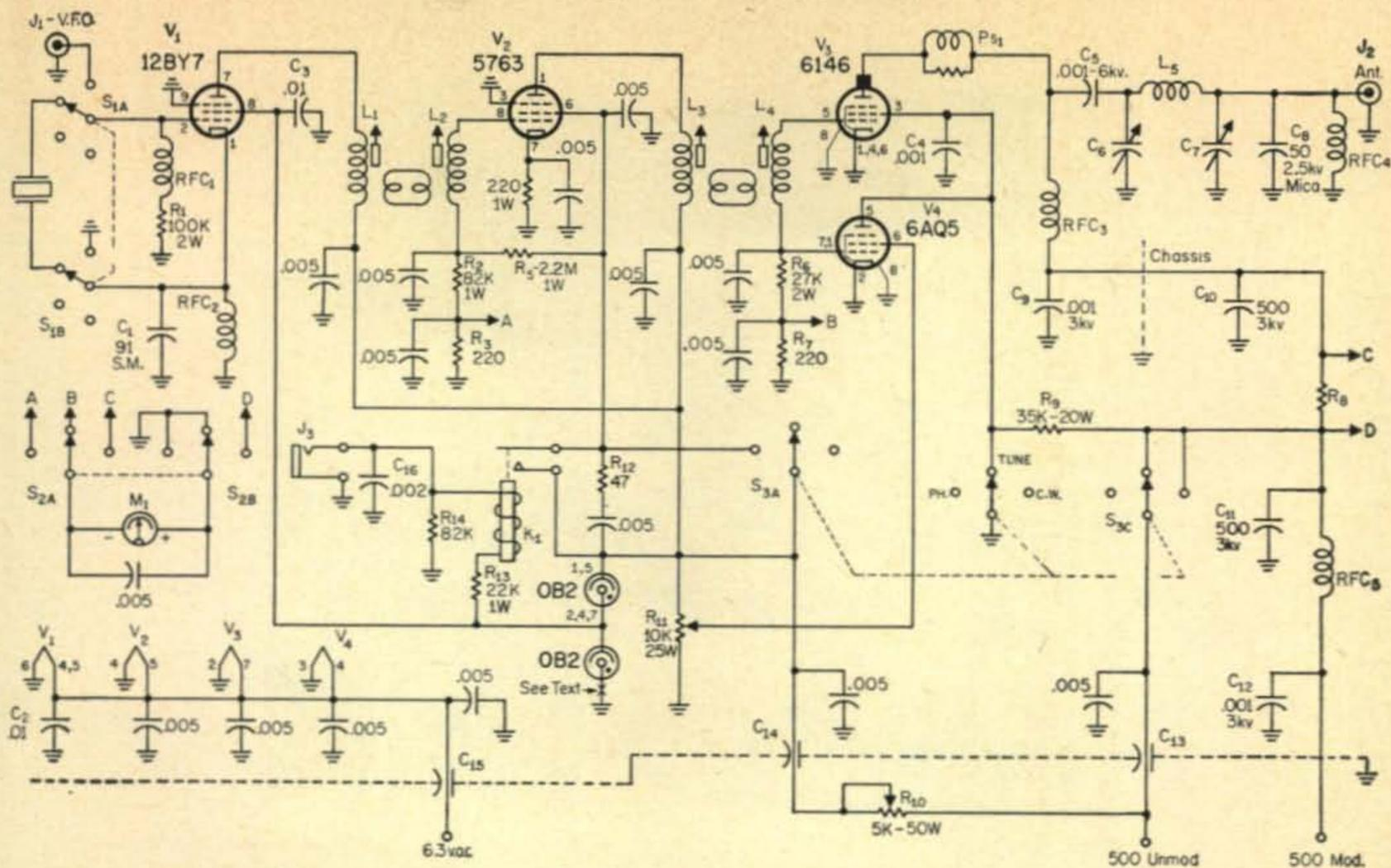
Fig. 1—Circuit of the broadbanded six meter transmitter. All resistors are  $\frac{1}{2}$  watt and all capacitors greater than 1 are in mmf unless otherwise noted. All capacitors are disc ceramic unless otherwise indicated.
