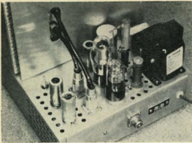
The "electronics," mounted on a 10" × 14" × 3" steel chassis, is coupled, via two lengths of coax to the inner compartment. The oscillator and doubler are placed at the left and the output 6AU6 is behind the voltage regulator. Connector  $J_4$  sits between  $V_1$  and the Amperite filament regulator tube. The aluminum heat shield is 7" × 9½".
