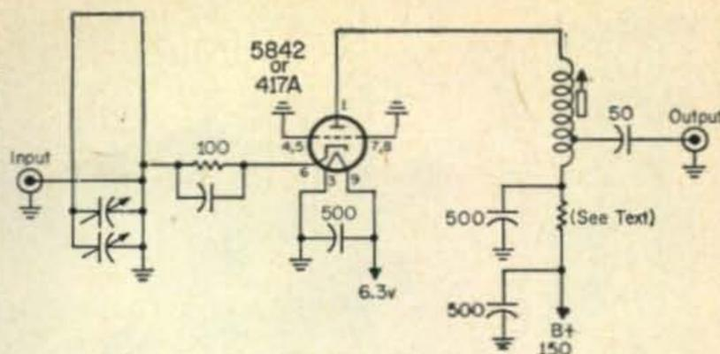
Fig. 2 Schematic diagram of the resonator and pre-amplifier.
