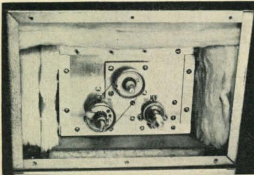
Two layers of insulation isolate the inner box from the outer shield. The shaft at the left tunes the variable capacitor, which is coupled, via a pulley arrangement, to the dial pointer. Notice that the dial pulley is mounted outside the chassis, insuring proper mechanical stability.
