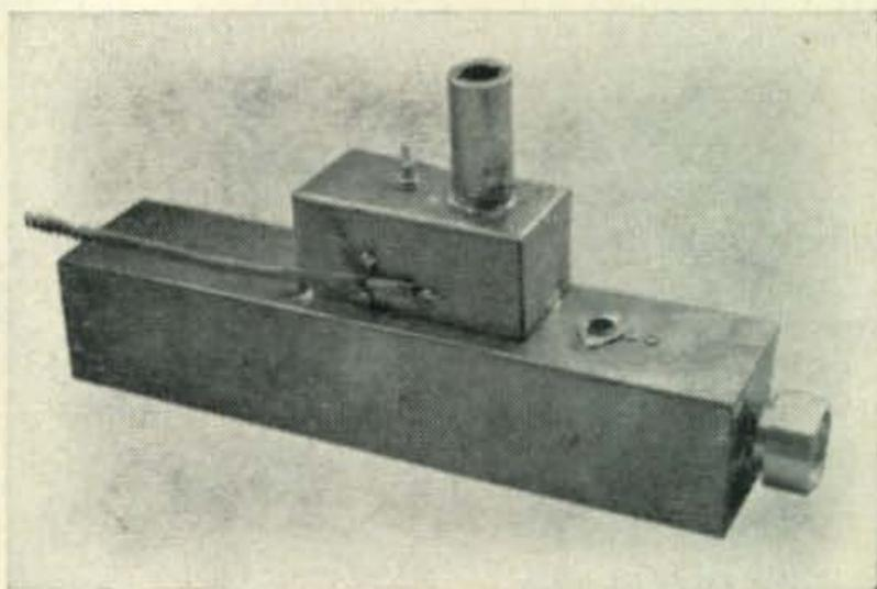
View of K3HNP's compact tunable cavity preamplifier for 50 mc overload problems. Tube used here is a 417A, but a 6CW4 or 6DS4 nuvistor can also be used with the same results.
