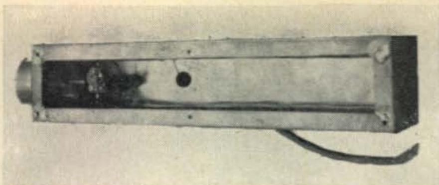
Underside view of the resonator. Lines run parallel with chassis edge along the entire length of the box (barely visible here). Dark section at the far left contains the variable capacitor and trimmer.
