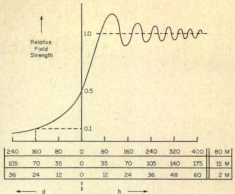
Fig. 2—Field strength at a depth  $d$  below and a height  $h$  above the hill-top relative to the incident plane wave is shown for the 80, 15, and 2 meter bands. The receiving antenna is 160 meters behind the hill ( $b=160$ ). Depth  $d$  and height  $h$  are in meters.
