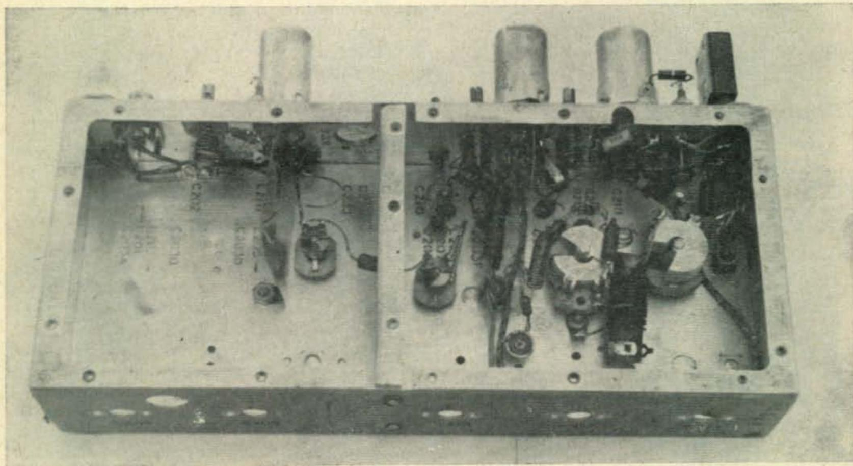
Inside view of the 432 mc transmitter. The chassis is surplus. Oscillator stage is at the right and final to the left. The shield partition separates the two 432 mc tuned circuits,  $L_7$  and  $L_8$ .
