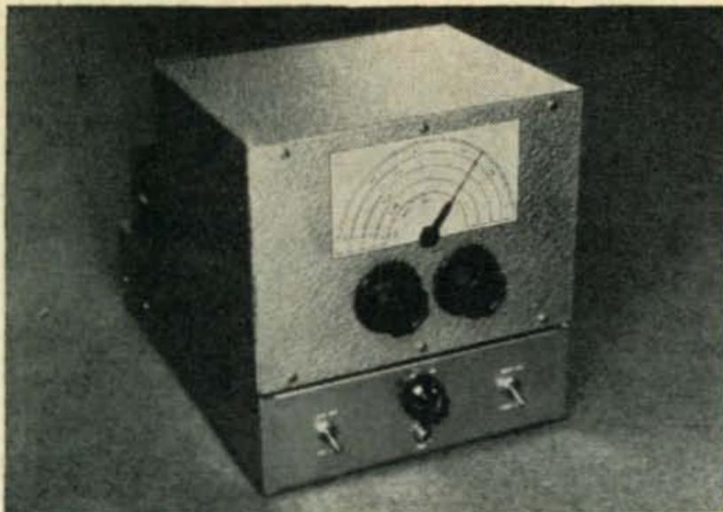
The "Silver Sentry" a high stability v.f.o. derives its name from the fact that the 10" X 8" X 7" utility box housing the inner chassis, which is insulated with fiberglass wool, is sprayed with silver paint for heat reflection purposes. The large controls are v.f.o. tuning and FINE tuning. The key jack is just below the band-switch and the SPOT switch is on the right.
