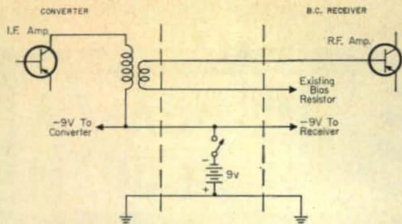
Fig. 1—Method of connecting a transistorized v.h.f. converter to a slightly modified 8-transistor BC radio. The existing BC-set antenna coil should be removed and its variable capacitor used to tune the converters' output coil.
