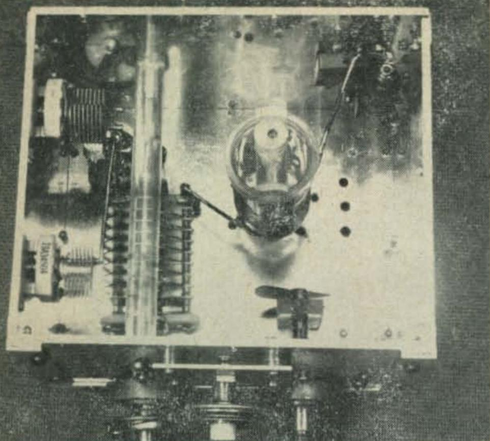
The heart of the v.f.o. is the tank circuit packaged into a home-brew  $\frac{1}{8}$ " aluminum box. The  $\frac{1}{2}$ " poly rod running front to back was needed to reduce cabinet flexing. The single plate, variable capacitor at the right is the very fine tuning control.
