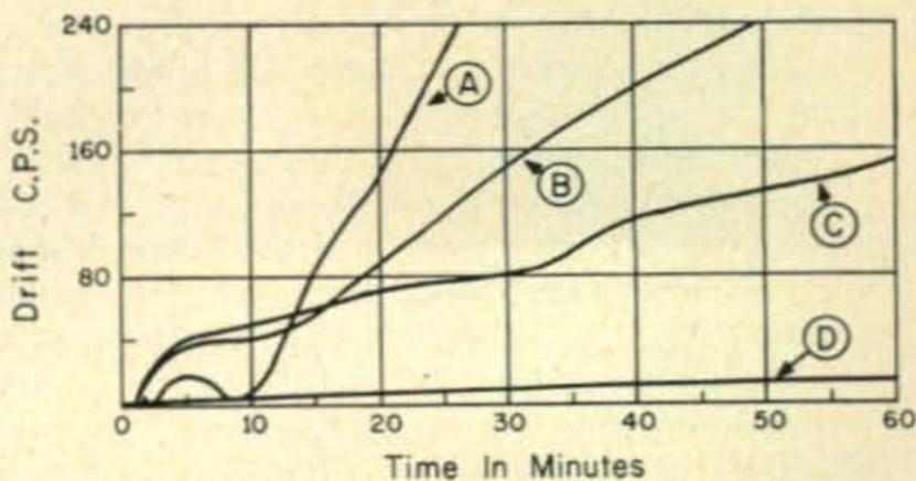
Fig. 1—Typical curves plotted by the author on: A—a medium priced commercially available s.s.b. transmitter; B—a high quality a.m. transmitter, circa 1952; C—top quality s.s.b. transmitter and D—The "Silver Sentry."
