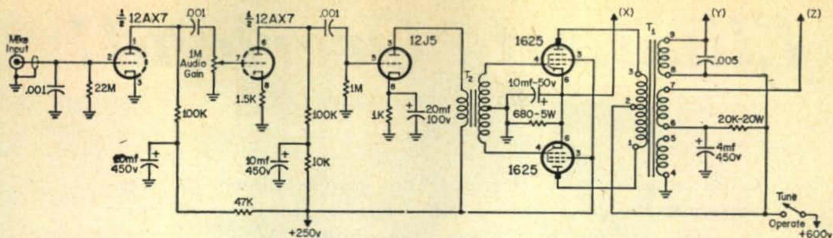
Fig. 2—Schematic diagram of the modulator and speech amplifier using 1625's.
