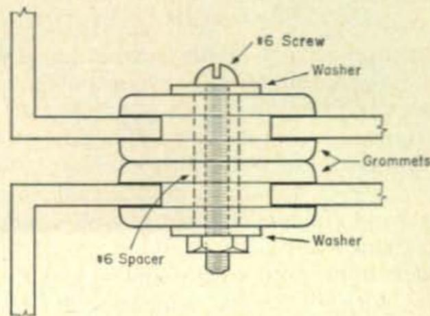
Fig. 3—Details of the shock mounting between chassis. This method also reduces heat conduction between units. Grommets are General Cement #HO 43-F.
