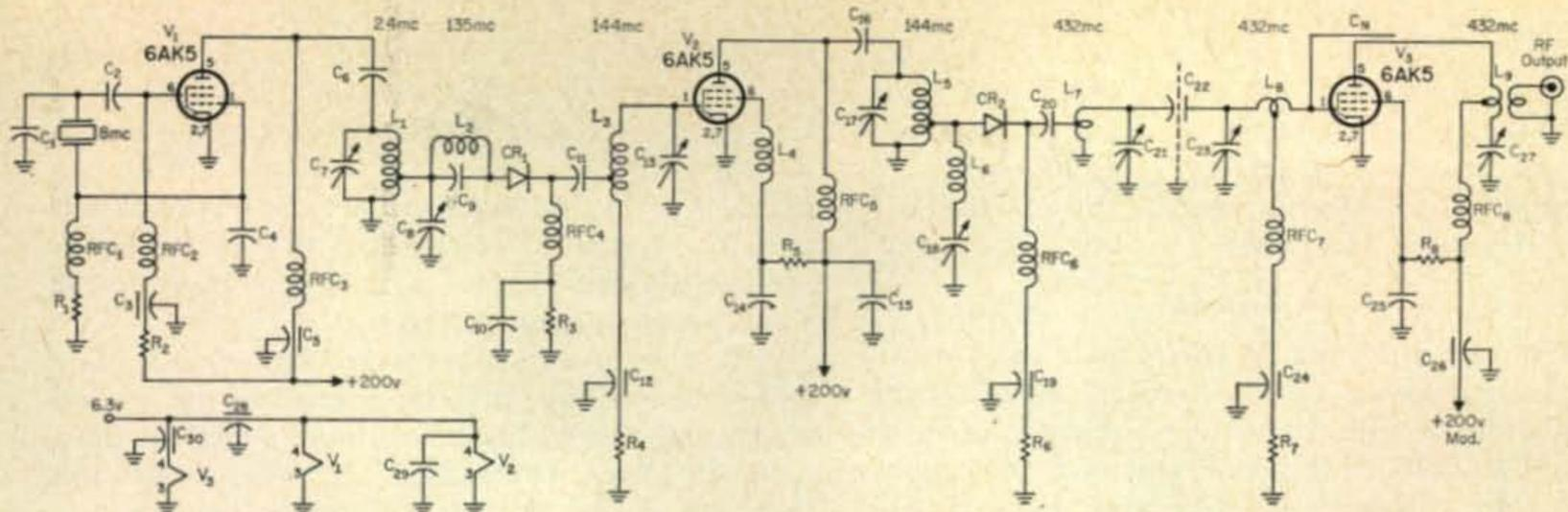
Fig. 1—Circuit of the 3 tube 432 mc exciter-transmitter capable of a quarter watt output. All resistors are  $\frac{1}{2}$  watt. Resistors  $R_4$ - $R_6$  and  $R_7$  are mounted external to the shielding for convenience in testing.
