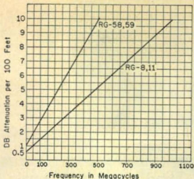
Figure 1—Normal attenuation of coax feedline as referenced to frequency. The difference between RG-58 and RG-59 is so small that they have been shown as a single line, as with RG-8 and 11.
