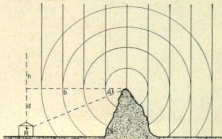
Fig. 1—The receiving station,  $R$ , is shown at a depth  $d$  below, and a distance  $b$  behind the hill-top. The straight vertical lines indicate a plane wave advancing from right to left. The circles indicate a diffracted cylindrical wave originating at the top of the hill. See Text.
