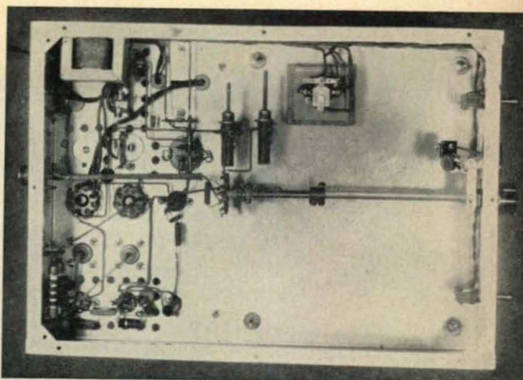
This view illustrates the mounting of the output inductors  $L_3$  and  $L_4$ . Notice the ventilating holes around the heat producing components at the left.
