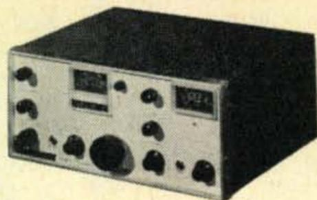
Complete SSB, AM, and CW coverage of the 80, 40, 20 meter amateur bands . . . many outstanding features for easy relaxed ham operation ■ Full 200 watts PEP input ■ Handsome, rugged NCX-3 complements both your car and ham shack ■ VOX or push to talk ■ CW break-in, SSB/CW AGC, S-meter ■ Separate AM detector! ■ Available in December! Order now for early delivery ■
