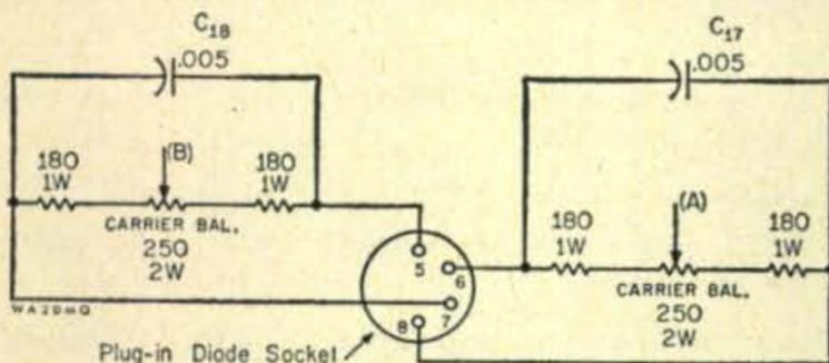
Figure 1—One method of obtaining a more s.s.b. with less a.m. on the 20A. See text.
