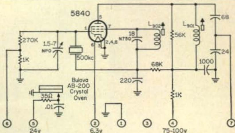
Fig. 1-Circuit of the calibrator for serial #2456 to #5602.
