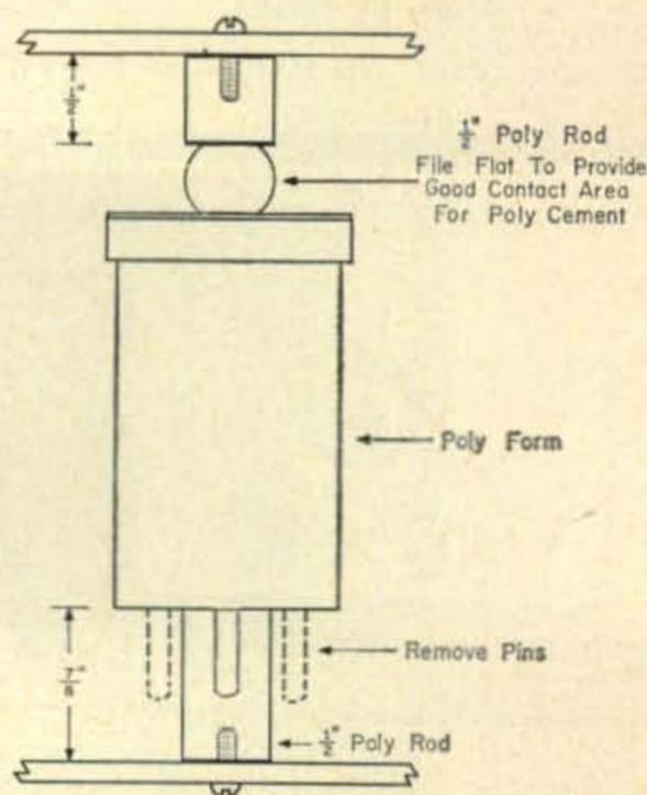
Fig. 4—Details of the construction of inductor  $L_1$ . Half-inch poly rods are used to "float" the coil between the top and bottom of the inner cabinet. See text.
