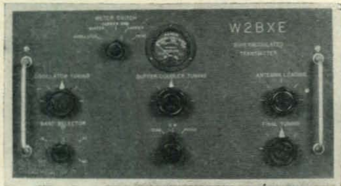
Front view of the Super-Pi transmitter employing Taylor supermodulation. The bottom row of controls, from l. to r. are, BAND SELECTOR, TUNE-OPERATE, FINAL TUNING. The next row is OSCILLATOR TUNING, BUFFER TUNING and ANTENNA LOADING. The METER switch is to the left of the meter.
