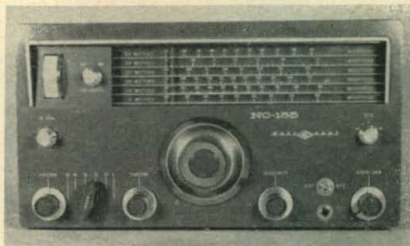
Front view of the NC-155. The controls are (bottom row) l. to r., ANTENNA, BANDSWITCH, FUNCTION, SELECTIVITY, STBY-REC. switch, AUDIO GAIN. Top row, l. to r., RF GAIN, MAIN TUNING, BFO. To the right of the S-meter, CALIBRATE Switch. Below the STANDBY-REC. switch is the phone jack.
