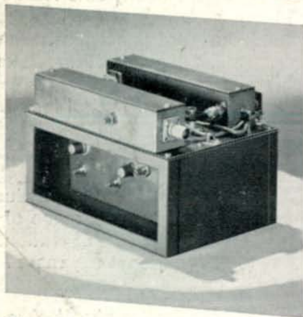
The Ham Tips 432-Mc Converter, using six RCA Nuvistors, including the RCA-8058 double-ended, high-mu triode which is used in 2 rf amplifier stages.
