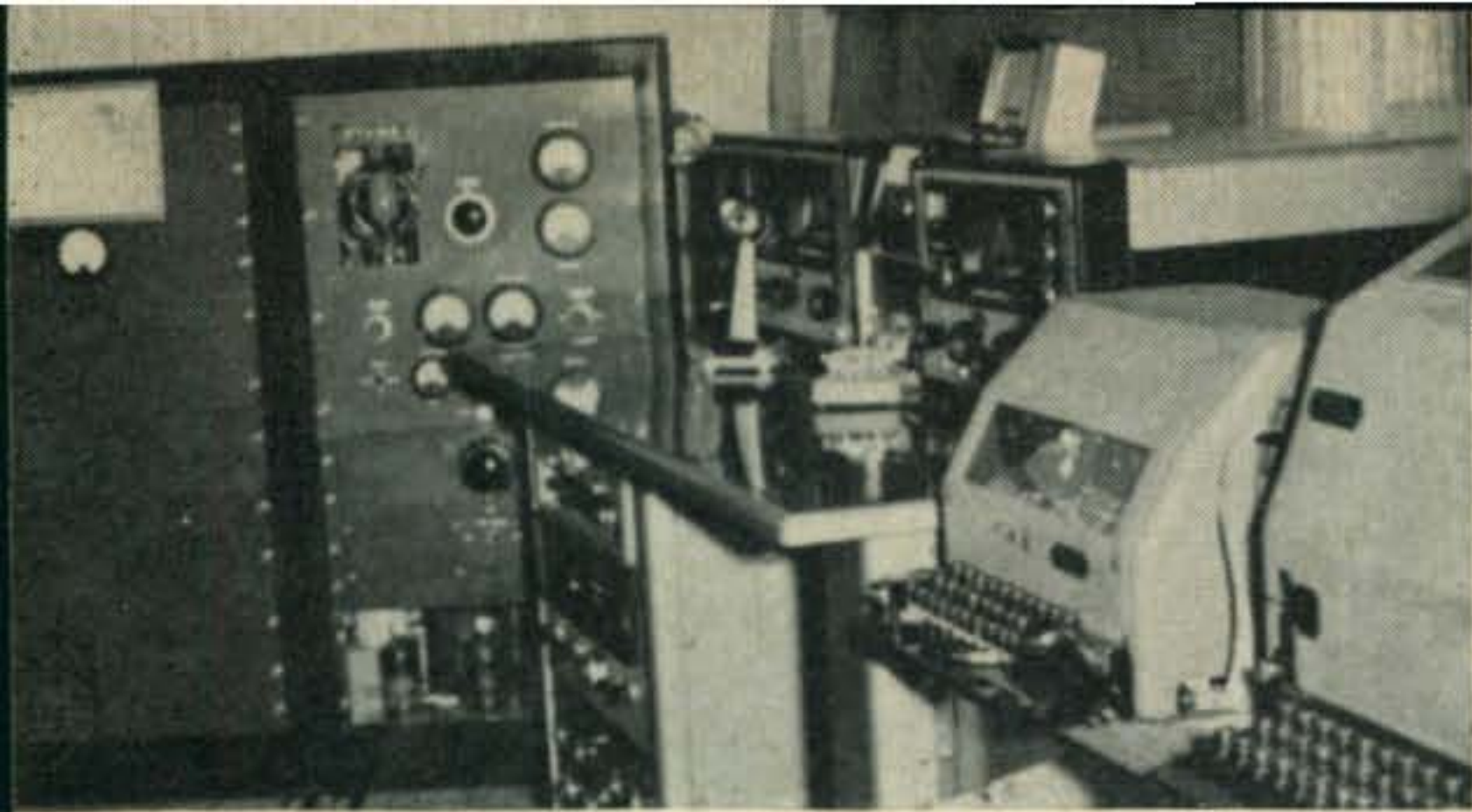
W7SMB/6 Trowbridge, California, RTTY station of E. M. Lenn. Exciter: HT-32B; Receiver: SX-115; Terminal Unit: CV-89 of AN/URA-8A; Final Amplifiers: HT-33A driving a pair of 1000-T's in grounded-grid; Antenna: 3 elements on 20, 2 elements on 40; 65 foot crank-up tower; Teletype: Model 15 and Model 14 Typing Reperforator and Model 14 TD.
