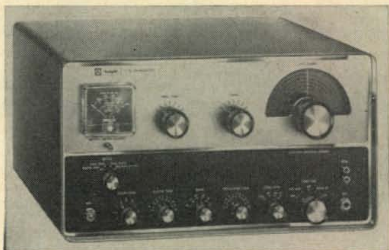
Front view of the Knight-Kit T-150 transmitter. Two 6146s are in the final, covering 80 through 6 meters.
