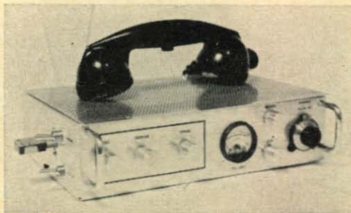
Completed unit after construction. Toggle switches on left are B+ and filaments. Front panel controls, left to right, oscillator, tripler, final loading, final grid meter, regen control, volume and tuning, 144-148 mc.
