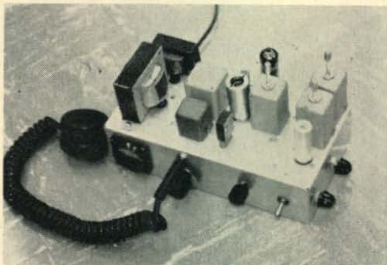
K6VLB's version of the Adapt-O-Citer described in the June '62 issue of CQ incorporating the VHF Quacker from the Sept. '62 VHF COLUMN. The balanced modulators are at the right front with the r.f. transformers in the shield cans.
