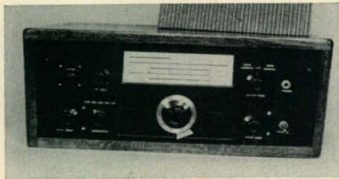
Front view of W6MTY's impressive receiver. The main tuning dial is a Millen 10035 with a Waldom 303 for vernier. The control functions are, lower row, left to right; A.V.C. DELAY, BANDSWITCH, AUDIO GAIN, STANDBY. The I.F. GAIN is above the BANDSWITCH and the CRYSTAL FILTER switch is above the AUDIO GAIN.
