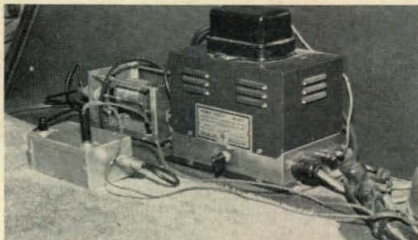
The trunk contains the Master Matcher rotary inductor and Elmac power supply. The coax phase detector is in the foreground.
