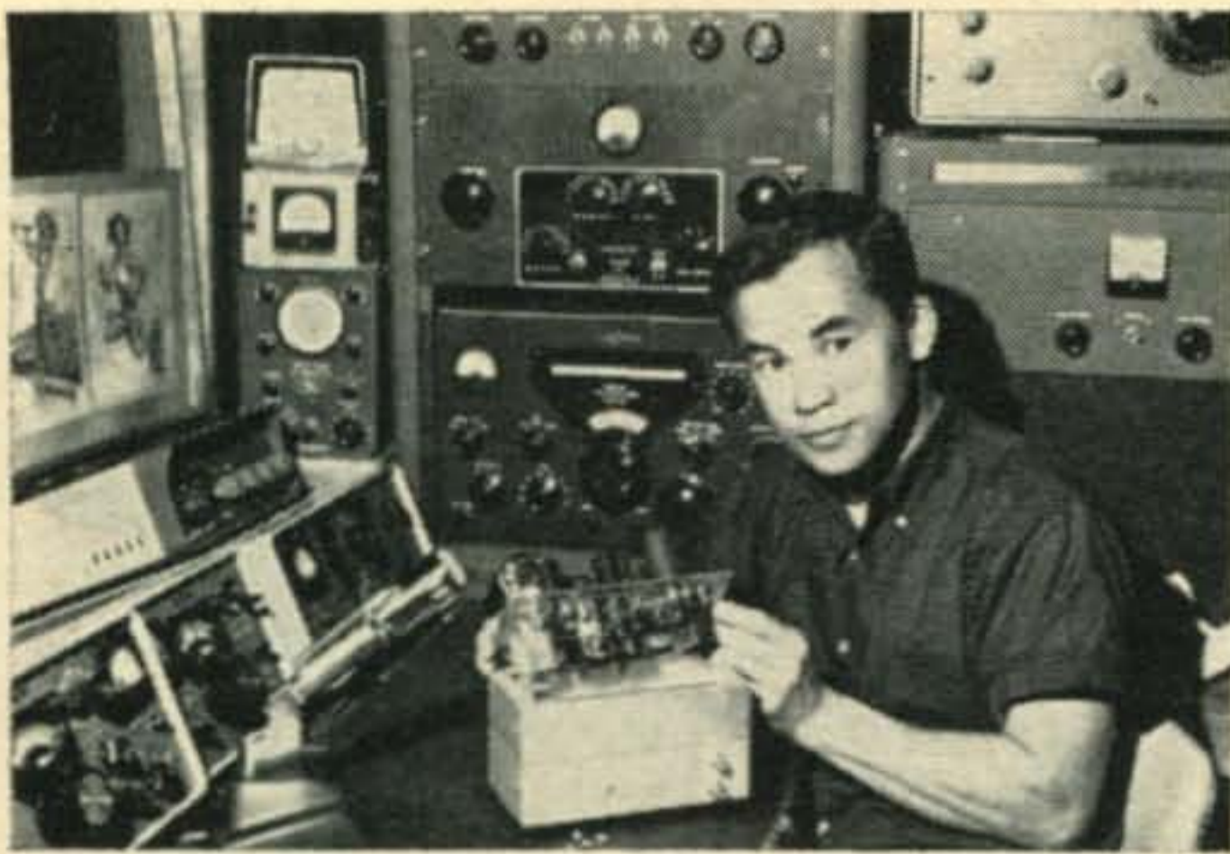
Step right up and meet George Chong, W6BUR, VHF enthusiast extraordinary, holding a homebrew 50 mc low level sideband mixer. Photo courtesy of Cal Cape.
