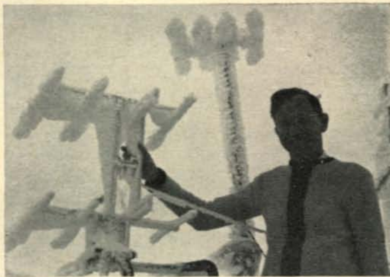
Ice-covered 432 mc antenna on top of Germany's highest mountain, Zugspitze. DL9JU controls antenna temperature . . . The Zugspitze is chosen as a contest location very often since it opens the VHF doors to the southeastern parts of Europe.
