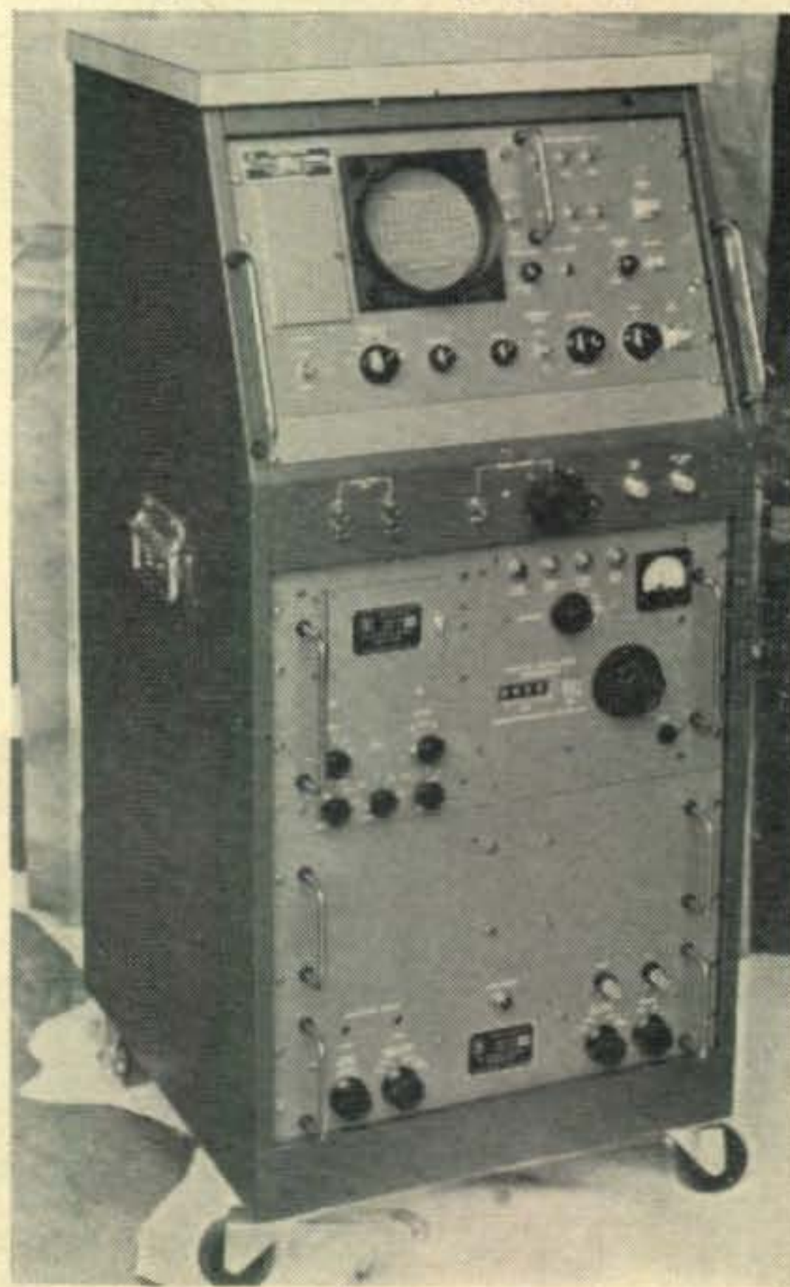
A modern spectrum analyzer which covers from 1.5 to 64 mc. At top is panadaptor display. At bottom are tone generators and power output jacks and manual sweep control. (Photo courtesy TMC, N. Y.)
