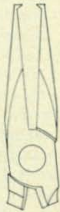
Nose-cutting pliers (left). A side-cutter is located slightly back from the tip of the nose. End-cutter with transverse cutting blades is shown at the right.
