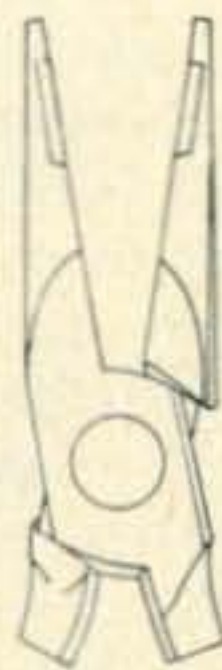
Nose-cutting pliers (left). A side-cutter is located slightly back from the tip of the nose. End-cutter with transverse cutting blades is shown at the right.
