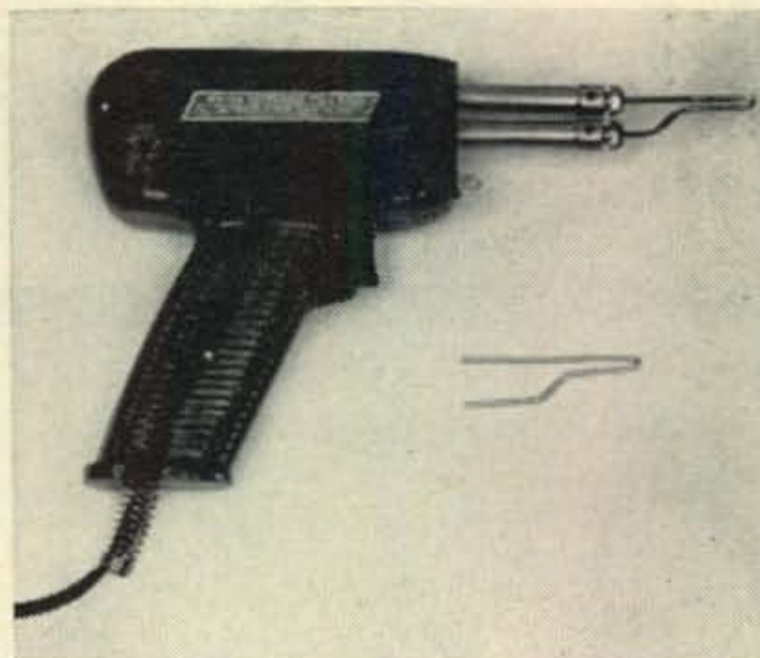
Soldering Gun. Weller Model 8200, 100-150 watt dual heat. Spare replaceable tip is shown below.
