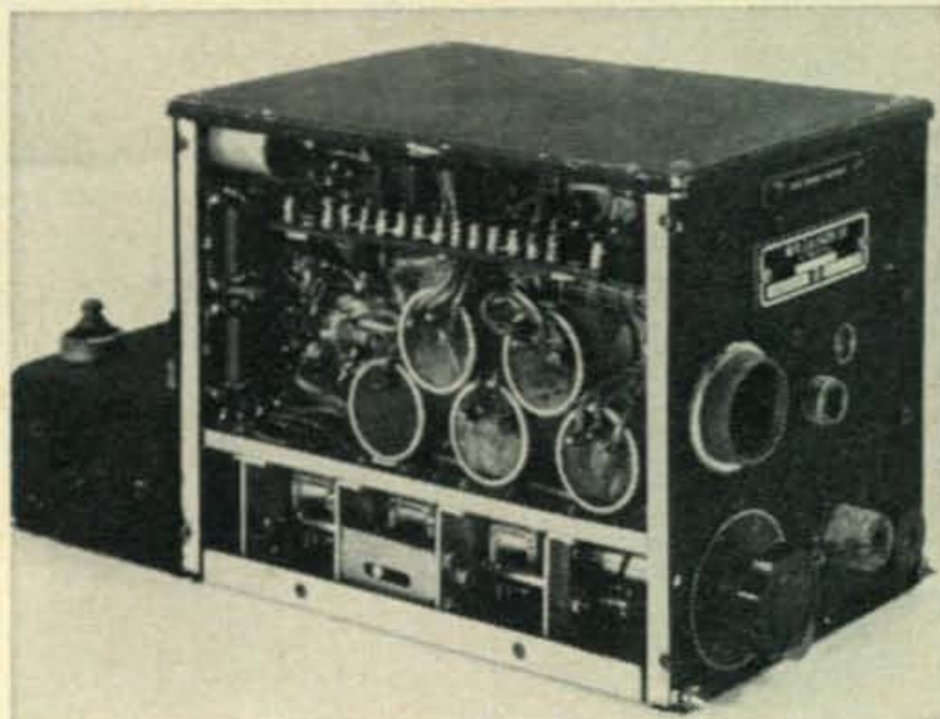
View of an unmodified ARR-2X. The tuning section is located at the lower left and is cut away from the main unit.
