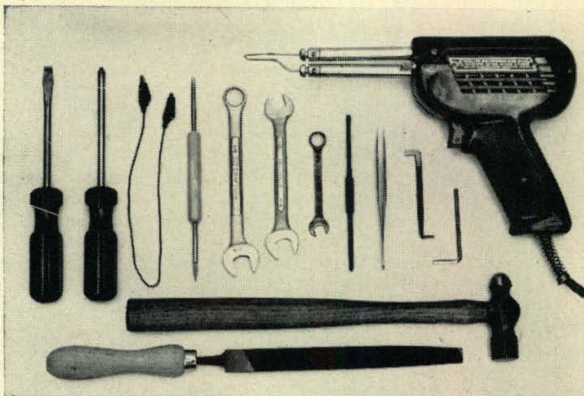
Fig. 5—Pictured left to right: 1/4" blade screwdriver, Phillips-head screwdriver, 12" clip lead with miniature clips, soldering aid, combination open end and box wrench, double open end wrench, ignition-type wrench, one type of alignment tool, tweezers, offset screwdriver and hex or Allen head wrench. Top right: soldering gun. Bottom: ball peen hammer and single-cut file.
